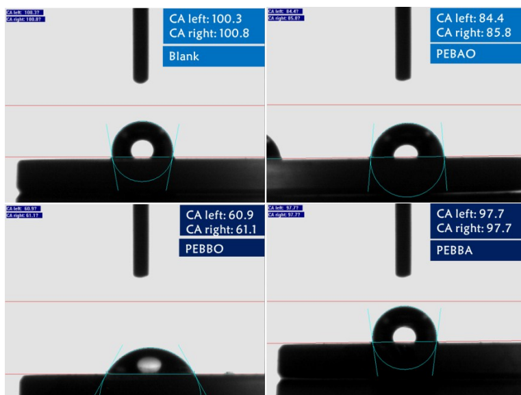
Fig. S13 The contact angle images of blank substrate and the LB films based on PEBBO, PEBAO or PEBBA.
