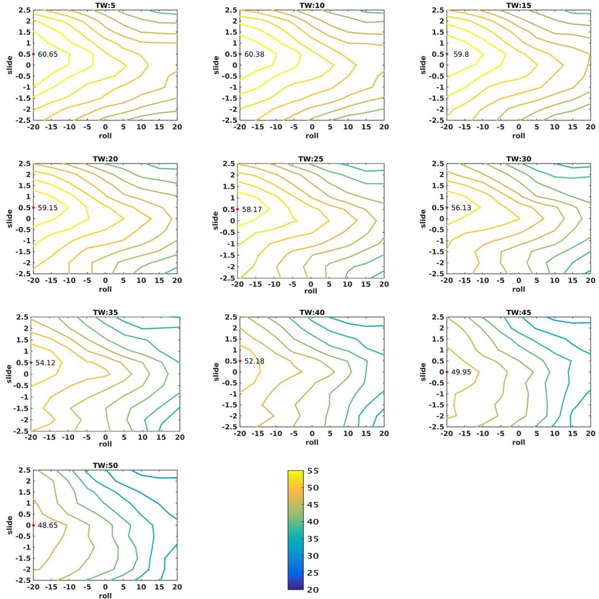
**Figure SI-2:** Stacking overlap area contours at different twist values for A:U W:WC::C:G:W:WC are shown here. Color bar is given in  $\text{\AA}^2$ . Contour lines are  $2.5 \text{\AA}^2$  apart.
