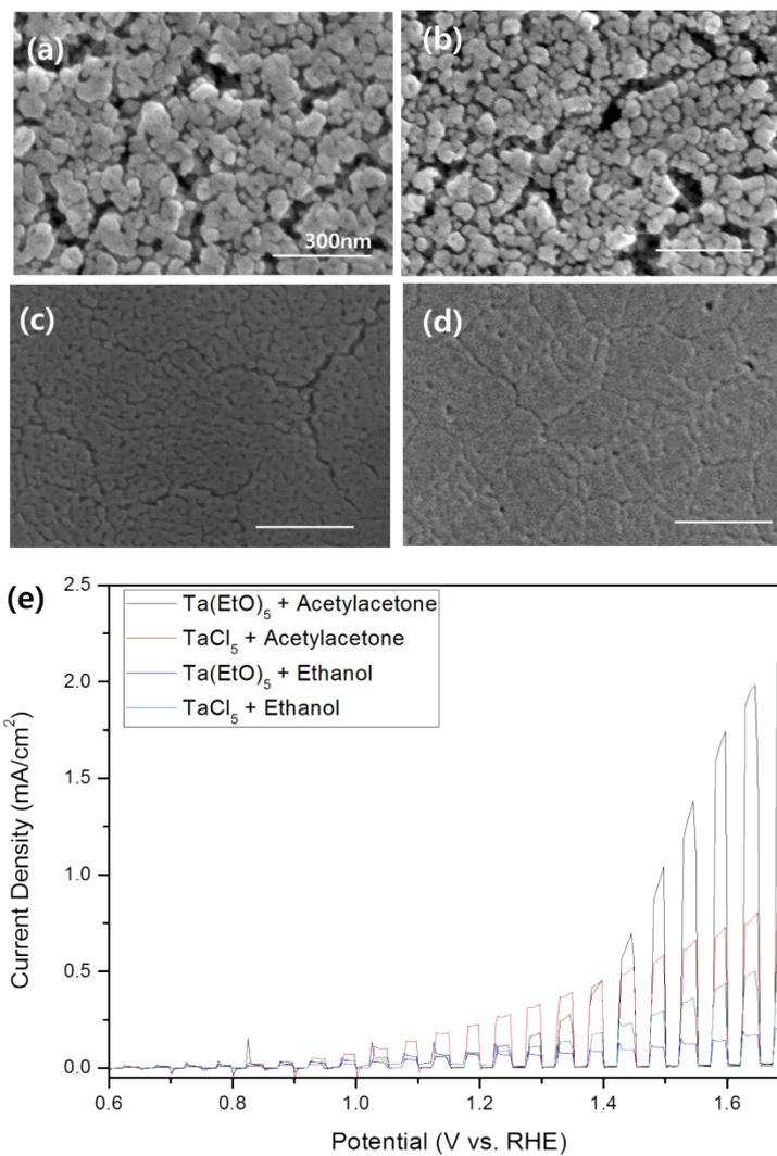
**Figure S4.** SEM images of Ta<sub>3</sub>N<sub>5</sub> thin film prepared from different precursor solutions: (a) Ta(EtO)<sub>5</sub> + Acetyl acetone, (b) TaCl<sub>5</sub> + Acetyl acetone, (c) Ta(EtO)<sub>5</sub> + Ethanol, and (d) TaCl<sub>5</sub> + Ethanol. (e) Effect of the precursor solution on the PEC activity of the Ta<sub>3</sub>N<sub>5</sub> photoanodes.
