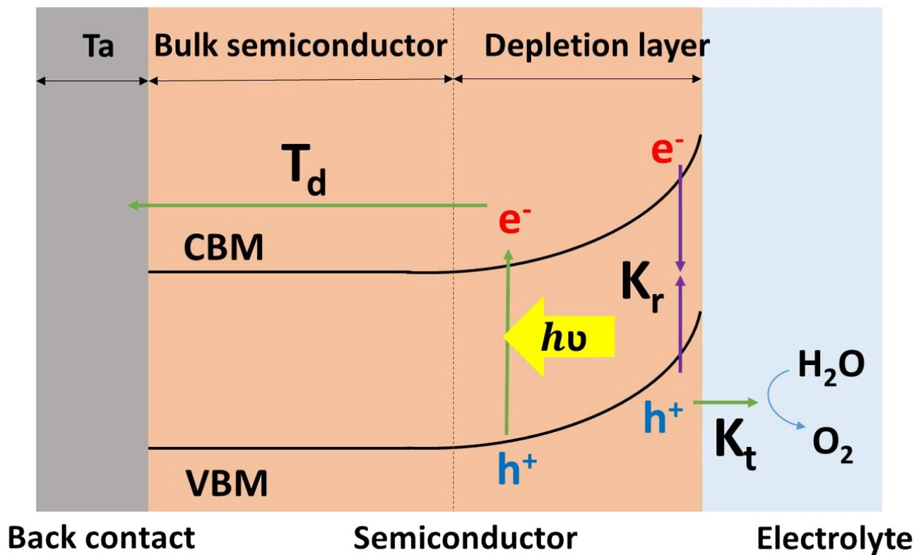
**Figure S5.** Schematic illustration of charge flow process and charge separation related parameters in a semiconductor photoanode.
