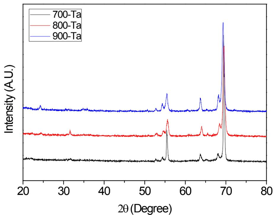
**Figure S3.** XRD patterns of 700-Ta, 800-Ta, and 900-Ta showing strong metallic Ta patterns. The absence of the  $\text{Ta}_3\text{N}_5$  patterns compared to 700-, 800-, and 900- $\text{Ta}_3\text{N}_5$  samples indicates the crystalline  $\text{Ta}_3\text{N}_5$  thin film is formed by using Ta source from the precursor solution through the preparation processes in this work.
