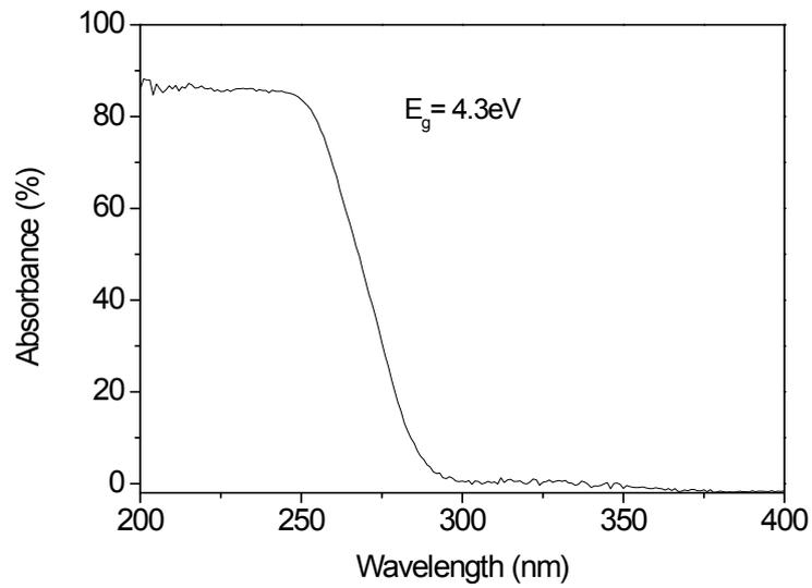
**Figure S1.** UV-vis spectroscopy of the deposited film on a quartz plate before the ammonia treatment. The tantalum precursor solution was spin coated on the quartz substrate, and it was annealed at 400°C in air for 1 hour to prepare tantalum oxide as described in the experimental method. The measured UV-vis spectra shows only UV region absorption due to large bandgap of tantalum oxide.
