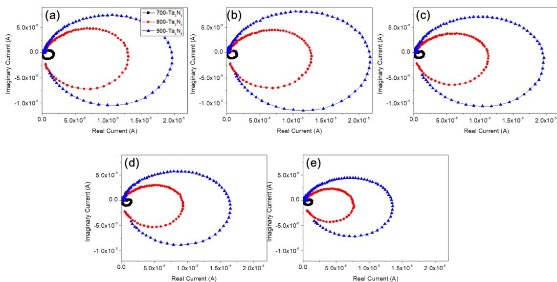
**Figure S6.** Nyquist plots of  $\text{Ta}_3\text{N}_5$  photoanodes depending on the nitridation temperatures at various applied potentials; (a) 1.05 V, (b) 1.25 V, (c) 1.45 V, (d) 1.65 V and (e) 1.85 V vs. RHE measured in 1 M KOH aqueous solution.
