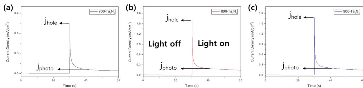
**Figure S7.** Current density versus elapsed time during IMPS measurement for each sample.  $j_{\text{hole}}$  and  $j_{\text{photo}}$  are marked in the I-t graph.
