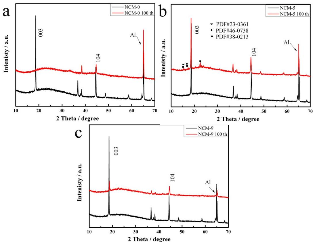
**Figure S5** XRD patterns of electrode before and after 100th cycles between 2.5-4.8 V.
