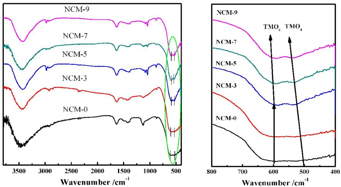
**Figure S3** FTIR spectra of the NCM-0, 3, 5, 7 and 9 samples.
