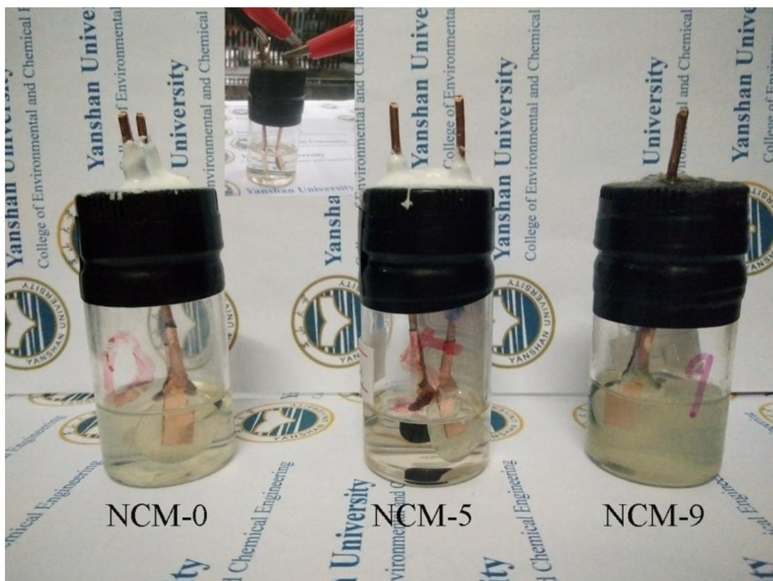
**Figure S6** Digital image of NCM-0, 5 and 9 electrodes were charged-discharged at 0.05 C to 4.8 V with two cycles. (The electrolyte consisting of  $\text{LiPF}_6$  (1 M) dissolved in ethylene carbonate, dimethyl carbonate, and diethyl carbonate mixed in a 1:1:1 volume ratio.)
