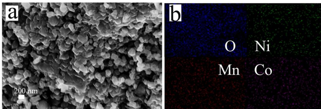
**Figure S4** SEM images of NCM-5 (a) and (b) EDS mapping images of the NCM-5.
