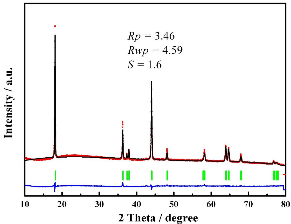
Figure S1 Observed refinement results of the as-prepared material NCM-3.
