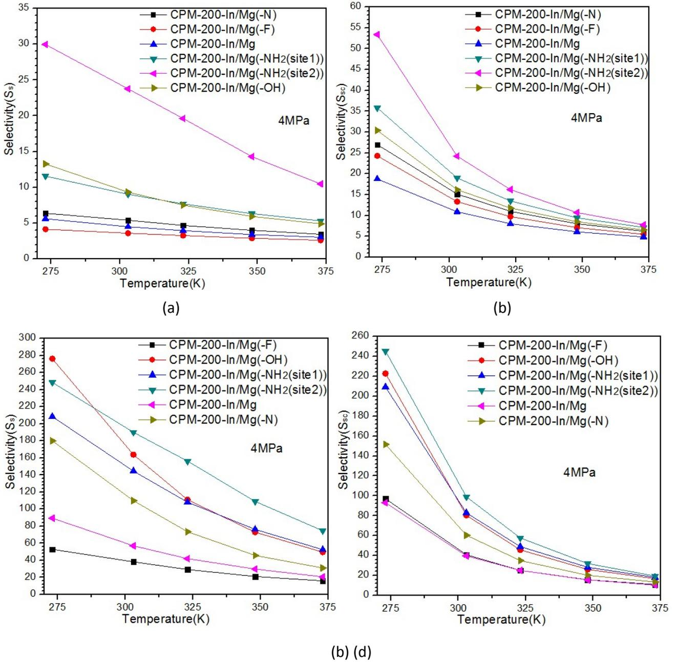
**Fig.S7** The effect of temperature on gas selectivity of materials in  $\text{CO}_2\text{-H}_2\text{S-CH}_4$ (a, b) and  $\text{SO}_2\text{-CO}_2\text{-N}_2$  (c, d) ternary mixtures systems at 4 MPa
