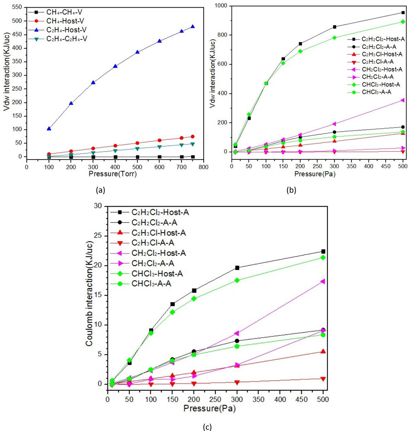
Fig.S4 The Vdw(a, b) and Coulomb(c) interactions between the host and adsorbate or among adsorbates respectively at 298 K
