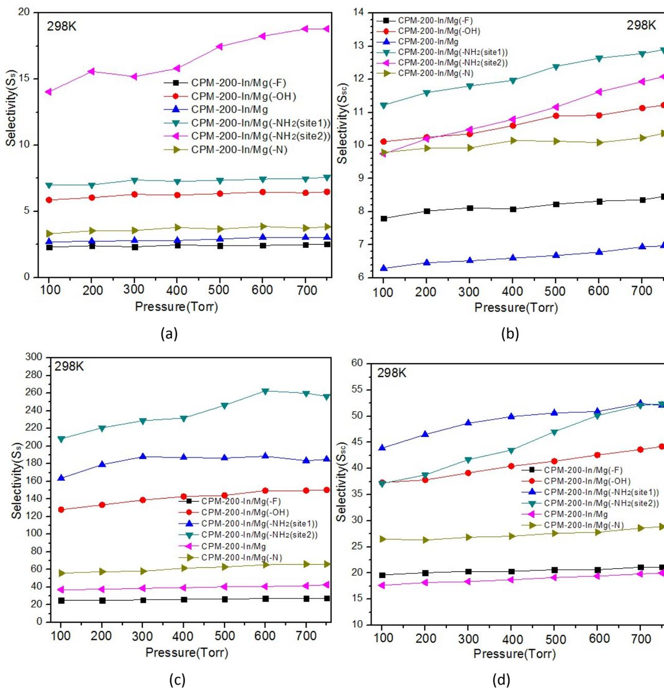
Fig.S5 Adsorption selectivities of MOFs in  $\text{CO}_2\text{-H}_2\text{S-CH}_4$ (a, b) and  $\text{CO}_2\text{-SO}_2\text{-N}_2$ (c, d) ternary mixtures systems at 298 K and low pressure area
