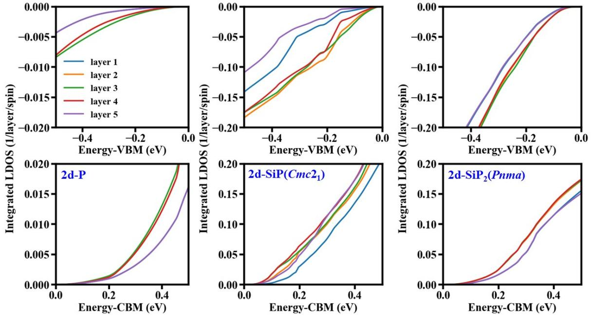
**Figure S3** Integrated layer-resolved local densities of states (LDOS) for 5-layer 2d-P, 2d-SiP( $Cmc2_1$ ), and 2d-SiP<sub>2</sub>( $Pnma$ ) computed using HSE. The k-point grids adopted in HSE calculations are scarcer compared to those in optB88-vdW (see Table S1). The integrated LDOS are calculated by integrating the LDOS over energy and given with respect to that for VBM (or CBM).
