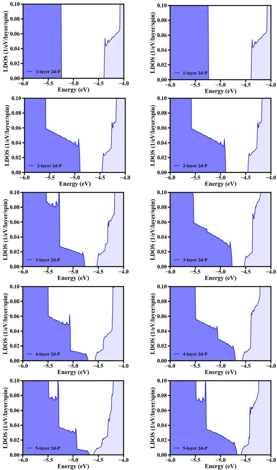
**Figure S2** Local densities of states (LDOS) projected on the outermost (left column) and central (right column) layers of 2d-P with different thicknesses computed using optB88-vdW functional. All energies are given with respect to the vacuum level.
