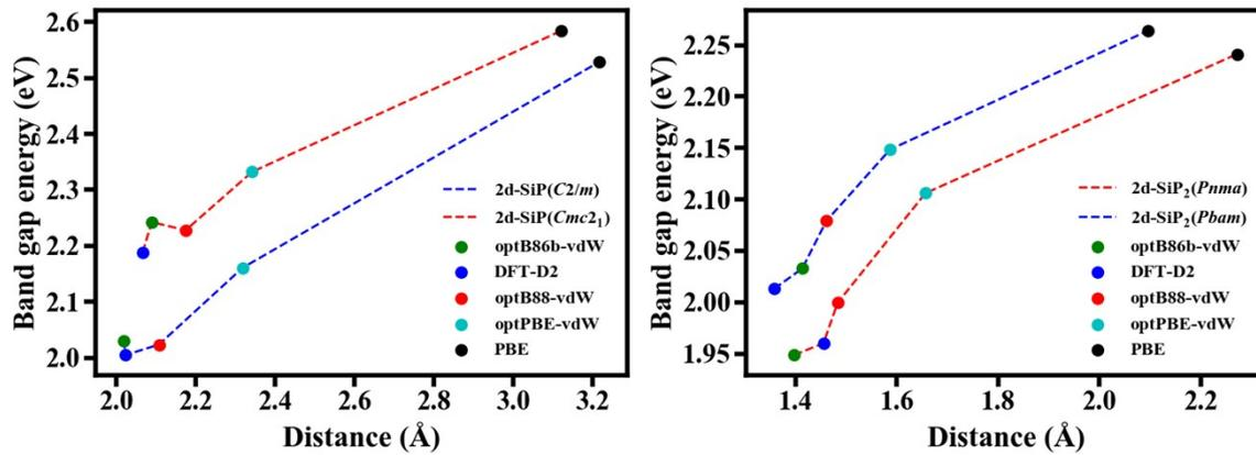
**Figure S1** HSE energy gaps of bilayer 2d-SiP (left) and 2d-SiP<sub>2</sub> (right). The results are given for structures from different functionals.
