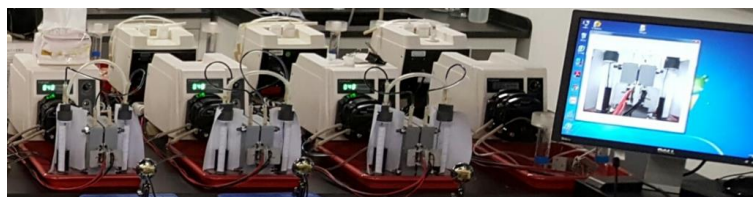
Fig. S4 Photograph of the multi-channel online monitoring system (OMS).
