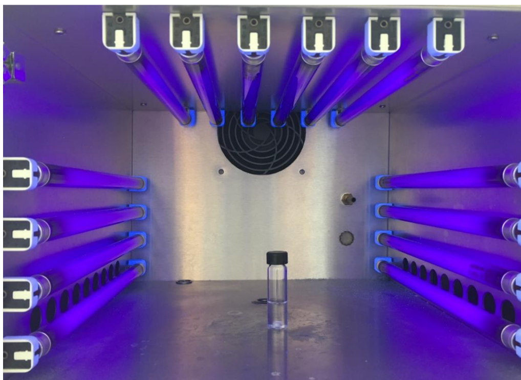
Figure S6. Picture of the UV photoreactor irradiation chamber (Luzchem UV lamp, model LZC 4V). It contains 14 lamps total, 6 installed on top and 8 installed on the sides (4 lamps on each side).
