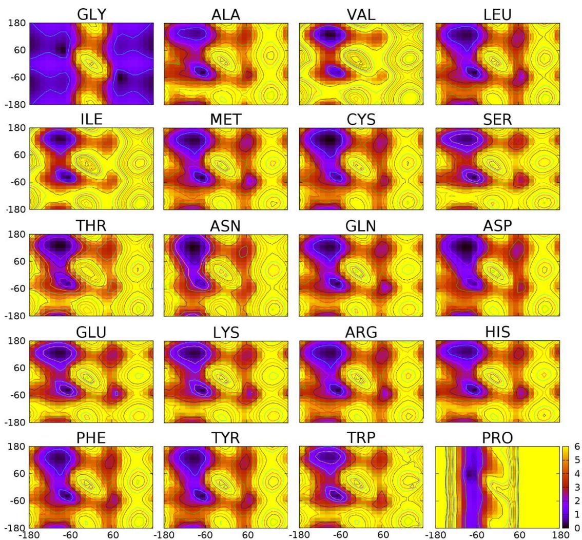
**Figure S4.** Backbone  $\phi/\psi$  adiabatic energy surfaces (in kcal/mol) of all 20 dipeptides in the HyRes model. The surface was calculated by energy minimization with  $\phi$  and  $\psi$  restrained at specified values. The surface was shifted such that the minimum value for each system was zero.
