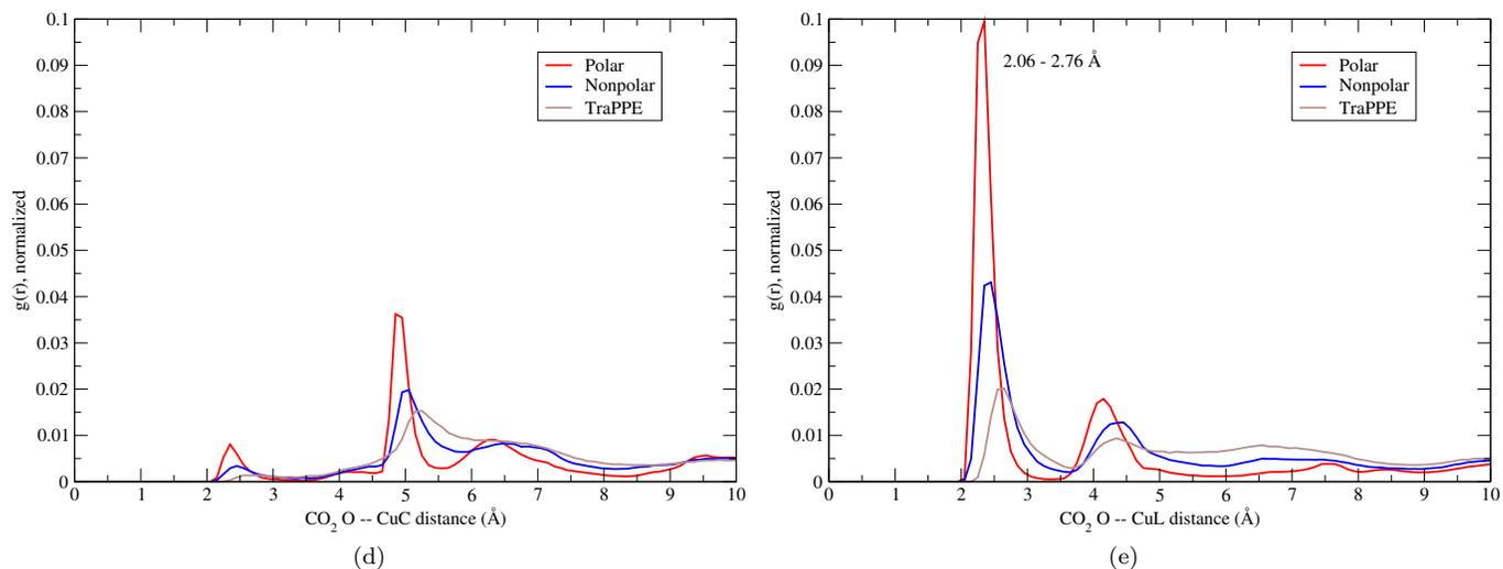
**Figure S11.** Radial distribution of CO<sub>2</sub> oxygen atoms with (a) CuC (the copper facing towards the rhombicuboctahedral cage), and (b) CuL at 298 K and 0.05 atm. Red = polar model; blue = nonpolar; brown = TraPPE.
