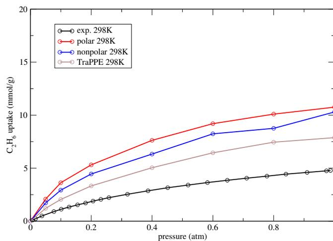
**Figure S42.**  $C_2H_6$  adsorption at 298 K from 0 to 1 atm. Black = experiment<sup>39</sup>; Red = polar model; blue = nonpolar; brown = TraPPE.
