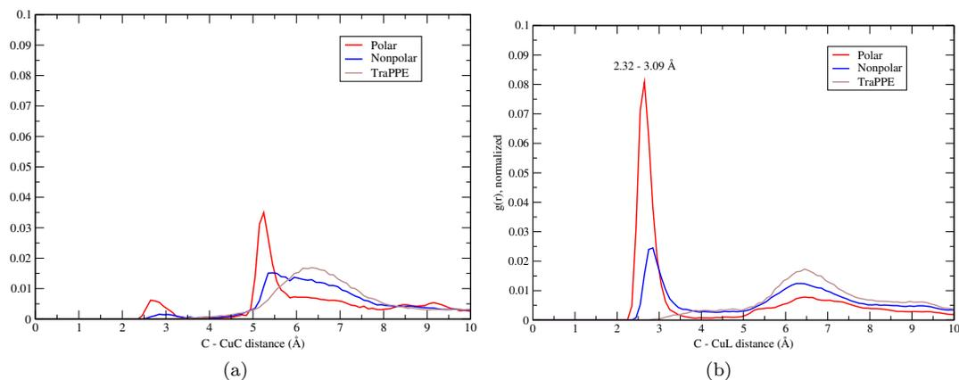
**Figure S34.** Sorption sites for (a) polar (site 2, CuC) and (b) nonpolar (site 4)  $C_2H_4$  as revealed by simulated annealing. The CuC - C distance for (a) is 2.62  $\text{\AA}$ .
