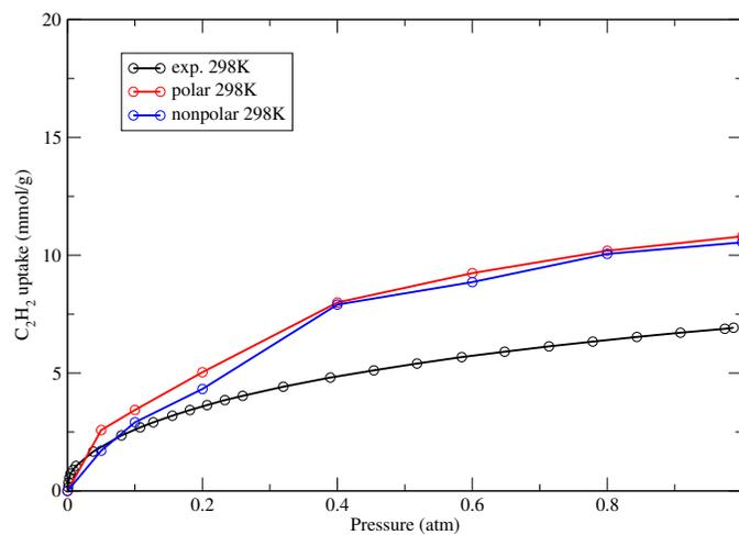
**Figure S28.**  $C_2H_2$  adsorption at 298 K from 0 to 1 atm. Black = experiment<sup>39</sup>; Red = polar model; blue = nonpolar.
