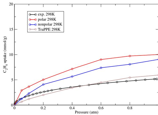
**Figure S35.**  $C_2H_4$  adsorption at 298 K from 0 to 1 atm. Black = experiment<sup>39</sup>; Red = polar model; blue = nonpolar; brown = TraPPE.
