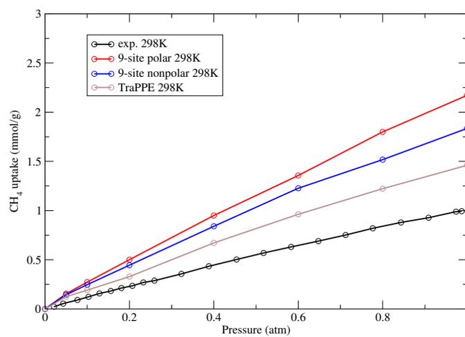
Figure S21. CH<sub>4</sub> adsorption at 298 K from 0 to 1 atm. Black = experiment<sup>39</sup>; Red = polar model; blue = nonpolar; brown = TraPPE.
