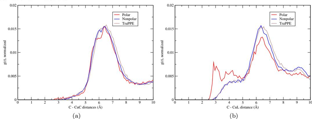
**Figure S41.** Sorption (site 4) for  $C_2H_6$  as revealed by simulated annealing.
