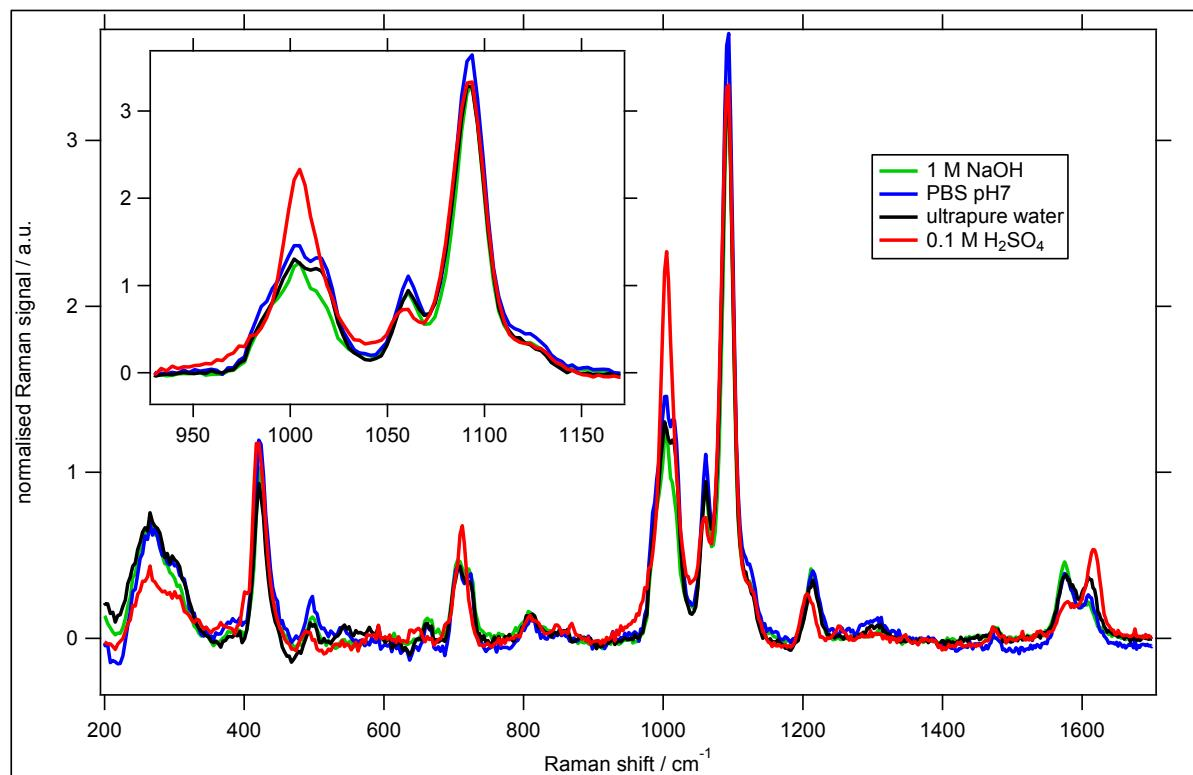
Figure S5 – Additional SER spectra of 4-mercaptopypyridine adsorbed on roughened gold in acidic and basic solutions.
