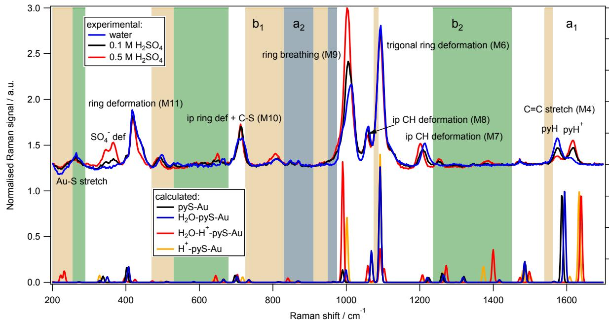
Figure S4 – Comparison between spectra from Figure 1 (main text) and the DFT calculation of various mercaptopyridine species bound to a single Au atom. The background is coloured according to the symmetry of the mode (with reference to the C<sub>2v</sub> symmetry of the pyridine ring).
