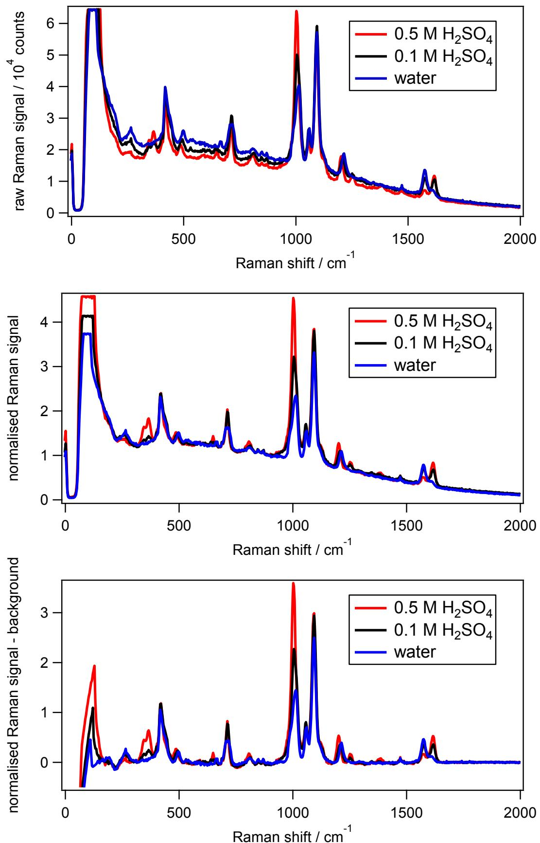
Figure S2. Raw, normalised and background-subtracted spectra for Figure 1 in the main text.
