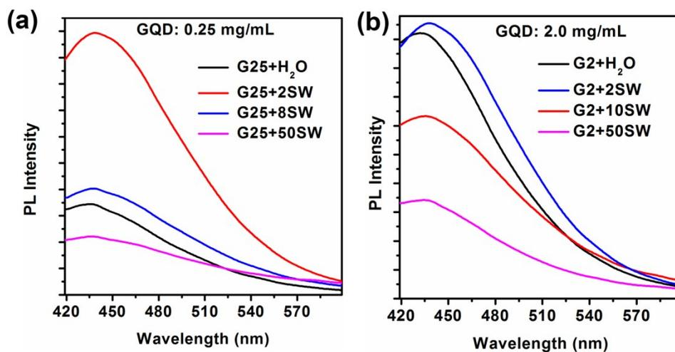
**Figure S6:** (a) Evolution of the PL spectra of GQDs (concentration of 0.25 mg/mL) in presence of SWCNTs at different concentrations. (b) The same for GQD concentration of 2 mg/mL. The code G25 is for 0.25 mg/mL and G2 is for 2.0 mg/mL of GQDs.
