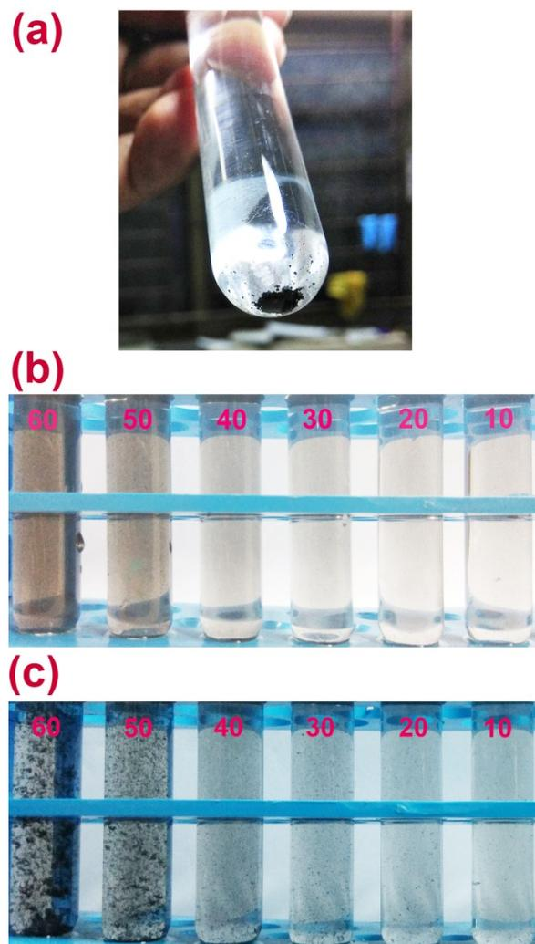
**Figure S1:** (a) Digital image of 0.6 mg SWCNTs in 10 mL MQ water before sonication showing precipitate. (b) Digital images of dispersion of SWCNTs in MQ water at different concentrations of SWCNTs (10-60  $\mu\text{g/mL}$  denoted as 10, 20, ....., 60, respectively, from right to left). (c) The stability of the dispersion 20 min after ultra-sonication, which shows agglomeration above 50  $\mu\text{g/mL}$ .
