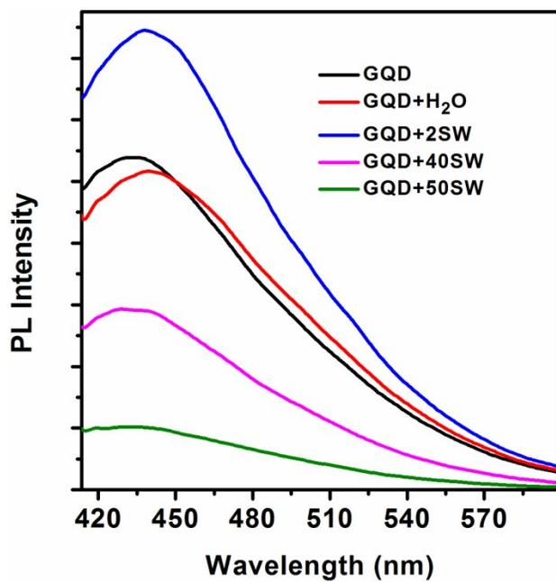
**Figure S4:** Dilution effect in the PL intensity of GQDs at 1.0 mg/ mL concentration
