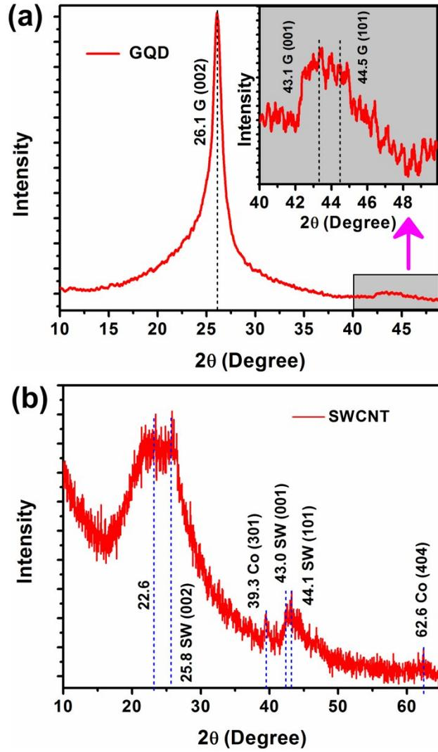
Figure S3: XRD pattern of (a) GQDs and (b) SWCNTs, showing the graphitic nature of the samples.
