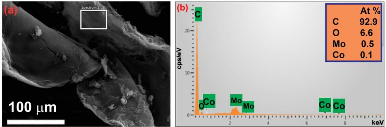
**Figure S2:** (a) FESEM image of SWCNTs, and (b) EDX spectrum of SWCNTs obtained from the square region shown in the (a)
