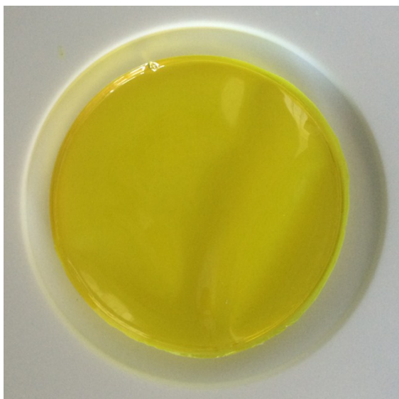
Figure S1. Photograph of a cast PIM-1 film (approx. 70mm diameter, 200 \mu\text{m} thickness)
