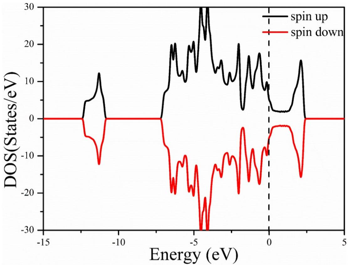
Fig. S2. The density of states of pristine  $\text{Mo}_2\text{CO}_2$ . The dashed line at energy zero represents the Fermi level.
