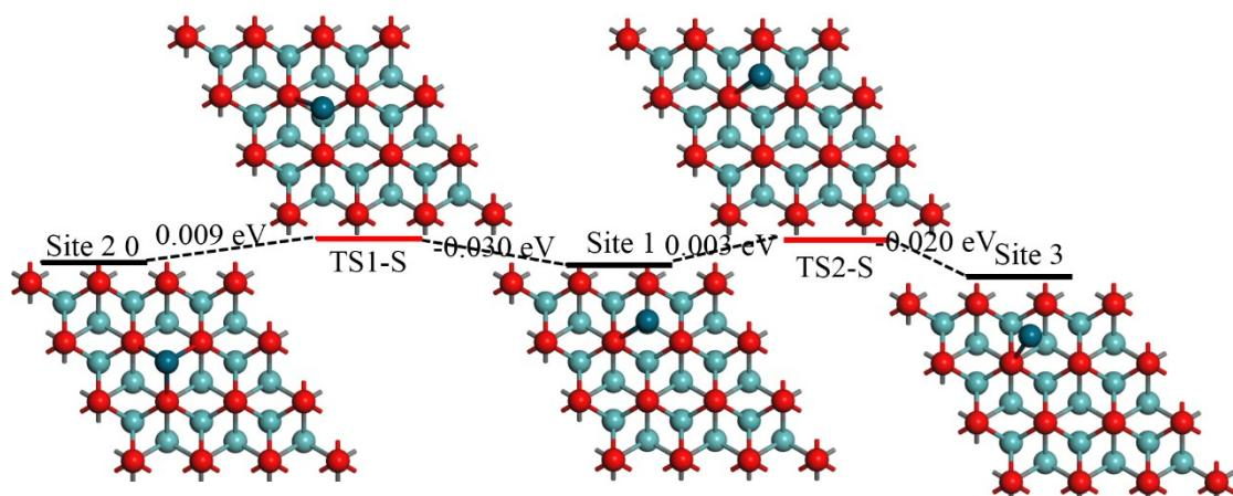
Fig. S1. Diffusion pathways of single Pd atom on the pristine Mo<sub>2</sub>CO<sub>2</sub> monolayer.
