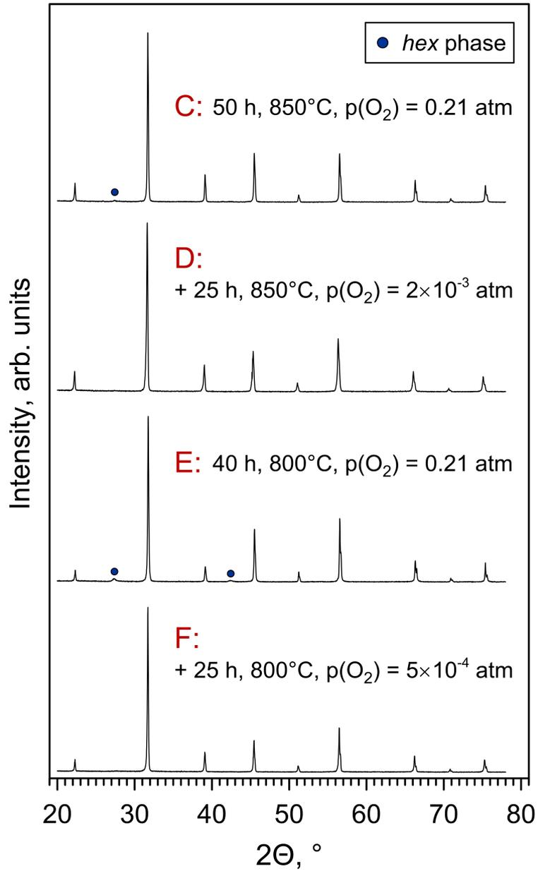
Figure S2. XRD patterns of BSCF samples after annealing in air at 800 or 850°C for 40-50 h (C and E) and then for 25 h at lower  $p(\text{O}_2)$  at the same temperature (D and F, respectively). The conditions C-F correspond to that marked in Fig.3. Reflections of the hexagonal phase are marked according to Ref.[16].
