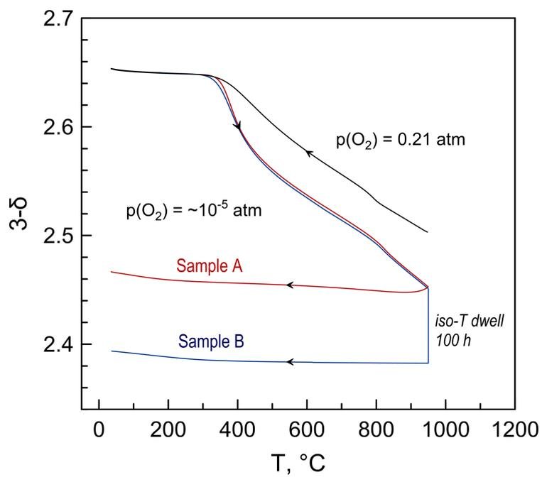
Figure S4. Changes of oxygen nonstoichiometry in BSCF samples on cooling in air and subsequent heating/cooling cycle in inert gas flow. Heating/cooling rate is 2°C/min. After reduction in inert gas, the samples were subjected for the neutron diffraction studies.
