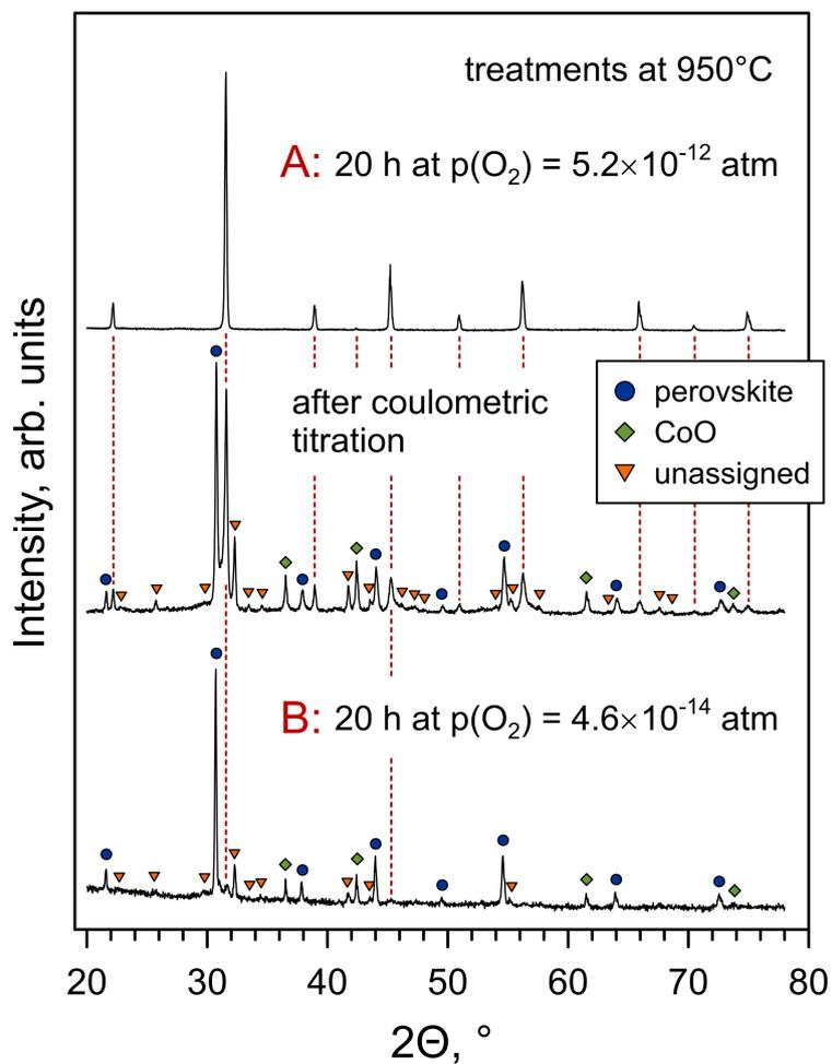
Figure S1. XRD patterns of BSCF samples after low- $p(\text{O}_2)$  treatments at 950°C: (center) after stability boundary determination by coulometric titration, and (A and B) after annealing for 20 h at different  $p(\text{O}_2)$ . The conditions A and B correspond to that marked in Fig.1. Vertical dotted lines mark the reflections of cubic perovskite BSCF.
