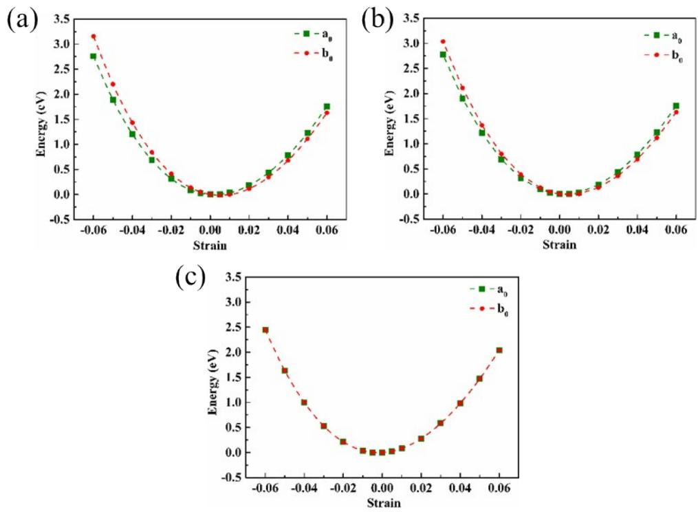
**Fig. S3** Energy-strain relationships along the  $a_0$  and  $b_0$  directions of bilayer InSe (a) adsorbed structures of O atom on  $B_b$  site, (b) inserted O atom in  $I_b1$  site and (c) substituted structure of Se by O atom at  $S_b2$  site.
