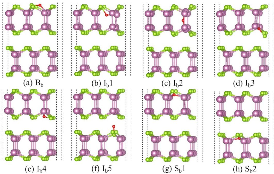
**Fig. S2** Adsorbed structures of O atom on different sites: (a) B<sub>b</sub>, (b) I<sub>b</sub>1, (c) I<sub>b</sub>2, (d) I<sub>b</sub>3, (e) I<sub>b</sub>4 and (f) I<sub>b</sub>5, and substituted structures of (g) S<sub>b</sub>1 and (h)S<sub>b</sub>2.
