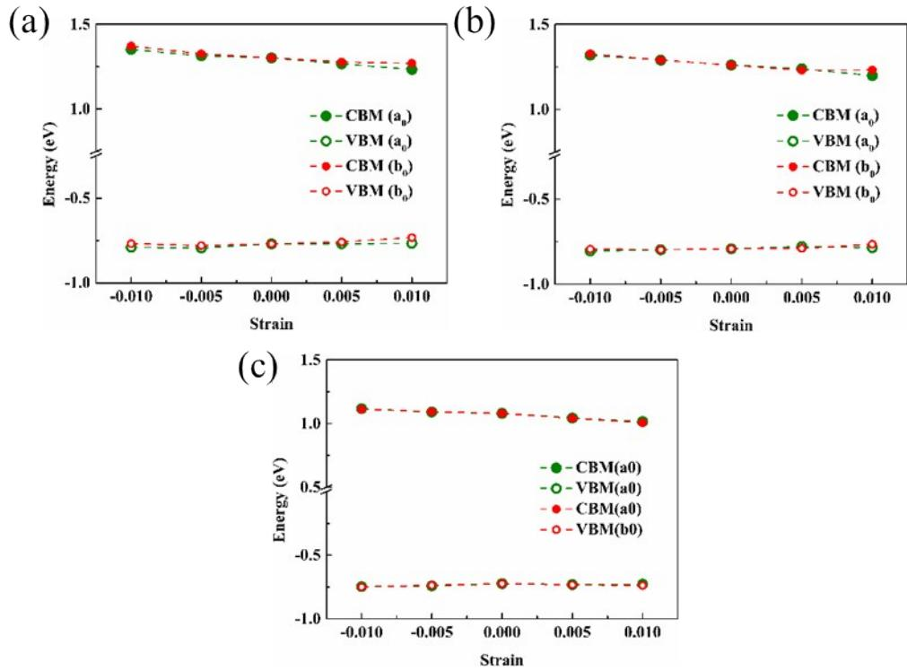
**Fig. S4** Shifts of CBM and VBM under uniaxial strain along  $a_0$  and  $b_0$  directions of monolayer InSe (a) adsorbed structures of O atom on  $B_b$  site, (b) inserted O atom in  $I_b1$  site and (d) substituted structure of Se by O atom at  $S_{b2}$  site.
