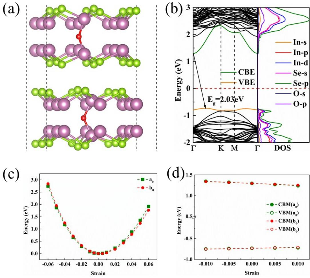
**Fig.S5** (a) Optimized structure of bilayer InSe inserted O atom into  $I_b2$  site of each layer and corresponding (b) Electronic band structure and density of states plots. The Fermi level is located at energy zero. (c) Energy-strain relationship and (d) shifts of CBM and VBM under uniaxial strain along  $a_0$  and  $b_0$  direction of bilayer InSe inserted O atom into  $I_b2$  site of each layer.
