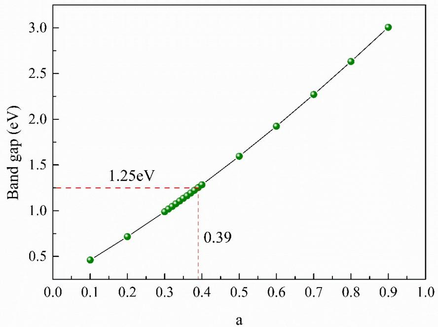
**Fig. S1** The relationship between mixing parameter  $\alpha$  and bandgap of bulk InSe
