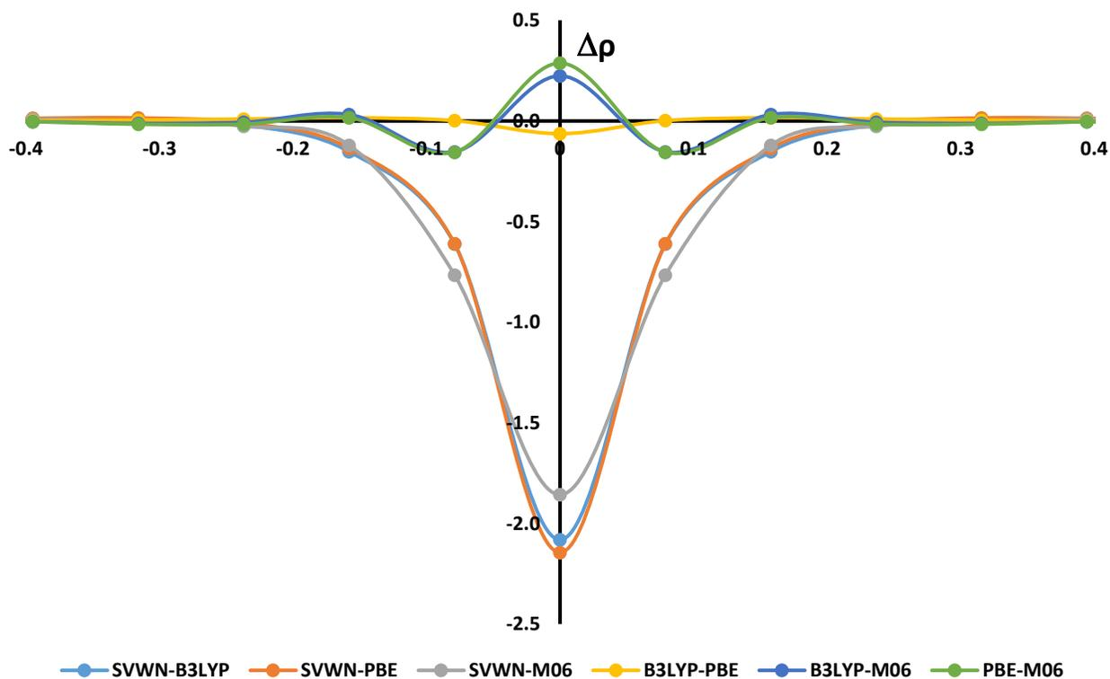
Figure S6. The six density difference plots of the four studied density functionals,  $N^{3+}$  ion. (aug-cc-pwCV5Z)
