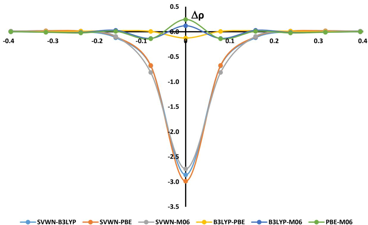
Figure S8. The six density difference plots of the four studied density functionals,  $O^{4+}$  ion. (aug-cc-pwCV5Z)
