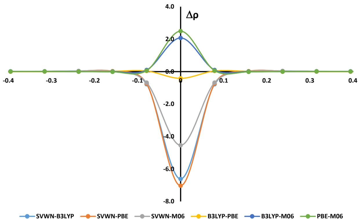
Figure S13. The six density difference plots of the four studied density functionals, Ne<sup>8+</sup> ion. (aug-cc-pwCV5Z)
