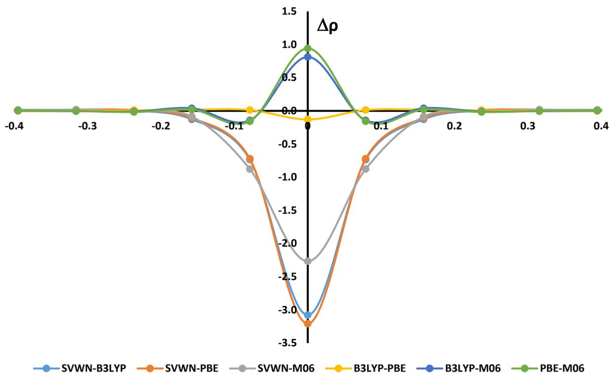
Figure S7. The six density difference plots of the four studied density functionals,  $N^{5+}$  ion. (aug-cc-pwCV5Z)
