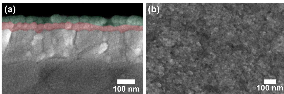
**Figure S4.** Scanning electron microscopy (SEM) images of (a) cross section and (b) top morphology of NC ink prepared from 1.15:1 ratio of  $\text{CH}_3\text{NH}_3\text{Br}:\text{PbBr}_2$ , spin coated on top of ITO/PEDOT:PSS. The green and red layers in (a) represent the perovskite emitter and PEDOT:PSS layer, respectively.
