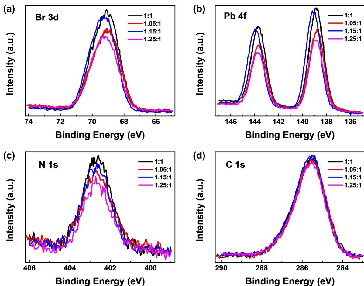
**Figure S2.** XPS (a) Br 3d spectra, (b) Pb 4f spectra, (c) N 1s spectra, and (d) C 1s spectra of the NCs prepared by varying the  $\text{CH}_3\text{NH}_3\text{Br}:\text{PbBr}_2$  ratios viz. 1:1 (black), 1.05:1 (red), 1.15:1 (blue) and 1.25:1 (magenta).
