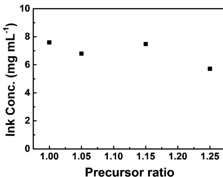
**Figure S3.** NC ink concentration/ NC synthesis yield for the NCs prepared from the various  $\text{CH}_3\text{NH}_3\text{Br}:\text{PbBr}_2$  ratios viz., 1:1, 1.05:1, 1.15:1, and 1.25:1.
