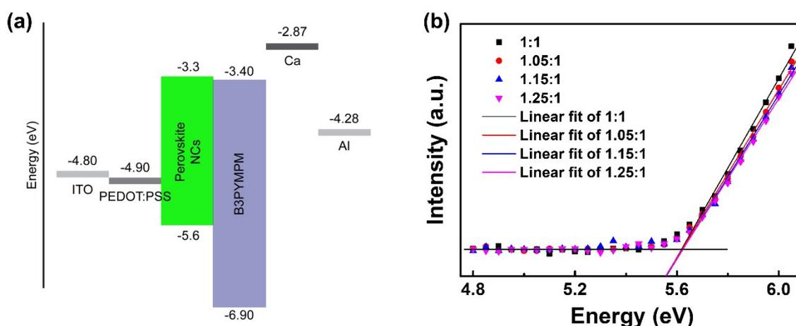
**Figure S5.** (a) Schematic diagram of the flat band energy levels of the LED device stack. (b) Valence band maxima (VBM) of the various NC inks prepared from the CH<sub>3</sub>NH<sub>3</sub>Br:PbBr<sub>2</sub> ratios of 1:1 (black), 1.05:1 (red), 1.15:1 (blue), and 1.25:1 (magenta), calculated from the photoelectron spectroscopy in air (PESA) measurements.
