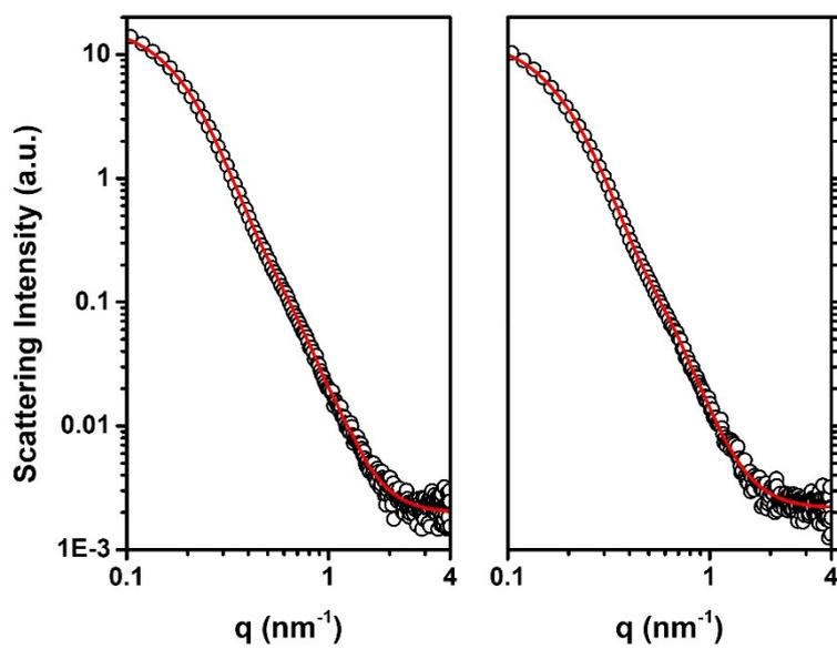
**Figure S1.** Exemplary fits for the scattering curves obtained from the small angle X-ray scattering (SAXS) measurements for CH<sub>3</sub>NH<sub>3</sub>Br:PbBr<sub>2</sub> ratios of 1:1 (left) and 1.15:1 (right).
