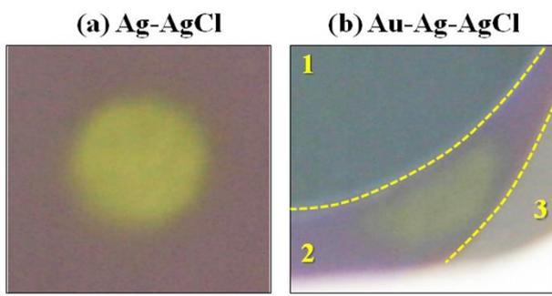
SI. 10 (a) Ag-AgCl sample and (b) Au-Ag-AgCl sample irradiated by green beam of Nd:YAG laser. In (b) part 1 is Au-Ag-AgCl thin film, part 2 is Ag-AgCl thin film and 3 is Ag thin film.
