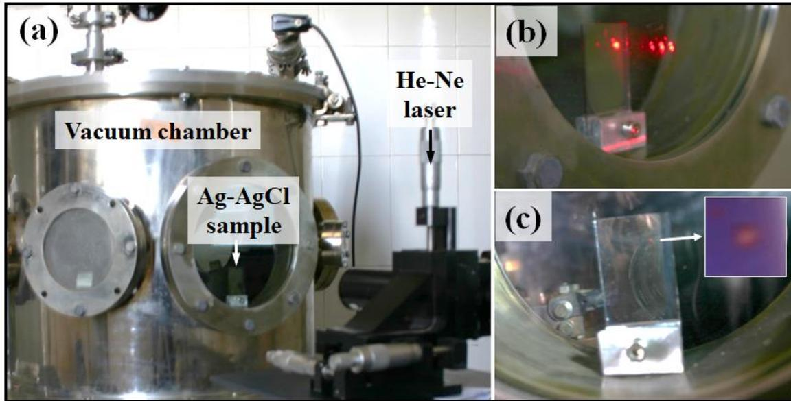
SI. 11 (a) The Ag-AgCl sample is located inside vacuum chamber, (b) He-Ne laser beam is irradiating to Ag-AgCl sample while it is inside the vacuum chamber, (c) after laser irradiation the colour change of the sample is obvious.
