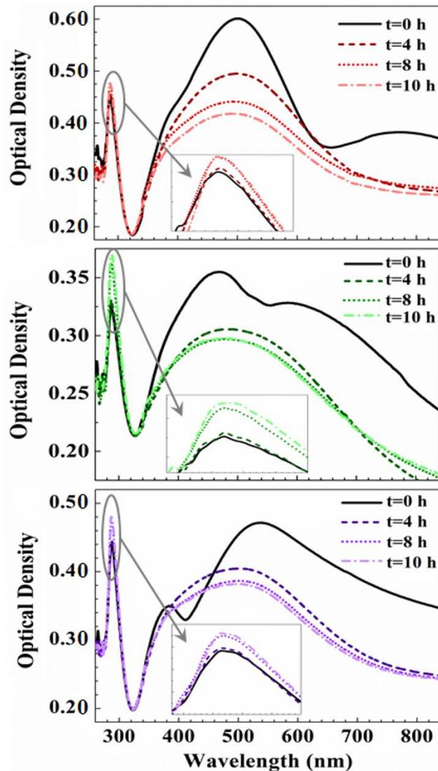
Sl. 8 OD spectra of coloured spots on Ag-AgCl thin film irradiated by (a) He-Ne laser ( $\lambda=632.8\text{nm}$ ), (b) Nd:YAG laser ( $\lambda=532\text{nm}$ ) and (c) violet diode laser ( $\lambda=405\text{nm}$ ) before white light irradiation (black solid curves), after three step white light irradiation in 4h, 8h and 10h (coloured curved).
