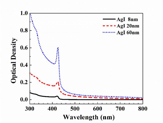
SI. 5 OD spectra of AgI thin films with different thickness 8nm, 20nm and 60nm on quartz substrate.
