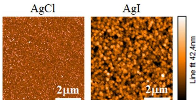
SI. 1 AFM image of AgCl and AgI thin films (thickness is 50nm).
