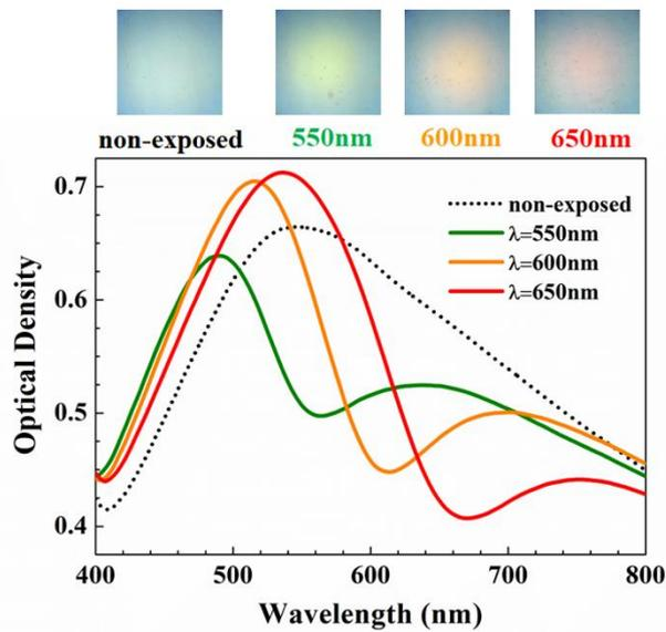
SI. 6 OD spectra of Ag-AgCl thin film before laser irradiation (black dotted curve) and after laser irradiation (solid curves) with different wavelengths 550nm, 600nm and 650nm. The colour spots on Ag-AgCl related to each wavelength is also shown.
