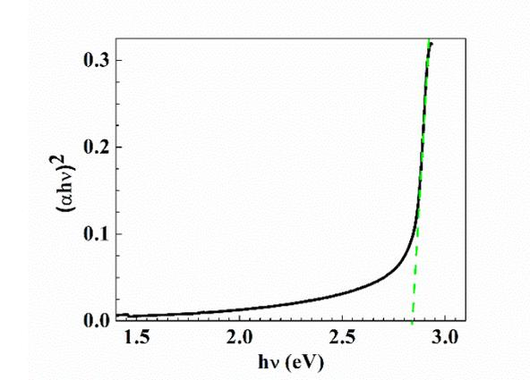
SI. 3 Tauc plot for determining the direct band gap energy of AgI.
