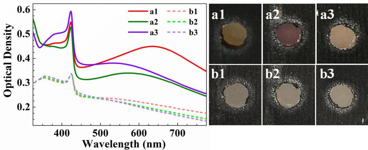
SI. 9 OD spectra of coloured spots on Ag-AgI irradiated by He-Ne laser, Nd:YAG laser and violet-diode laser; before white light irradiation indicated by a1, a2 and a3, after white light irradiation for 8h shown by b1, b2 and b3, respectively.
