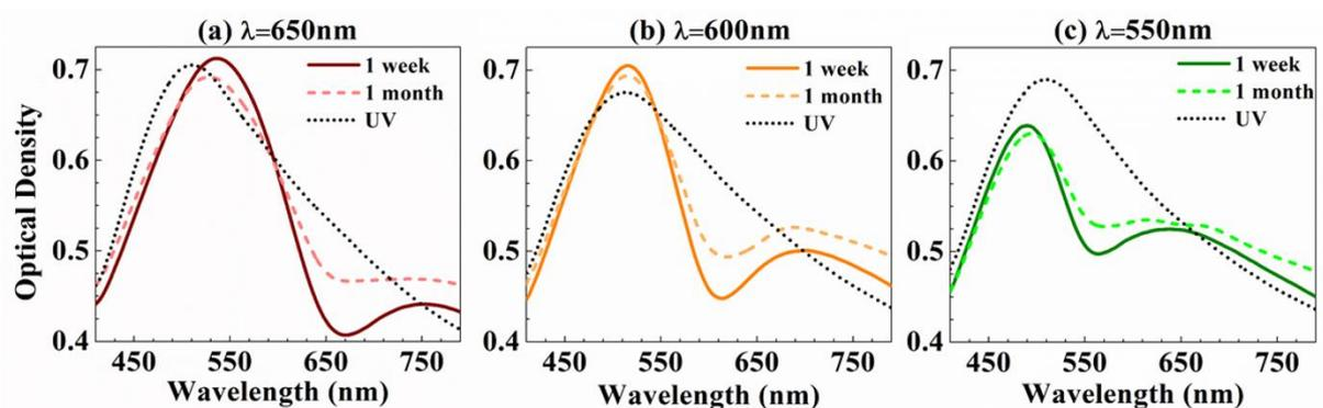
SI. 7 OD spectra of Ag-AgCl thin film after laser irradiation with wavelengths (a) 650nm, (b) 600nm and (c) 550nm. The OD spectra were measured one week after laser irradiation (solid curves) and one month after laser irradiation (dashed curves). The dotted curves are the OD spectra after the sample are irradiated by UV light.
