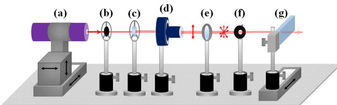
SI. 2 Scheme of the setup used for irradiating the samples: (a) Laser and its xyz stage, (b) ND filter, (c) Concave lens, (d) Glan-Taylor calcite polarizer, (e) Depolarizer, (f) Aperture, (g) Sample and its holder.
