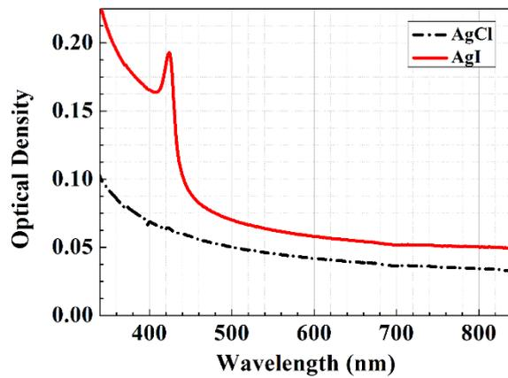
SI. 4 OD spectra of AgCl (black dash-dotted curve) and AgI (red solid curve).
