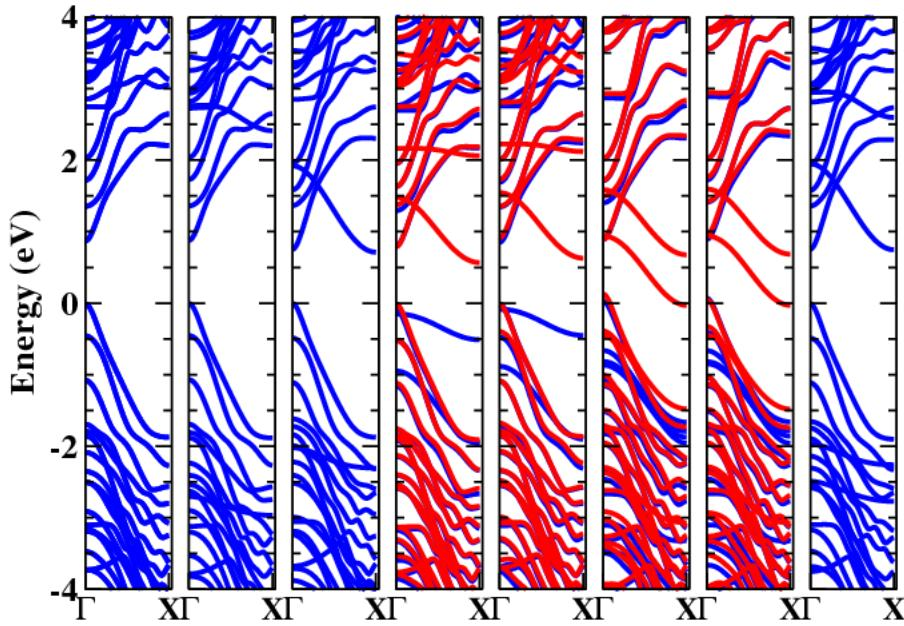
**Fig. 5** Band structures of various configurations of 18-CC-BN-ABNCNR: (a)  $c_0$ , (b)  $c_1$ , (c)  $c_2$ , (d)  $c_3$ , (e)  $c_4$ , (f)  $c_5$ , (g)  $c_6$ , and (h)  $c_7$ . Configurations are explained in the main text.
