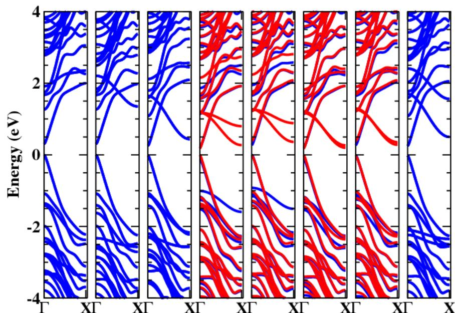
**Fig. 4** Band structures of various configurations of 18-CC-CC-ABNCNR: (a)  $b_0$ , (b)  $b_1$ , (c)  $b_2$ , (d)  $b_3$ , (e)  $b_4$ , (f)  $b_5$ , (g)  $b_6$ , and (h)  $b_7$ . Configurations are explained in the main text.
