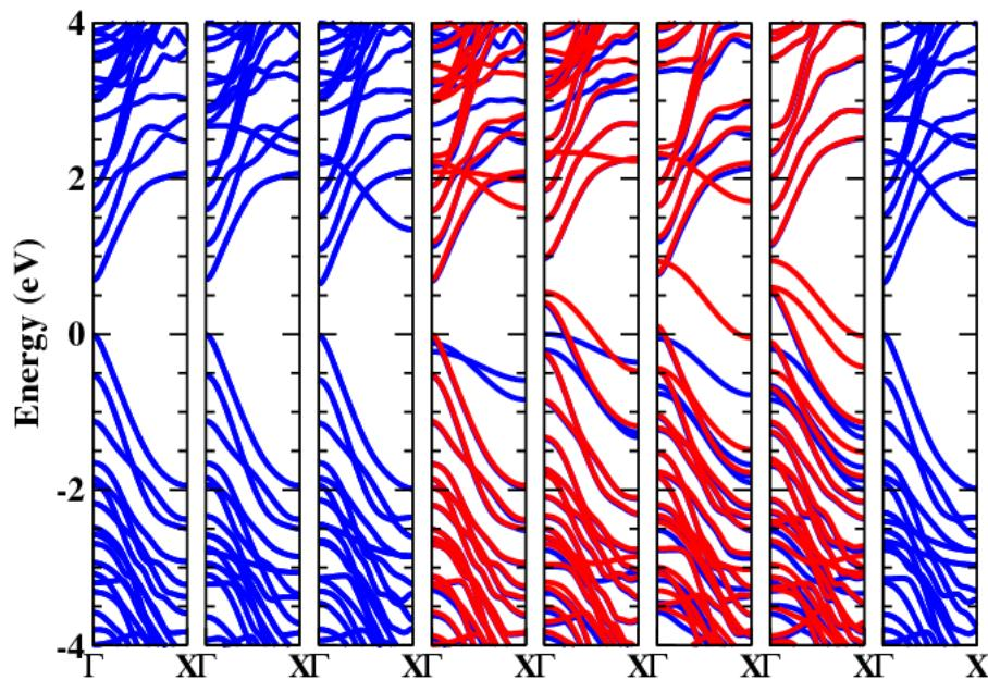
**Fig. 3** Band structures of various configurations of 18-BN-BN-ABNCNR: (a)  $a_0$ , (b)  $a_1$ , (c)  $a_2$ , (d)  $a_3$ , (e)  $a_4$ , (f)  $a_5$ , (g)  $a_6$ , and (h)  $a_7$ . Configurations are explained in the main text.
