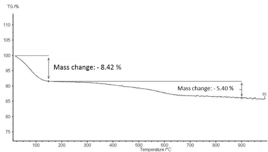
**Figure S4.** Thermogravimetric analysis (TGA) profile for hi-MSP-CLZ<sub>i</sub> (top) and ho-MSP-CLZ<sub>i</sub> (bottom). Decomposition temperatures of CLZ is within the range of 150-900°C. Mass changes from 20°C to 150 °C are related to presence of water and solvent.
