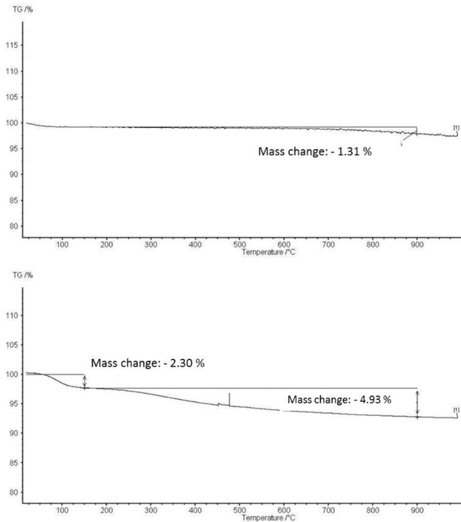
**Figure S2.** Thermogravimetric analysis (TGA) profile for ho-MSP (top) and hi-MSP (bottom). Decomposition temperatures of silanol groups is within the range of 150-900°C. Mass changes from 20°C to 150 °C are related to presence of water and solvent.
