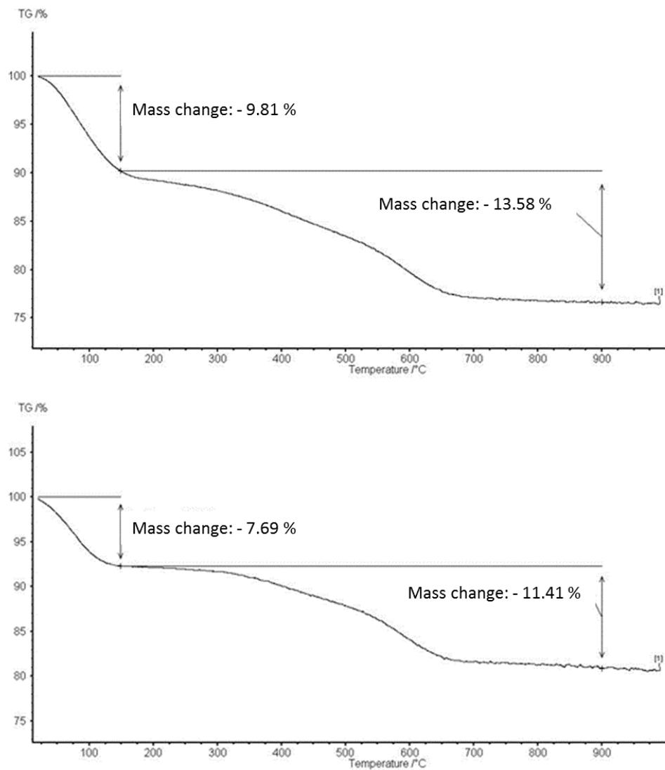
**Figure S3.** Thermogravimetric analysis (TGA) profile for hi-MSP-CLZ<sub>h</sub> (top) and ho-MSP-CLZ<sub>h</sub> (bottom). Decomposition temperatures of CLZ is within the range of 150-900°C. Mass changes from 20°C to 150 °C are related to presence of water and solvent.
