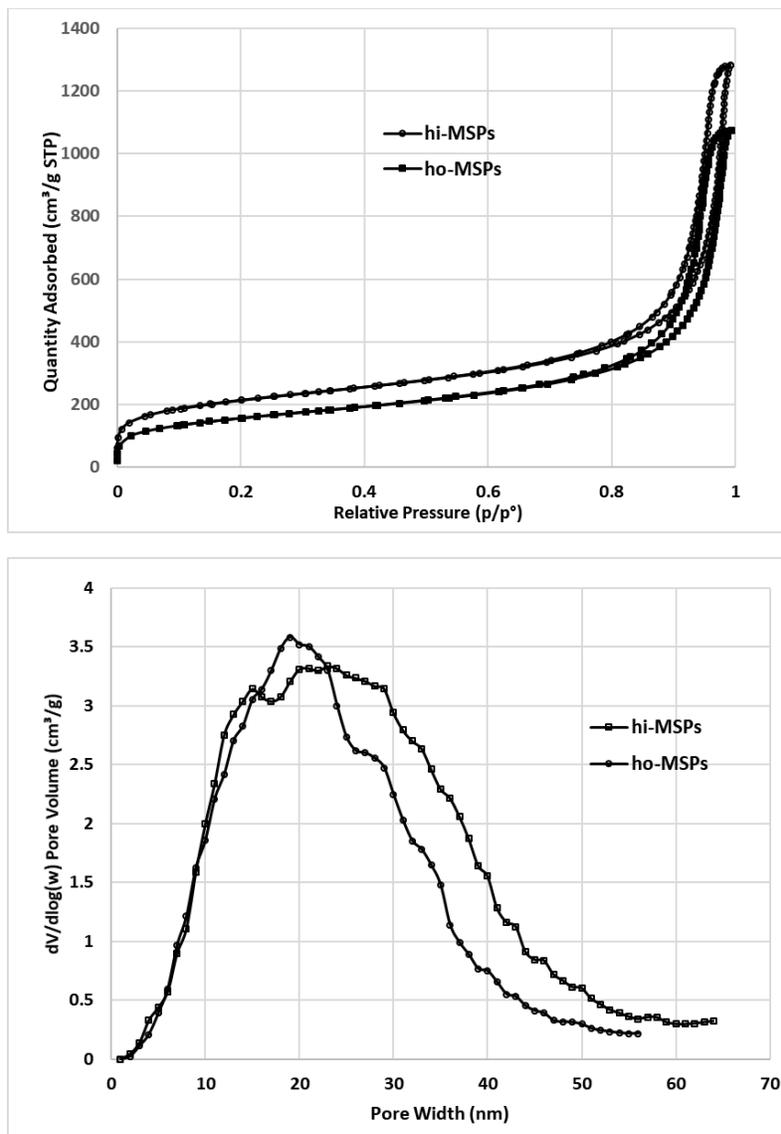
**Figure S1.** Nitrogen adsorption/desorption isotherm (top), and pore size distribution (bottom) obtained from BJH model using desorption branch of isotherm for hi-MSPs and ho-MSPs.
