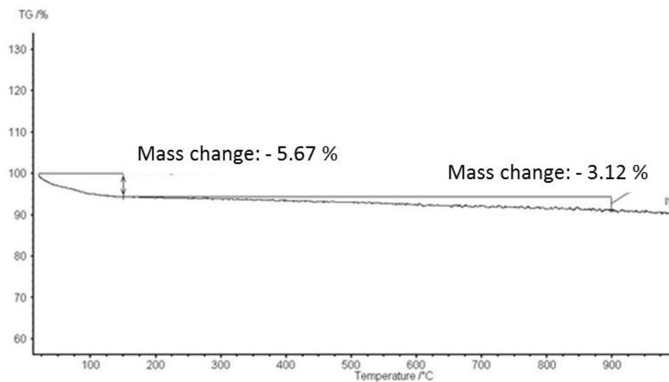
**Figure S5.** Thermogravimetric analysis (TGA) profile for hi-MSP-CLZ<sub>1</sub> (top – black line) and ho-MSP-CLZ<sub>1</sub> (bottom). Decomposition temperatures of CLZ is within the range of 150-900°C. Mass changes from 20°C to 150 °C are related to presence of water and solvent,
