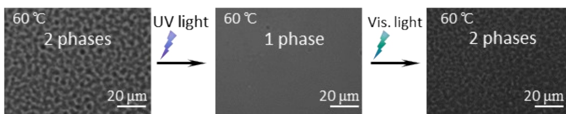
Fig. S2 Optical micrographs of PS solution (polymer concentration = 5 wt%) at 60 °C. The solution was irradiated with UV light ( \lambda = 365 nm, intensity = 150 mW/cm 2 ), and then irradiated with visible light ( \lambda = 435 nm, intensity = 200 mW/cm 2 ).
