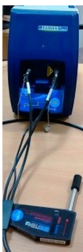
Fig S1: Photo of the Raman Spectrometer used for our measurement
