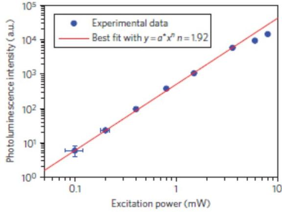
**Figure S1.** Upconversion photoluminescence intensity as a function of excitation power. Reprinted with permission from Ref. 7 (Copyright 2012, Nature Publishing Group). The upconversion intensity of IR806-sensitized NaYF<sub>4</sub>:Yb,Er nanoparticles (integrated in the range 500–685 nm) as a function of excitation power from an 800 nm laser. The number of photons which are required to populate the upper emitting state under unsaturated condition can be obtained by the relation,
