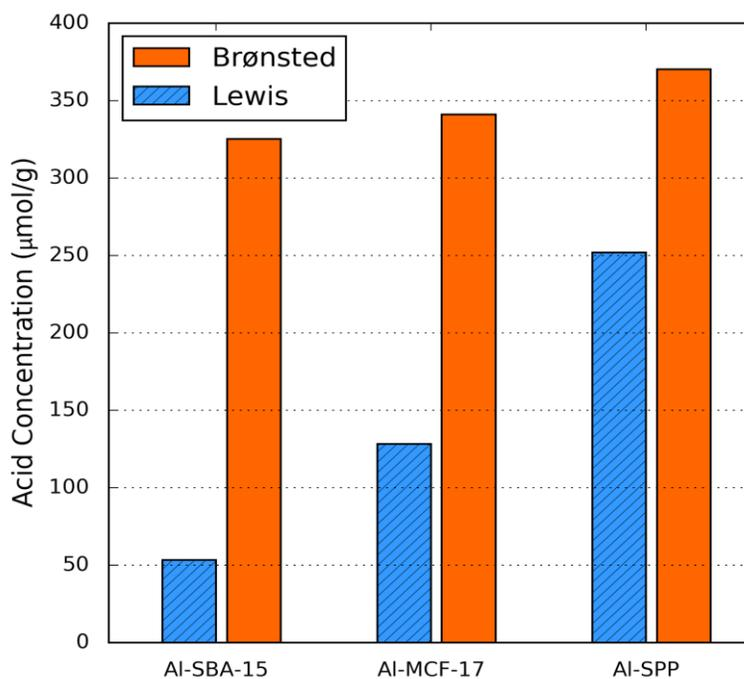
**Figure S4.** Total Brønsted and Lewis acid site concentration for three different aluminum modified silica supports. The acid sites were quantified by titrating the sites with pyridine and analyzing the corresponding IR bands.
