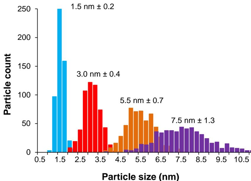
**Figure S5.** Average particle sizes and size distributions of platinum nanoparticles characterized by TEM. The platinum nanoparticles were synthesized by a polyol technique, in which the size of the particles was controlled by a capping agent, polyvinylpyrrolidone (PVP).
