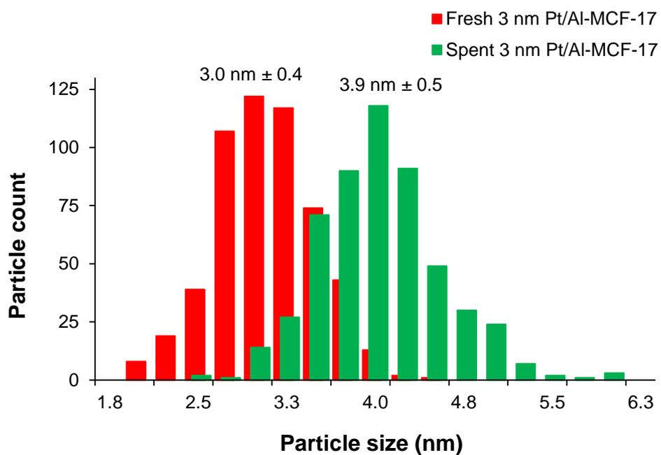
**Figure S7.** The difference in platinum particle size and size distribution before (red) and after (green) the reaction for 3.0 nm Pt/Al-MCF-17 as characterized by TEM.
