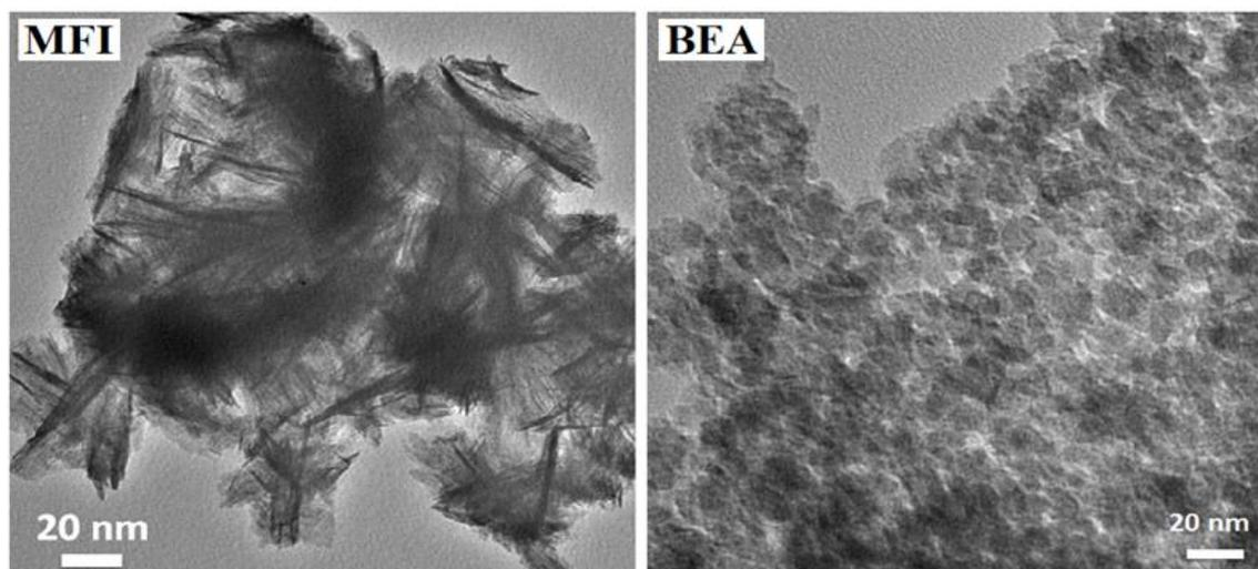
**Figure S1.** TEM images of mesoporous MFI (left) and BEA (right) zeolites. Physicochemical properties are given in Tables 1 and S1.
