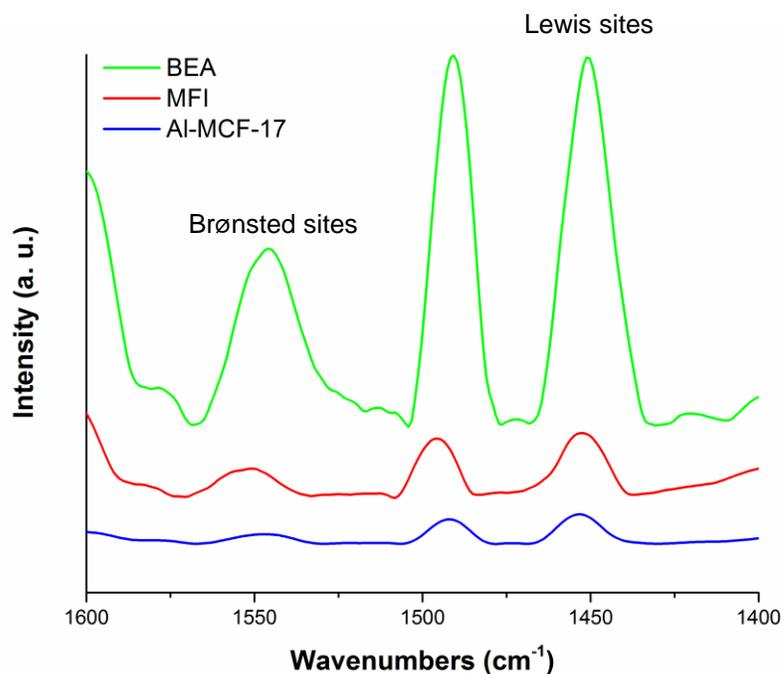
**Figure S2.** FT-IR spectra of pyridine molecules adsorbed on Brønsted and Lewis acid sites of mesoporous BEA and MFI zeolites and mesoporous Al-MCF-17. The amount of Brønsted and Lewis acid sites can be calculated by correlating the adsorbed pyridine molecules to the acid sites.
