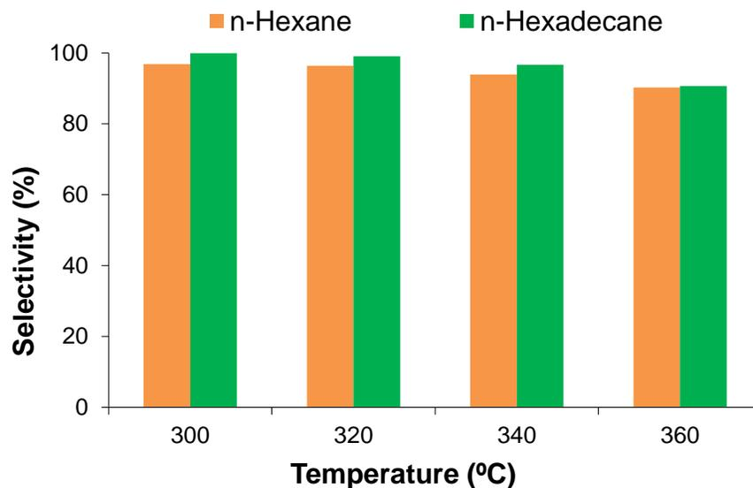
**Figure S9.** Total isomer selectivity for gas-phase n-hexane and n-hexadecane conversions on Pt/Al-MCF-17 at 1 bar and 300 – 360 °C. Both reactants were converted to their corresponding isomers with nearly 100% selectivity despite large difference in molecular weight.
