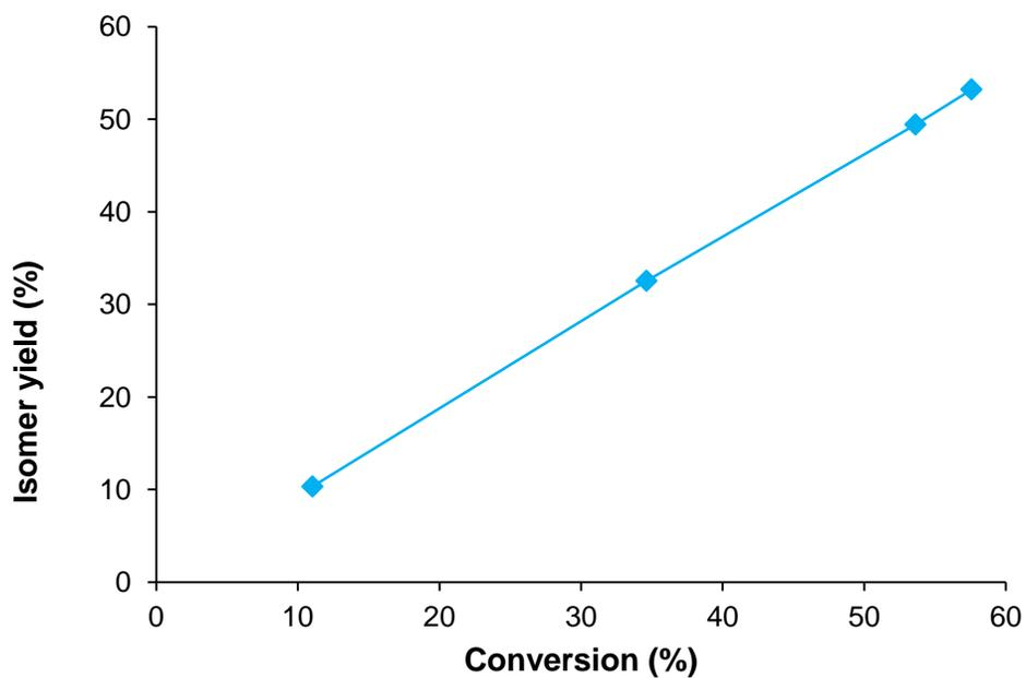
**Figure S8.** Isomer yield as a function of reaction conversion. The conversion was controlled by increasing catalyst bed, i.e., residence time while keeping reaction temperature constant at 300 °C and 1 bar.
