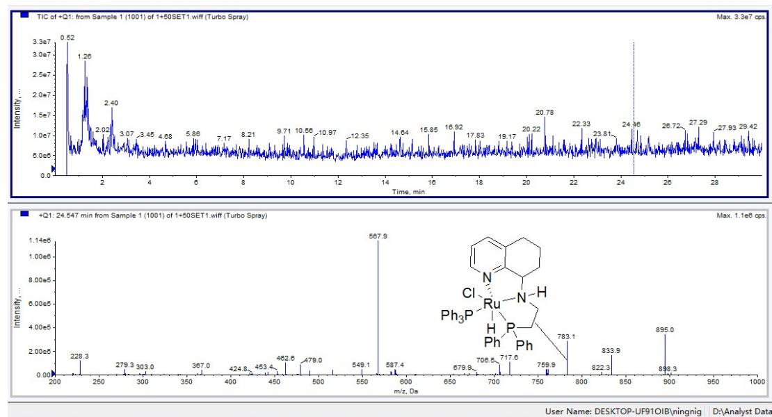
**Figure S5.** ESI mass spectra of **C** and benzyl alcohol in the presence of *t*-BuOK (1 eq.) in CDCl<sub>3</sub> at 45 °C, recorded after 24 hours using the 3200 QTRAP 1200 infinity series instrument. Acetonitrile:water = 70:30, flow rate = 1 ml / min, electronic energy = 50 eV, Q1MS scan range = 200~1000. The base peak corresponds to the intermediates [(M-3)+1]<sup>+</sup> at *m/z* 761.3 and [(M-3)+Na]<sup>+</sup> at *m/z* 823.9.
