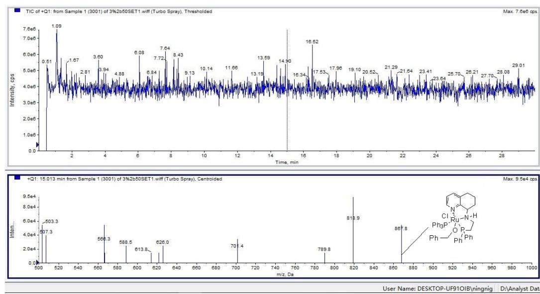
**Figure S4:** ESI mass spectra of **C** and benzyl alcohol in the presence of *t*-BuOK (1 eq.) in CDCl<sub>3</sub> at 45 °C, recorded after 24 hours using the 3200 QTRAP 1200 infinity series instrument. Acetonitrile:water = 70:30, flow rate = 1 ml / min, electronic energy = 50 eV, Q1MS scan range = 500~1000. The base peak corresponds to the intermediates [(M-2'')+1] at *m/z* 867.8.
