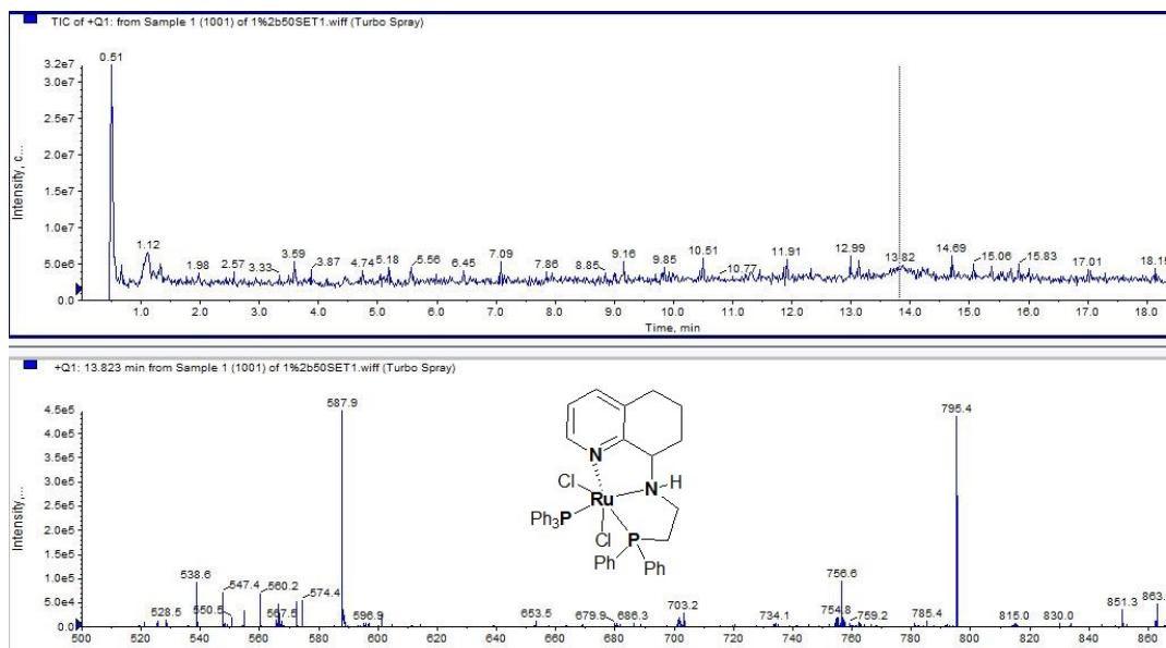
**Figure S1.** ESI mass spectra of **C** in  $\text{CDCl}_3$  (1 mL) recorded using the 3200 QTRAP 1200 infinity series instrument. Acetonitrile:water = 70:30, flow rate = 1 ml / min, electronic energy = 50 eV, Q1MS scan range = 500~900. The base peak corresponds to  $[\mathbf{C}+1]^+$  at  $m/z$  795.4.
