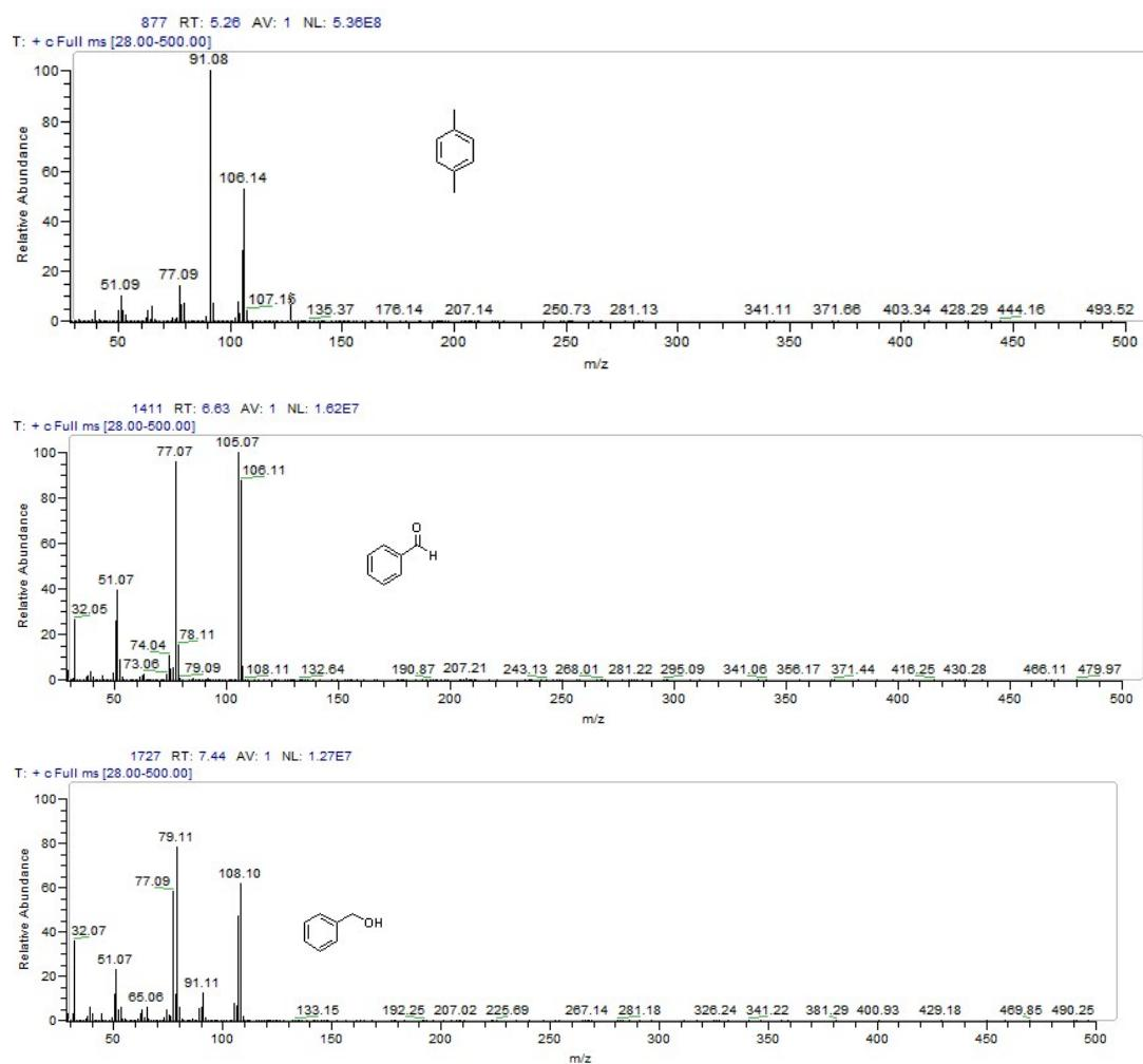
**(b) GC-MS spectra of the product of benzyl alcohol in AAD reaction at 160 °C.**
