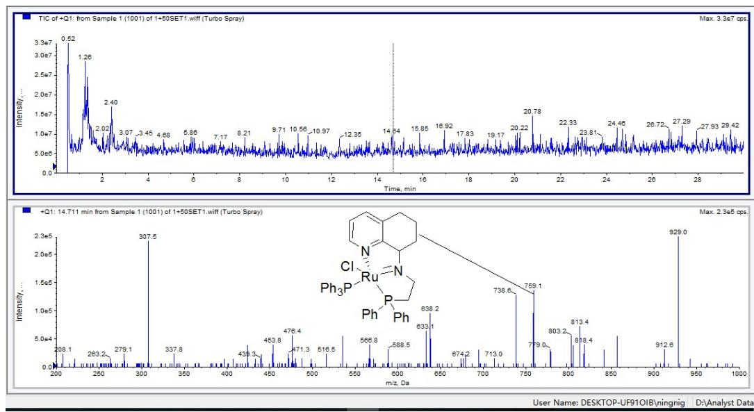
**Figure S2.** ESI mass spectra of **C** and benzyl alcohol in the presence of *t*-BuOK (1 eq.) in  $\text{CDCl}_3$  at 45 °C, recorded after 24 hours using the 3200 QTRAP 1200 infinity series instrument. Acetonitrile:water = 70:30, flow rate = 1 ml / min, electronic energy = 50eV, Q1MS scan range = 200~1000. The base peak corresponds to the intermediates  $[(\mathbf{M}-1)+1]^+$  at  $m/z$  759.1
