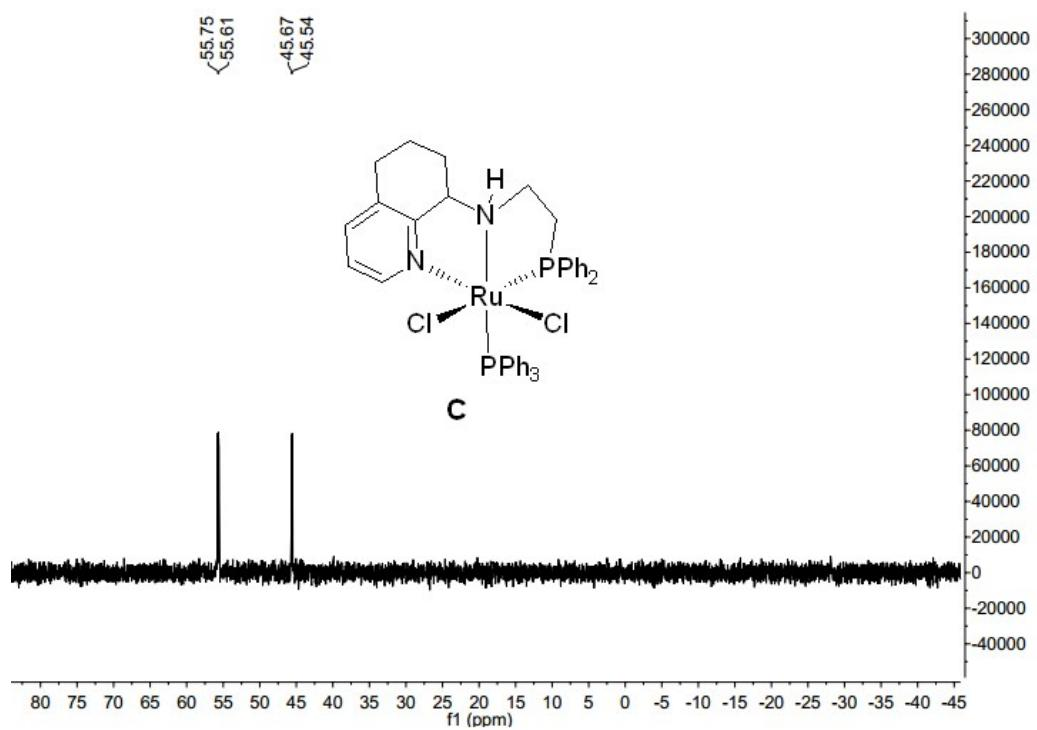
**4. The  $^{13}\text{C}\{\text{H}\}$  NMR spectrum of C in  $\text{CDCl}_3$ : spectrum recorded after 4 hours**
