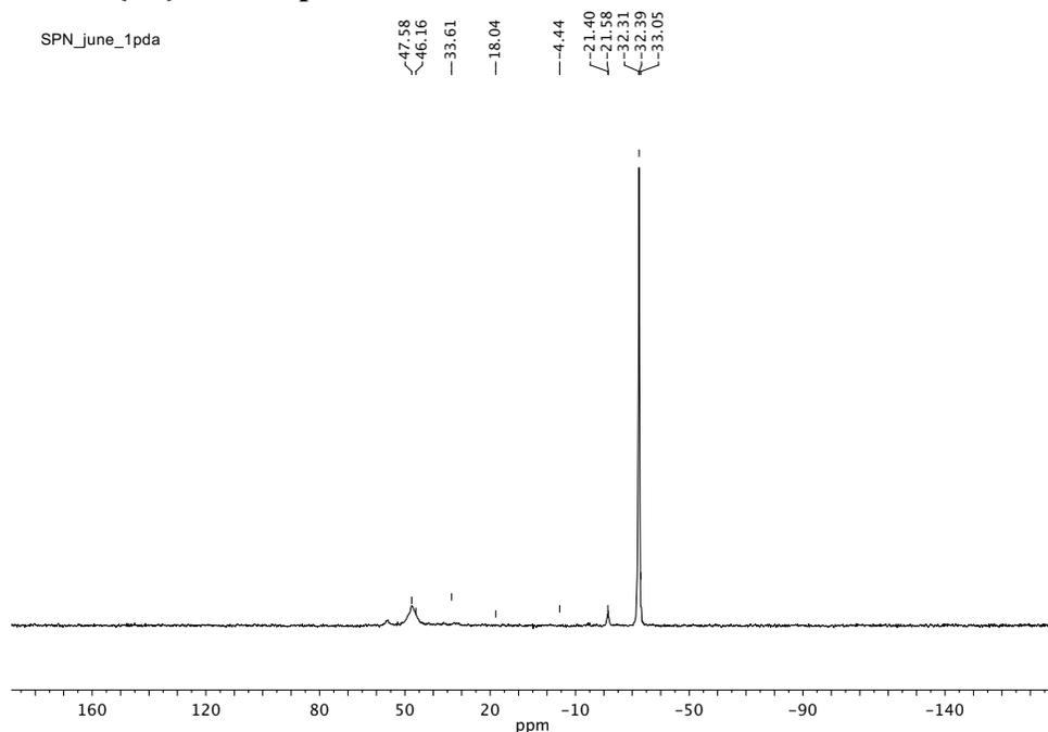
**Figure S1.** SS- $^{31}\text{P}\{^1\text{H}\}$  NMR spectrum (161.71 MHz) of **SPN1** acquired with a standard one pulse sequence. The signal at  $\delta = -32$  corresponds to tertiary phosphine sites, the broad signals at  $\delta = \text{ca. } 50$  are consistent with phosphine oxide sites.
