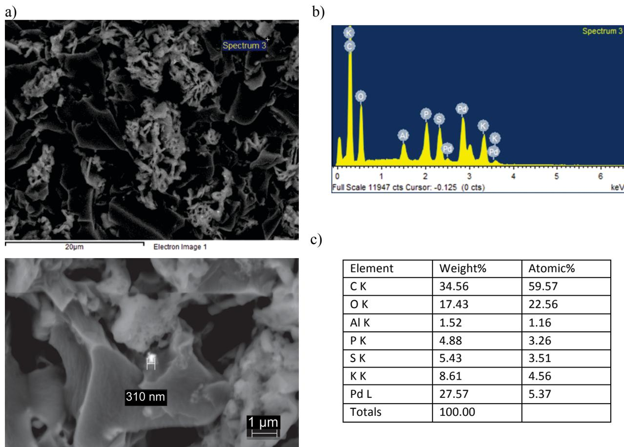
**Figure S5.** Analysis of the SPN polymer after Pd sequestration from a Suzuki coupling reaction. a) SEM images showing the only observed evidence of a nanoparticle associated with the polymer (see bright spot on the bottom image visualized using a backscatter detector); b) EDX spectra; and c) Element compositions of the potential Pd nanoparticle.
