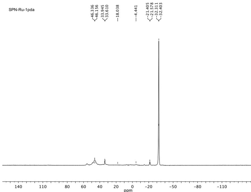
**Figure S2.** SS- $^{31}\text{P}\{^1\text{H}\}$  NMR spectrum (161.71 MHz) of **Ru-SPN1** acquired with a standard one pulse sequence. The signal at  $\delta = -32$  corresponds to tertiary phosphine sites, the broad signals at  $\delta = \text{ca. } 50$  are consistent with phosphine oxide sites.
