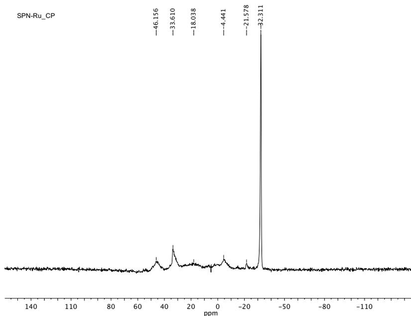
**Figure S3.** SS- $^{31}\text{P}\{^1\text{H}\}$  NMR spectrum (161.71 MHz) of **Ru-SPN1** acquired with a cross polarization pulse sequence. The signal at  $\delta = -32$  corresponds to tertiary phosphine sites, the broad signals at  $\delta = \text{ca. } 50$  are consistent with phosphine oxide sites. The broad signals in the range of 0–40 ppm are consistent with Ru-phosphine adduct formation.
