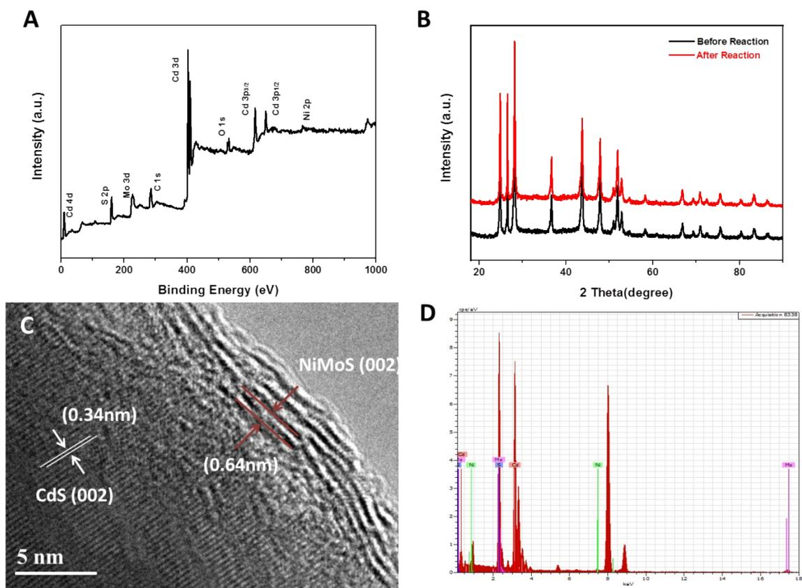
Fig. S4 XPS survey spectra of the CdS@NiMoS core-shell nanorods (A), Comparing XRD spectra before and after photocatalytic reaction (B), HRTEM image of 3wt% CdS@NiMoS nanocomposite (C), EDS spectrum of 3wt% CdS@NiMoS nanocomposite (D).
