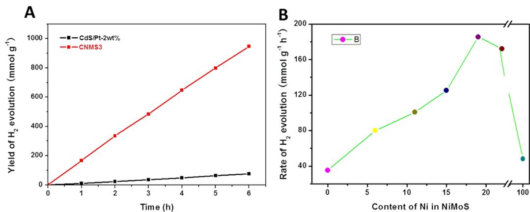
Fig. S3 Comparison of the photocatalytic H<sub>2</sub> evolution activity of different samples (A), and the photocatalytic H<sub>2</sub> evolution of the corresponding CdS@NiMoS samples (B).
