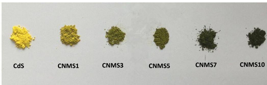
Fig. S1 Digital photographs of CdS nanorods and 1D CdS@NiMoS core-shell nanorods loading with various amounts of NiMoS.
