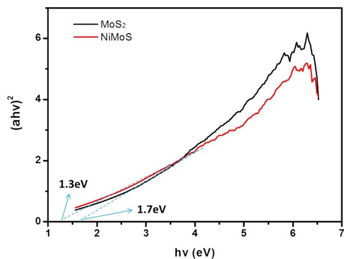
Figure S7 The band gap of NiMoS and MoS<sub>2</sub> determined from the  $(ah\nu)^2$  versus photon-energy.
