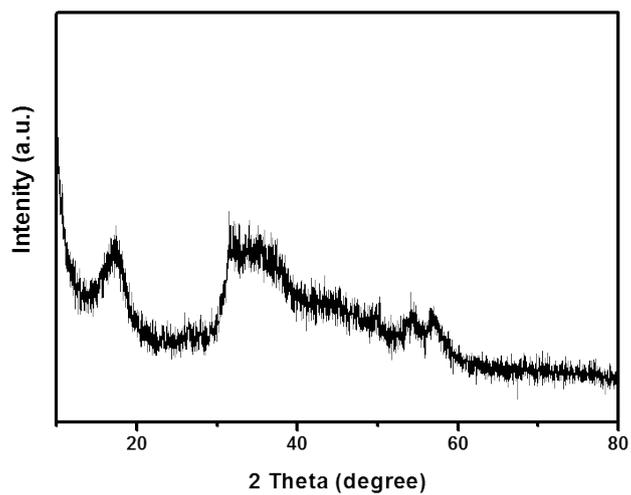
Fig. S6 X-ray diffraction pattern for NiMoS.
