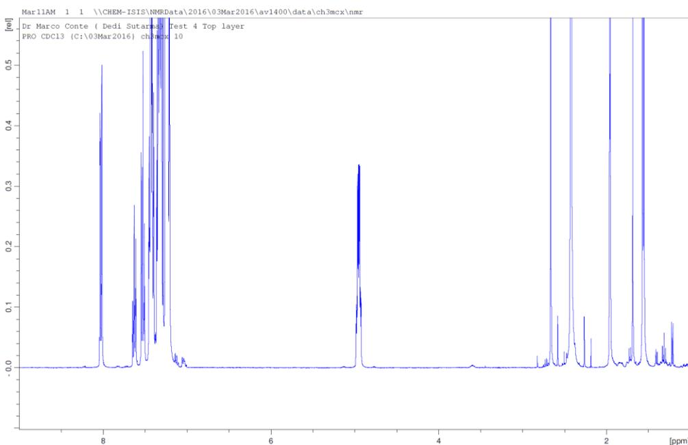
**Fig. S26** Representative <sup>1</sup>H NMR for the oxidation of 1-phenylethanol using Rh-PI/CB in water/toluene, volume ratio 2:1, M:S = 1:100, T = 100 °C, P = atmospheric pressure and in the presence of base, NaOH (base to alcohol molar ratio 1:10).
