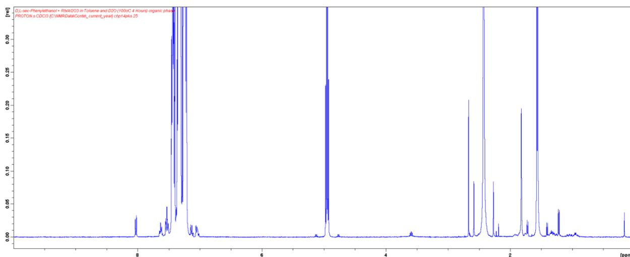
**Fig. S23** Representative  $^1\text{H}$  NMR for the oxidation of 1-phenylethanol using  $\text{Rh}/\text{Al}_2\text{O}_3$  in  $\text{D}_2\text{O}/\text{toluene}$ , volume ratio 2:1, M:S = 1:100,  $T = 100\text{ }^\circ\text{C}$ ,  $P = \text{atmospheric pressure}$ .
