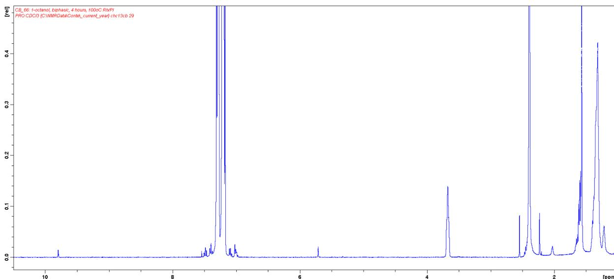
**Fig. S33** Representative  $^1\text{H}$  NMR for the oxidation of 1-octanol using Rh-PI in water/toluene, volume ratio 2:1, M:S = 1:100, T = 100  $^\circ\text{C}$ , P = atmospheric pressure of air t = 4 h.
