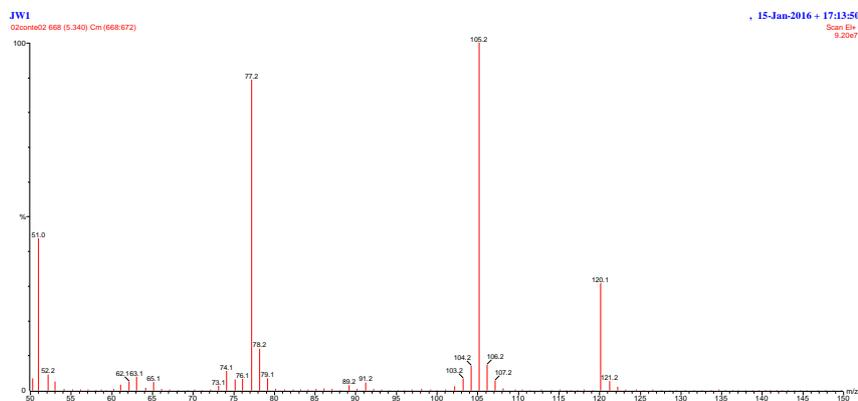
**Fig. S4** Mass spectrometry for acetophenone. Mass of molecular ion 120 Da. Fragmentation pattern m/z: 120 (molecular ion), 105 (loss of methyl  $\text{CH}_3$ ), 104 (loss of water); m/z 77 ( $\text{C}_6\text{H}_5^+$ ), m/z 51 ( $\text{C}_4\text{H}_3^+$ ).
