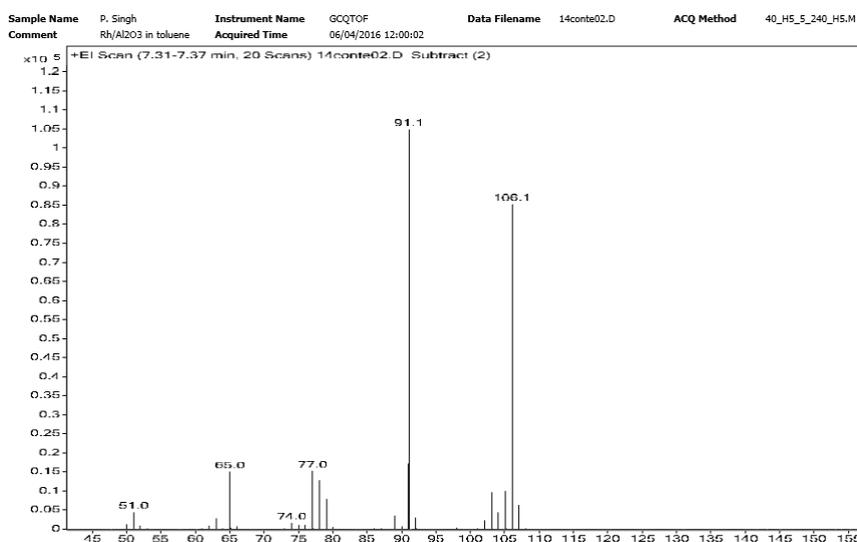
**Fig. S6** Mass spectrometry for ethylbenzene, mass of molecular ion 106 Da. Fragmentation pattern  $m/z$ : 106 (molecular ion), 91 (loss of 2 H) 107 ( $C_7H_7^+$ , loss of methyl  $CH_3$ ),  $m/z$  77 ( $C_6H_5^+$ ),  $m/z$  65 ( $C_5H_5^+$ ),  $m/z$  51 ( $C_4H_3^+$ ).
