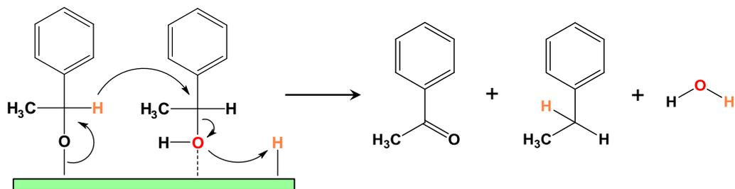
**Scheme S2** One of the accepted reaction mechanisms for the disproportionation reaction of an alcohol to a ketone and an alkane. A pre-adsorption of an alcohol molecule is needed to allow hydride transfer over the catalyst surface. A concerted mechanism would then occur, with formation of a ketone, and subsequent further hydride transfer with formation of an alkane and elimination of a water molecule.<sup>S4</sup>
