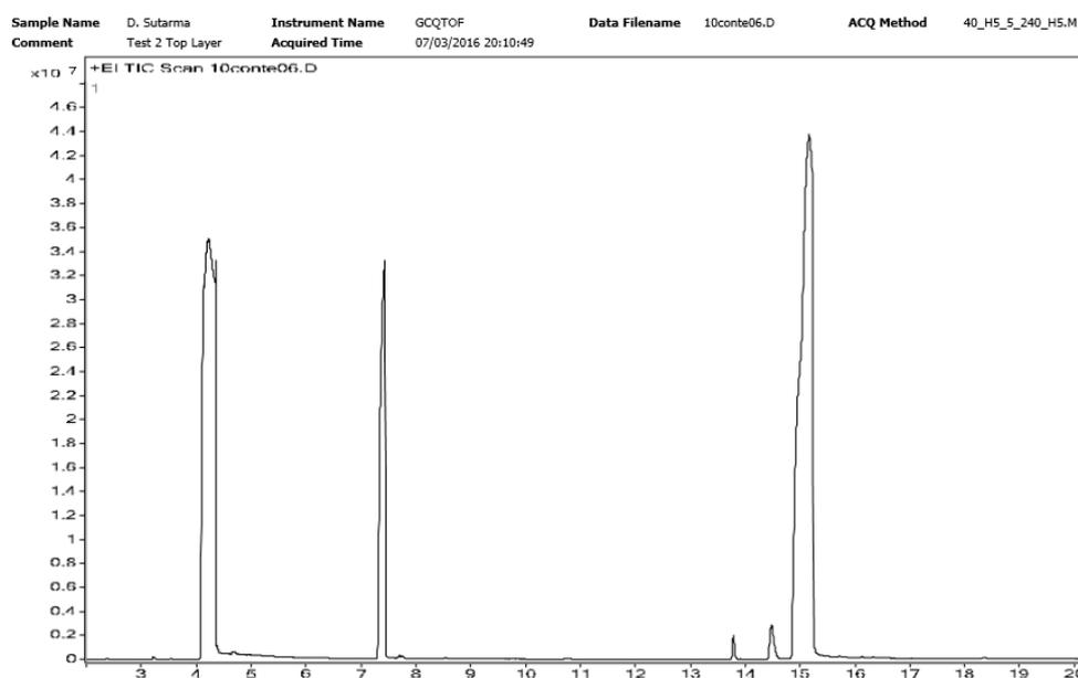
**Fig. S15** Representative GC/MS (chromatogram part) for the oxidation of 1-phenylethanol using Rh-PI/CB in water/toluene, volume ratio 2:1, M:S = 1:100, T = 100 °C, P = atmospheric pressure of air.
