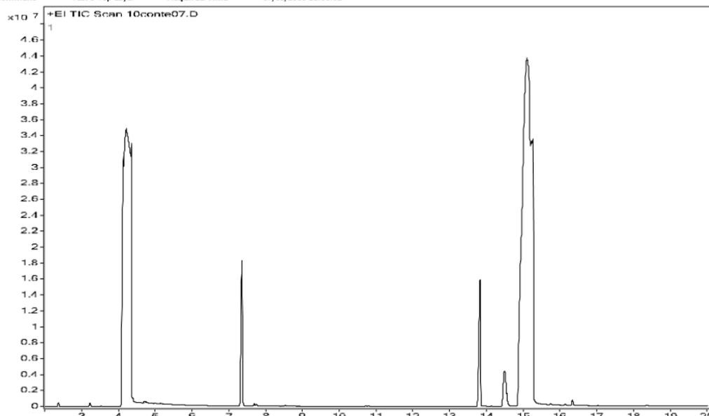
**Fig. S25** Representative GC/MS (chromatogram part) for the oxidation of 1-phenylethanol using Rh/Al<sub>2</sub>O<sub>3</sub> in water/toluene, volume ratio 2:1, M:S = 1:100, T = 100 °C, P = atmospheric pressure and in the presence of base, NaOH (base to alcohol molar ratio 1:10).
