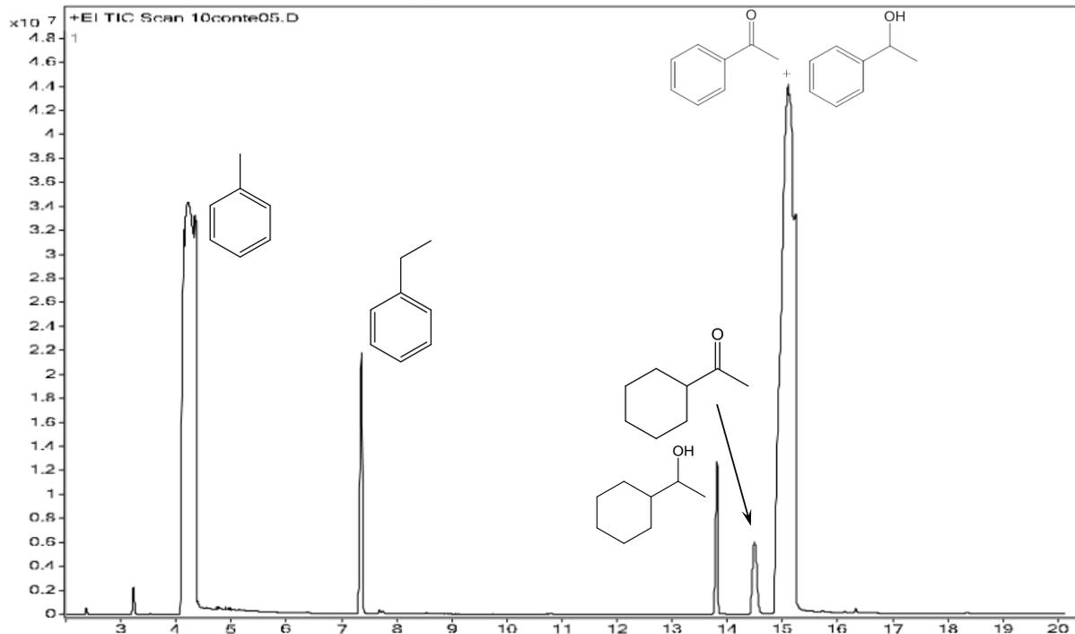
**Fig. S13** Representative GC/MS (chromatogram part) for the oxidation of 1-phenylethanol using Rh/ $\text{Al}_2\text{O}_3$  in water/toluene, volume ratio 2:1, M:S = 1:100, T = 100 °C, P = atmospheric pressure of air.
