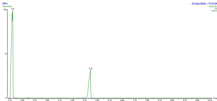
**Fig. S2** Gas chromatogram for the reaction mixture of Fig. S1. Peak at 2.21 min toluene, peak at 5.32 min: 1-phenylethanol + acetophenone (shoulder).
