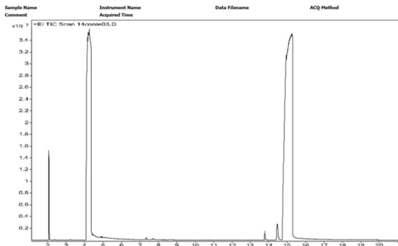
**Fig. S8** Representative GC/MS (chromatogram part) of 1-phenylethanol, starting material, in toluene. With enhanced resolution of the species (chromatographic method 2).
