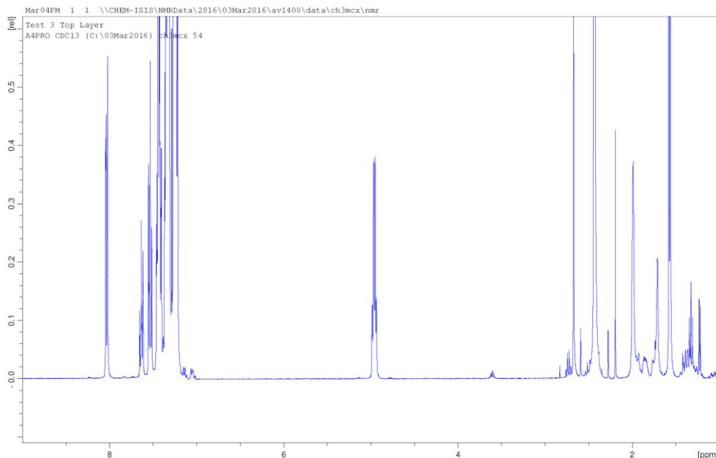
**Fig. S24** Representative  $^1\text{H}$  NMR for the oxidation of 1-phenylethanol using  $\text{Rh}/\text{Al}_2\text{O}_3$  in water/toluene, volume ratio 2:1, M:S = 1:100, T = 100 °C, P = atmospheric pressure and in the presence of base, NaOH (base to alcohol molar ratio 1:10).
