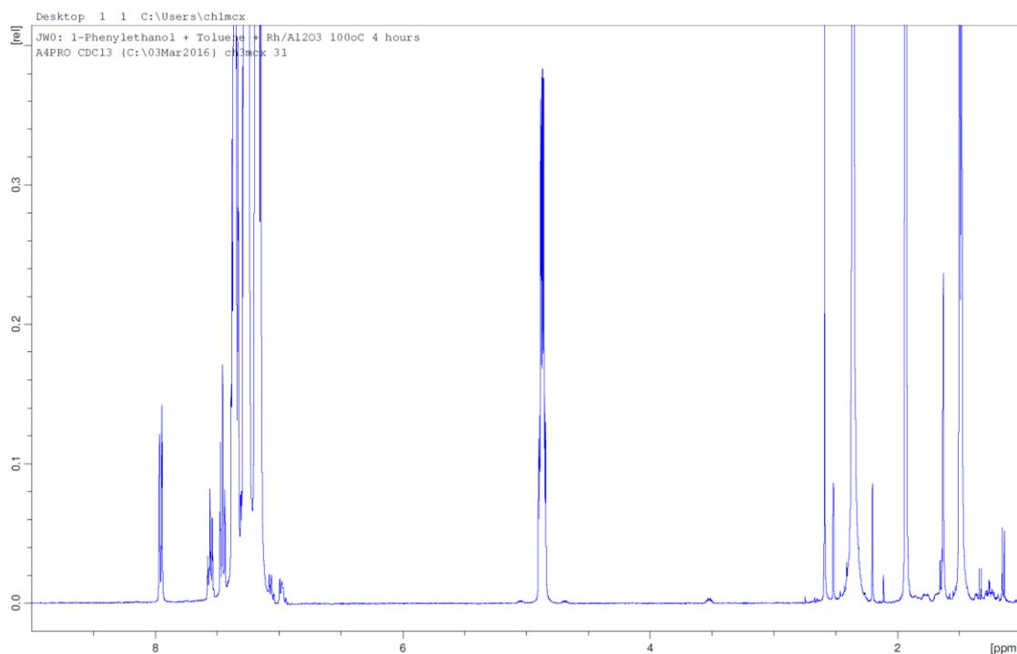
**Fig. S1** Representative  $^1\text{H}$  NMR for a catalytic test of 1-phenylethanol in toluene using  $\text{Rh}/\text{Al}_2\text{O}_3$ . M:S 1:100,  $T = 100\text{ }^\circ\text{C}$ ,  $P = \text{atmospheric pressure}$ .
