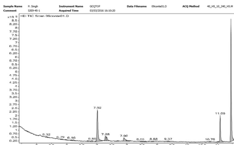
**Fig. S5** Representative chromatogram's details for the determination of impurities in the reaction mixture of Rh/Al<sub>2</sub>O<sub>3</sub> and 1-phenylethanol in toluene. From left to right: Peak at 7.2 min: ethylbenzene Peaks at 7.28 and 7.90; xylenes Peaks at 11.09 and 11.8 min: 1-cyclohexyl ethanol and cyclohexyl methyl ketone.
