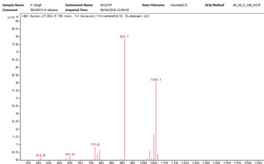
**Fig. S7** Mass spectrometry for *o*-xylene, mass of molecular ion 106 Da. Fragmentation pattern: m/z 106 (molecular ion), m/z 91 (loss of 2 H) m/z 107 ( $C_7H_7^+$ , loss of methyl  $CH_3$ ), m/z 77 ( $C_6H_5^+$ ), m/z 65 ( $C_5H_5^+$ ), m/z 51 ( $C_4H_3^+$ ).
