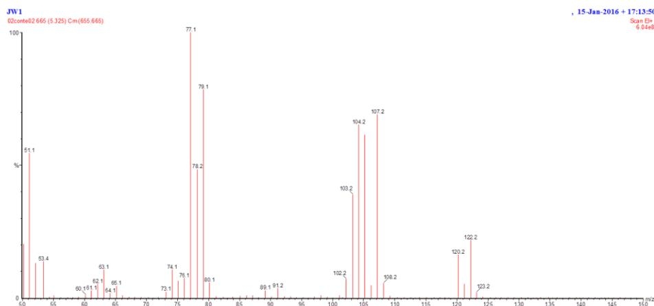
**Fig. S3** Mass spectrometry for 1-phenylethanol. Mass of molecular ion 122 Da. Fragmentation pattern m/z: 122 (molecular ion), 120 (loss of 2 H) 107 (loss of methyl  $\text{CH}_3$ ), 104 (loss of water); m/z 79 ( $\text{C}_6\text{H}_7^+$ ), m/z 77 ( $\text{C}_6\text{H}_5^+$ ), m/z 51 ( $\text{C}_4\text{H}_3^+$ ).
