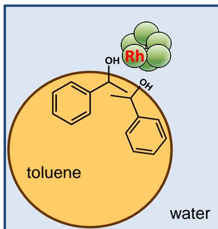
**Fig. S20** Possible enhancement of a disproportionation route in agreement with scheme S2. In this case the toluene droplet would promote the formation of a pre-oriented pair of alcohols that could favour the disproportionation pathway and the formation of ethylbenzene (and a ketone) above the catalyst surface.
