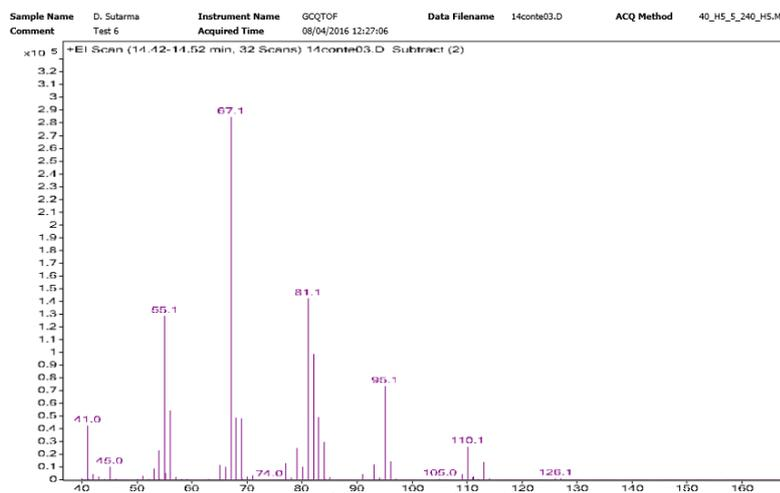
**Fig. S10** Mass spectrometry for 1-cyclohexyl ethanol. Mass of molecular ion 128 Da. Fragmentation pattern: m/z 128 (molecular ion), m/z 126 (loss of 2 H), m/z 110 (loss of H<sub>2</sub>O from molecular ion), m/z 95 (C<sub>6</sub>H<sub>7</sub>O<sup>+</sup>), m/z 81 (loss of CH<sub>2</sub>), m/z 67 (C<sub>5</sub>H<sub>7</sub><sup>+</sup>), m/z 55 (C<sub>4</sub>H<sub>7</sub><sup>+</sup>) m/z 43 (C<sub>4</sub>H<sub>7</sub><sup>+</sup> or CH<sub>3</sub>CO<sup>+</sup>).
