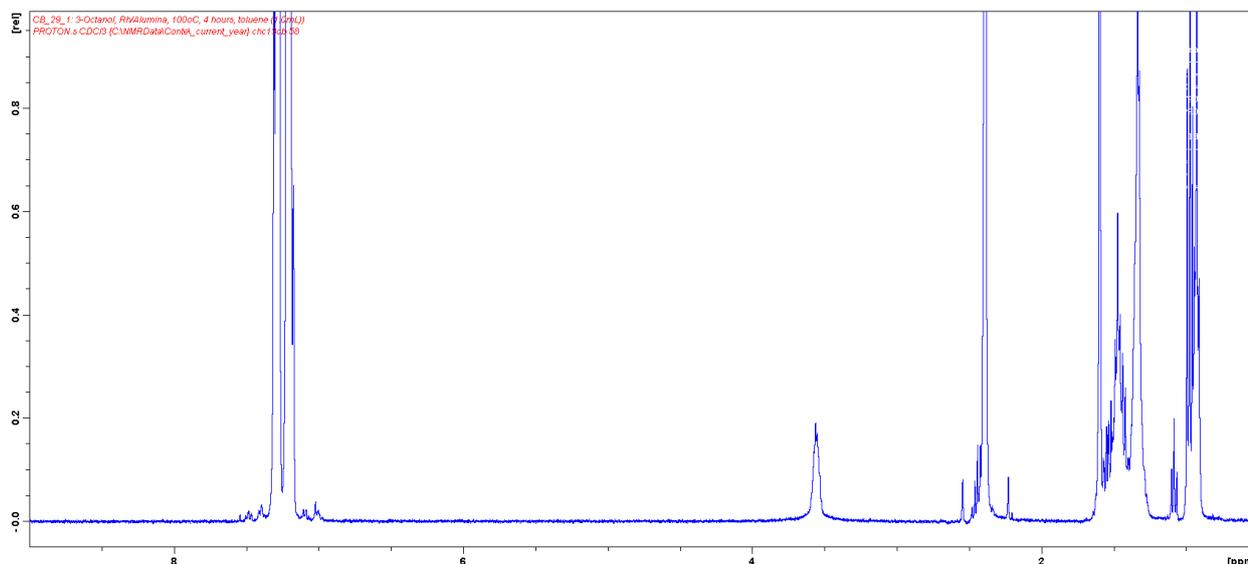
**Fig. S34** Representative  $^1\text{H}$  NMR for the oxidation of 3-octanol using  $\text{Rh}/\text{Al}_2\text{O}_3$  in toluene, M:S = 1:100, T = 100 °C, P = atmospheric pressure of air, t = 4h.
