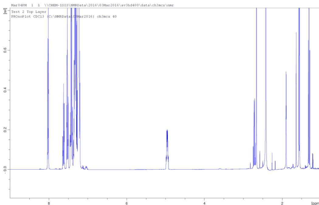
**Fig. S14** Representative  $^1\text{H}$  NMR for the oxidation of 1-phenylethanol using Rh-PI/CB in water/toluene, volume ratio 2:1, M:S = 1:100, T = 100 °C, P = atmospheric pressure.
