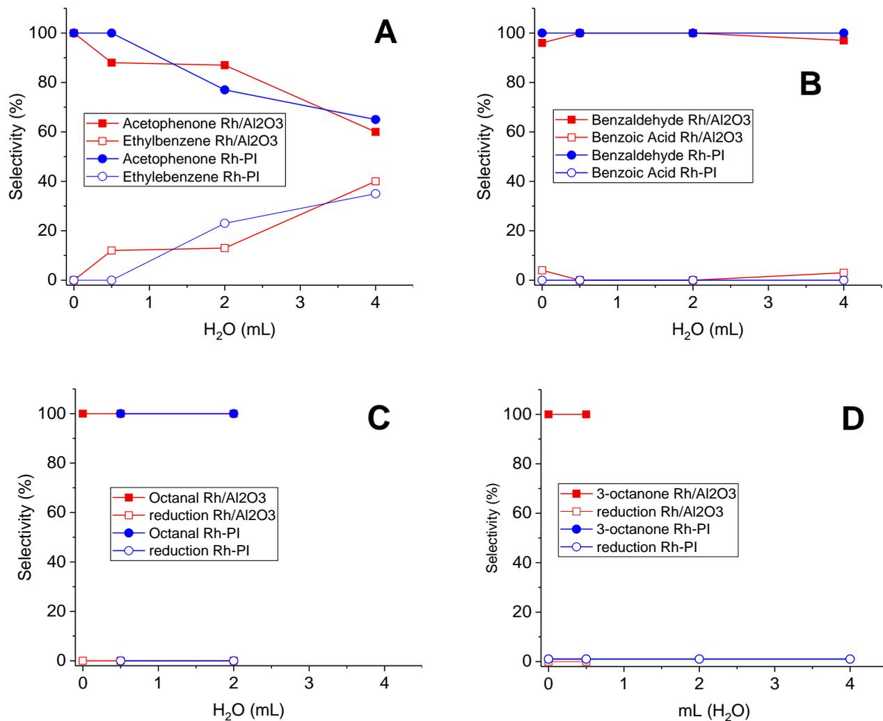
**Fig. S29** Selectivity trends for Rh/Al<sub>2</sub>O<sub>3</sub> and Rh-PI per different amount of water added to 1 mL of toluene in the oxidation of the alcohols: (A) 1-phenylethanol, (B) benzyl alcohol, (C) 1-octanol and (D) 3-octanol. Reaction conditions: T = 100 °C, P = atmospheric pressure of air, reaction time 4 h.
