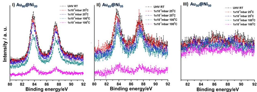
Figure S8: Au 4f spectra obtained for (I)  $\text{Au}_{80}@\text{Ni}_{20}$ , (II)  $\text{Au}_{65}@\text{Ni}_{35}$  and (III)  $\text{Au}_{50}@\text{Ni}_{50}$  under oxygen atmosphere at various pressure and temperature conditions.
