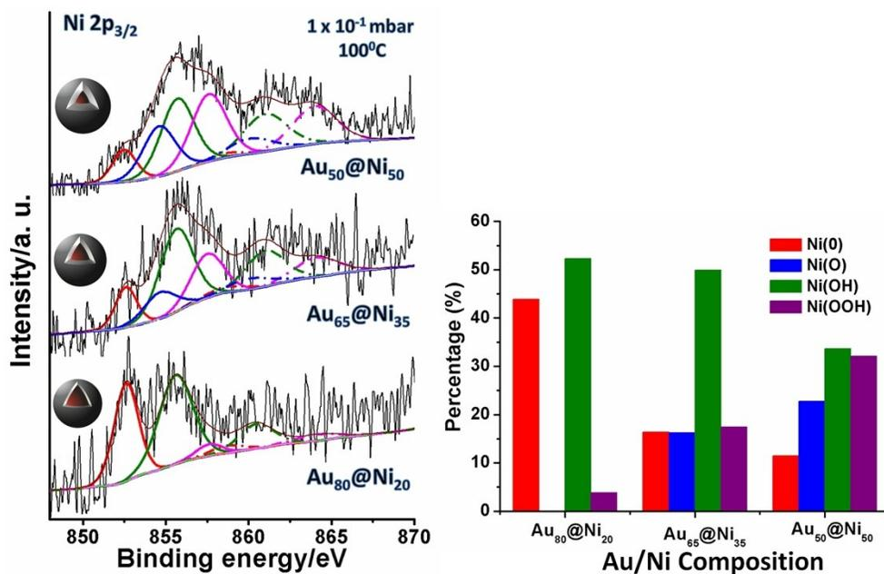
Figure S7: Ni 2p<sub>3/2</sub> spectra and its deconvolution obtained for Au<sub>80</sub>@Ni<sub>20</sub>, Au<sub>65</sub>@Ni<sub>35</sub> and Au<sub>50</sub>@Ni<sub>50</sub> core-shell nanoparticles at 0.1 mbar oxygen pressure and 100°C. Figure b)
