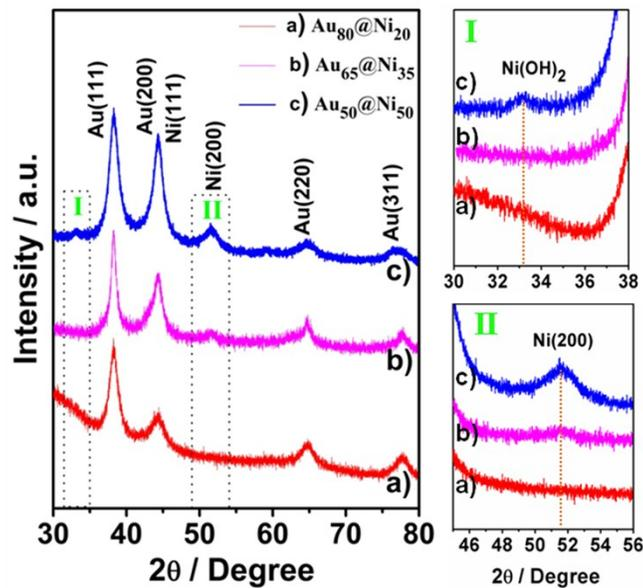
Figure S5: XRD patterns of core shell (a) Au<sub>80</sub>@Ni<sub>20</sub>, (b) Au<sub>65</sub>@Ni<sub>35</sub> and (c) Au<sub>50</sub>@Ni<sub>50</sub> nanoparticles. (I & II) are the zoomed images of the area marked in the dotted boxes and the dotted lines corresponds to Ni(OH)<sub>2</sub> and metallic Ni features respectively.
