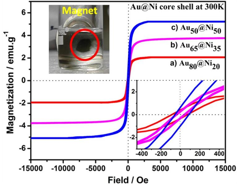
Figure S4: Hysteresis loops of (a)  $\text{Au}_{80}\text{@Ni}_{20}$  (b)  $\text{Au}_{65}\text{@Ni}_{35}$  and (c)  $\text{Au}_{50}\text{@Ni}_{50}$  nanoparticles obtained at room temperature. Inset (down) shows the hysteresis width near to the zero magnetic field. Digital photograph shows the ferromagnetic character of  $\text{Au@Ni}$  core shell nanoparticles.
