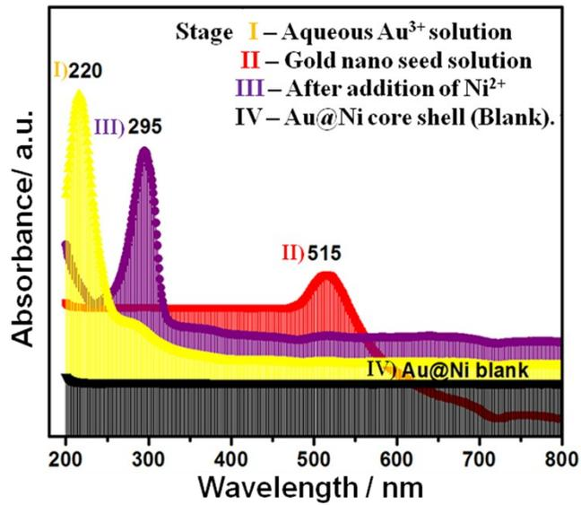
Figure S1: UV-Vis spectra recorded at each stage of synthesis of Au@Ni core-shell nanoparticles.
