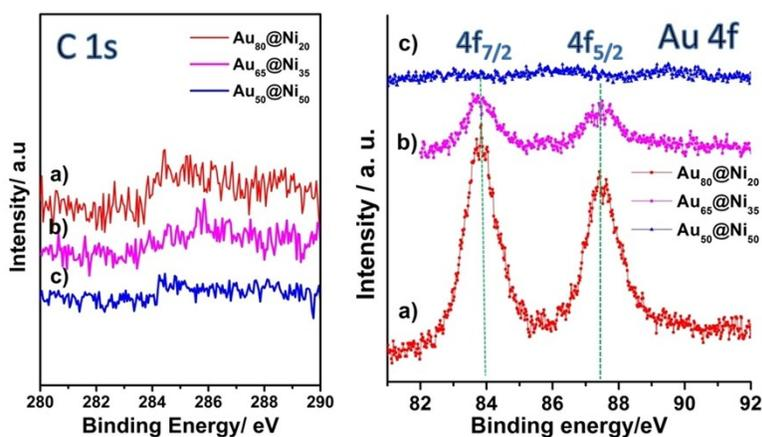
Figure S3: C 1s and Au 4f spectra of the as synthesized (a) Au<sub>80</sub>@Ni<sub>20</sub> (b) Au<sub>65</sub>@Ni<sub>35</sub> and (c) Au<sub>50</sub>@Ni<sub>50</sub> core-shell nanoparticles at UHV-RT conditions.
