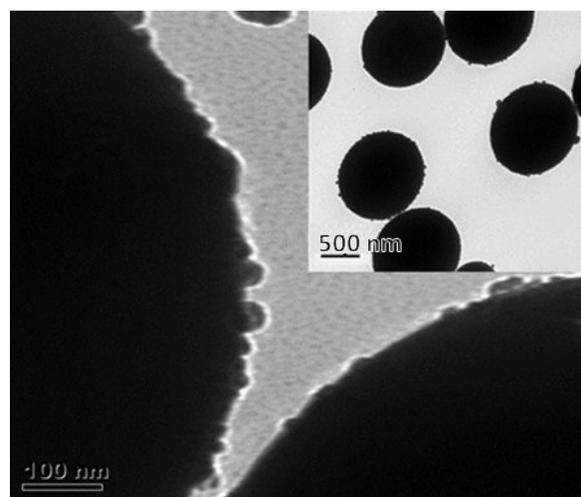
*Figure S3: TEM micrographs of spent Co<sub>3</sub>O<sub>4</sub>/SiO<sub>2</sub> model catalysts after exposure to CO-PROX reaction conditions at maximum temperature of 450 °C.*
