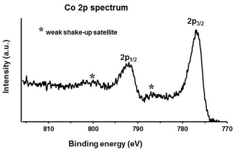
Figure S6: XPS profiles of wide spectrum, Co 2p in the Co<sub>3</sub>O<sub>4</sub>/SiO<sub>2</sub> (nanocubes)
