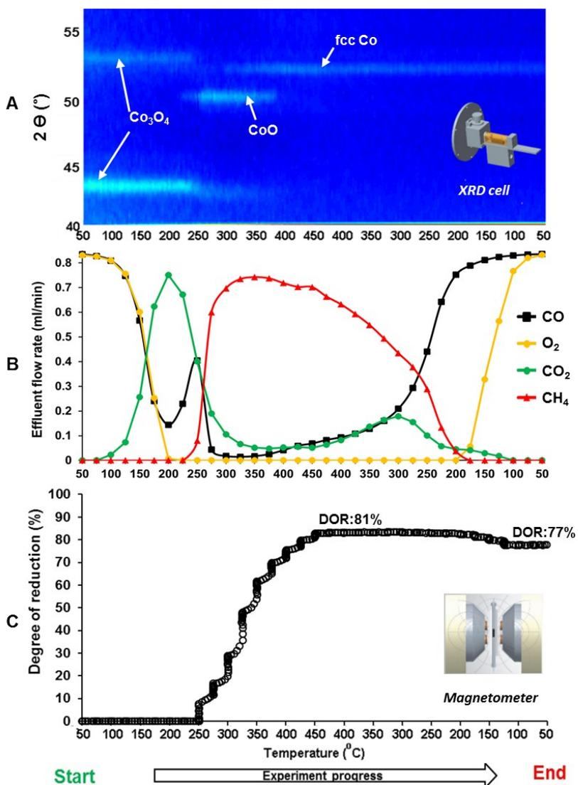
Figure S1: In situ XRD scans and degree of reduction from magnetometer measurements for nanosheets/SiO<sub>2</sub>. A: in situ XRD on top view. B: effluent flow rate of CO, CO<sub>2</sub>, CH<sub>4</sub> and O<sub>2</sub>. C: degree of reduction measured in the magnetometer. (Temperature: 450 °C, Heating rate: 50 °C to 450 °C back to 50 °C holding for 1 hr every 25 °C with a ramp rate of 1 °C/min, magnetic readings: taken at -20, 0, 20 and 0 kOe every 10 min).
