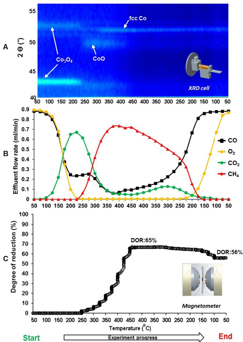
Figure S2: In situ XRD scans and degree of reduction from magnetometer measurements for nanobelts/SiO<sub>2</sub>. A: in situ XRD on top view. B: effluent flow rate of CO, CO<sub>2</sub>, CH<sub>4</sub> and O<sub>2</sub>. C: degree of reduction measured in the magnetometer. (Temperature: 450 °C, Heating rate: 50 °C to 450 °C back to 50 °C holding for 1 hr every 25 °C with a ramp rate of 1 °C/min, magnetic readings: taken at -20, 0, 20 and 0 kOe every 10 min).
