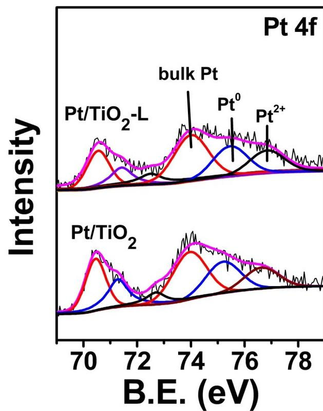
Fig. S7. Pt4f fine XPS spectra of Pt/TiO<sub>2</sub> and Pt/TiO<sub>2</sub>-L.
