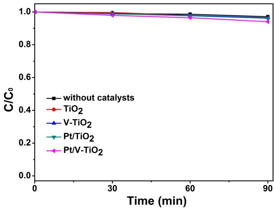
Fig. S1. The concentration variations of CO with or without catalyst in the dark.
