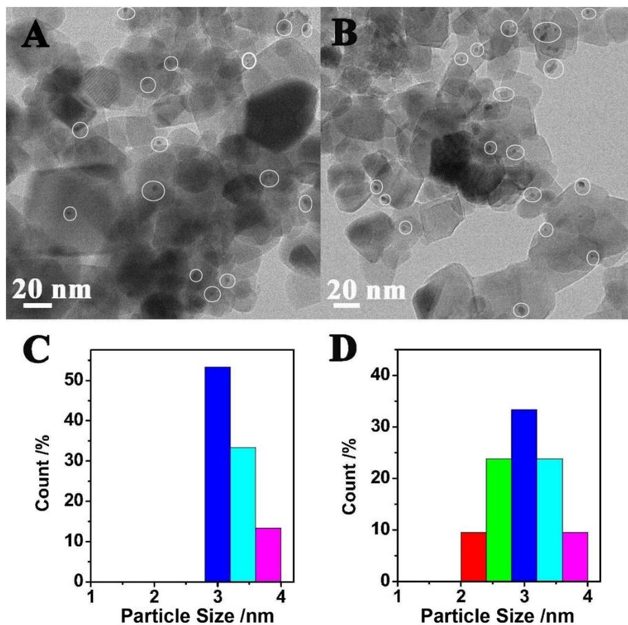
**Fig. S3.** HRTEM images of A) Pt/TiO<sub>2</sub> and B) \*Pt/TiO<sub>2</sub>-L; diameter statistics of the Pt particles for C) Pt/TiO<sub>2</sub> and D) Pt/TiO<sub>2</sub>-L. \* Pt/TiO<sub>2</sub>-L refers to the Pt/V-TiO<sub>2</sub> sample experienced 360 min photocatalytic reaction (4 cycles).
