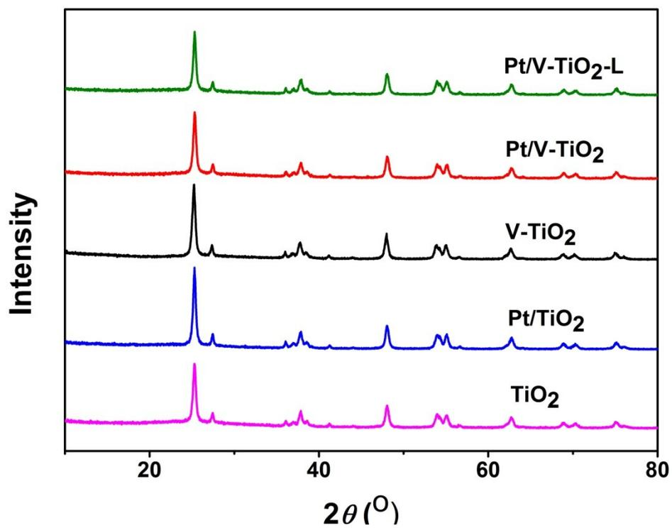
Fig. S2. XRD patterns of TiO<sub>2</sub>, Pt/TiO<sub>2</sub>, V-TiO<sub>2</sub>, Pt/V-TiO<sub>2</sub> and Pt/V-TiO<sub>2</sub>-L.
