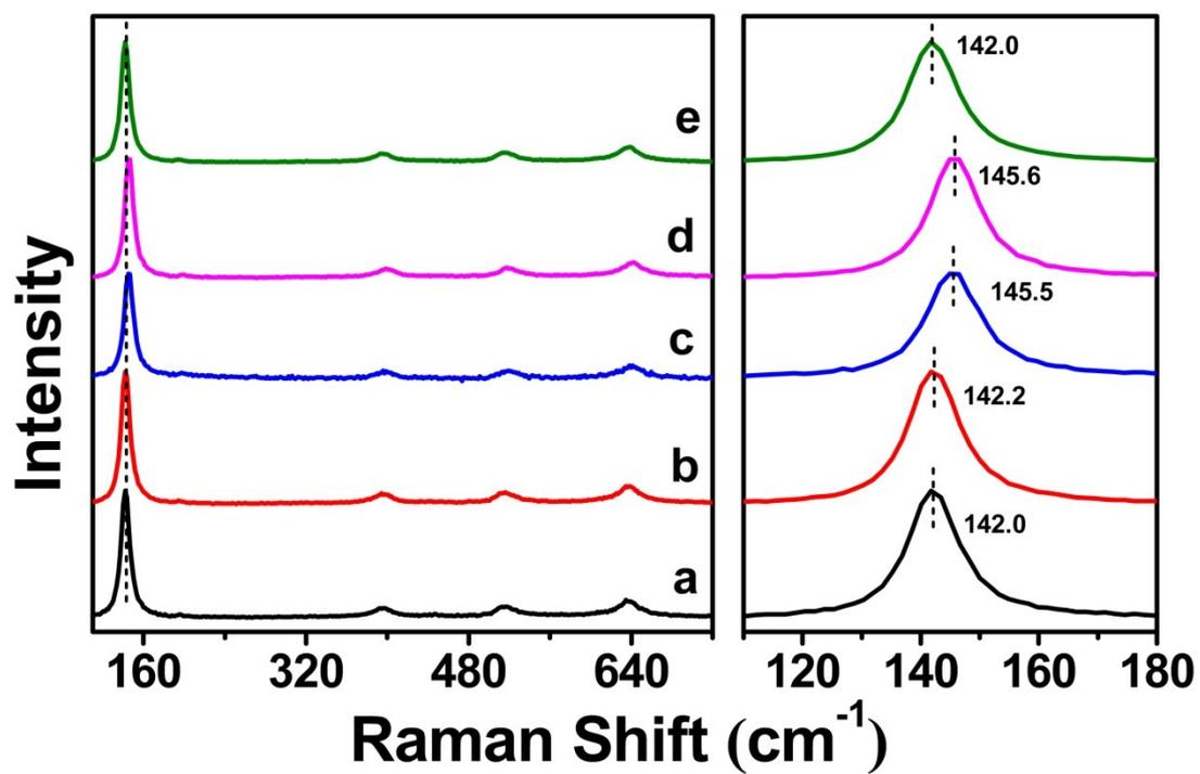
**Fig. S6.** Raman spectra of (a)  $\text{TiO}_2$ , (b)  $\text{Pt/TiO}_2$ , (c)  $\text{V-TiO}_2$ , (d)  $\text{Pt/V-TiO}_2$  and (e)  $\text{Pt/V-TiO}_2\text{-L}$
