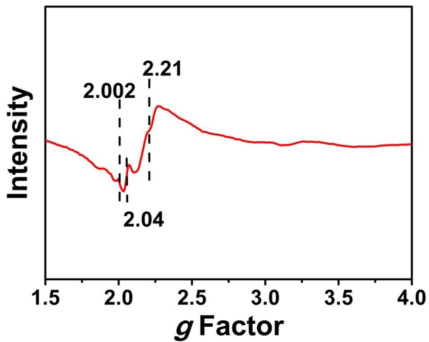
Fig. S5. EPR spectrum of Pt/V-TiO<sub>2</sub> after storing in the dark for two weeks
