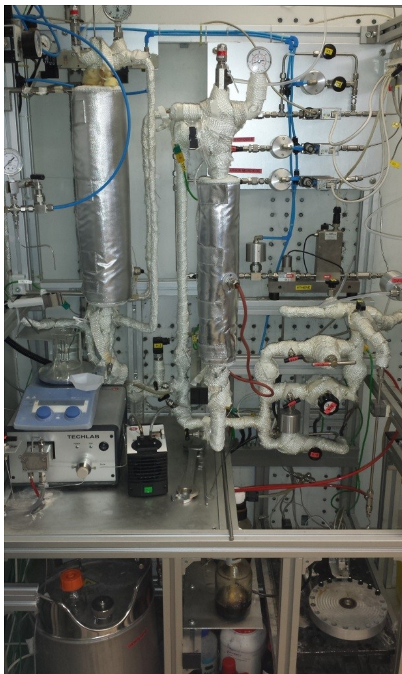
Figure S2. Photograph of the continuous gas-phase hydroformylation reactor.
