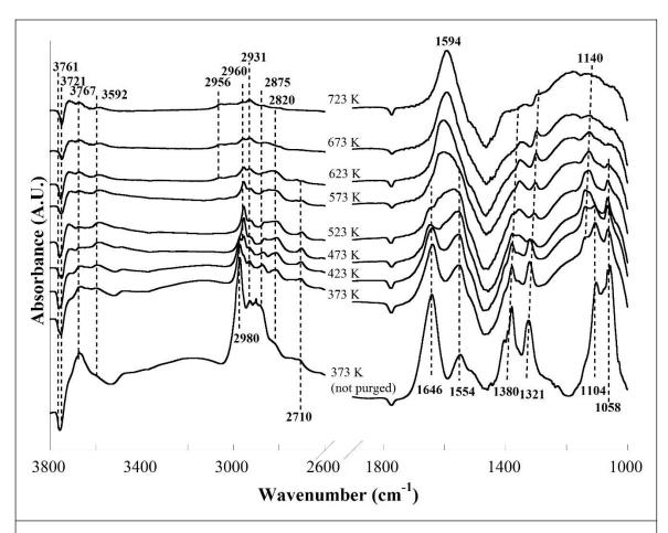
**Figure S1.** *In-situ* spectroscopy of ethanol on MgO catalyst. Ethanol was adsorbed on the sample surface and temperature ramped up from 373 to 723 K while spectra being recorded. Subtracted spectra are shown. Spectra are offset for clarity.
