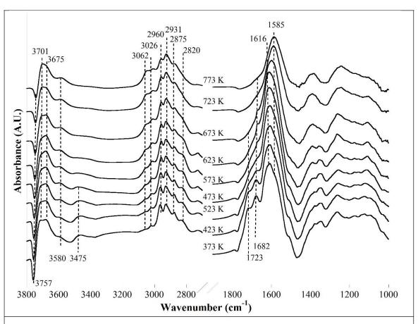
**Figure S2.** *In-situ* spectroscopy of acetaldehyde on MgO catalyst. Acetaldehyde was adsorbed on the sample surface and temperature ramped up from 373 to 723 K while spectra are being recorded. Spectra are offset for clarity.
