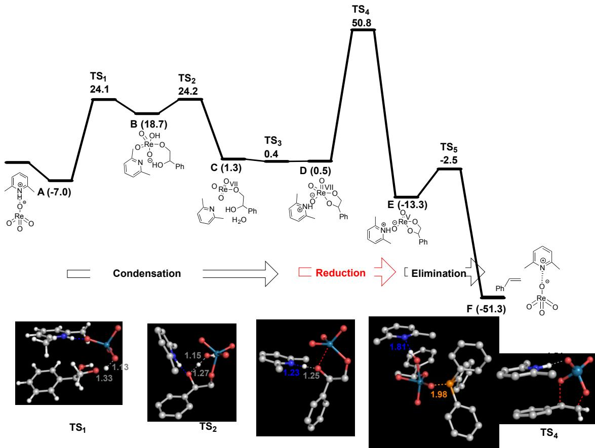
**Figure S32.** Structures and relative free energies ( $\Delta G$ , in kcal mol<sup>-1</sup>; selected distances in Å) of stationary points involved in the catalytic cycle for the DODH reaction of styrene diol by **3** proceeding via condensation, reduction and extrusion steps. Energy values were calculated at the SMD(CHCl<sub>3</sub>)B3LYP-D3(BJ)/Def2QZVP//B3LYP-D3(BJ)/6-31G+(d) level of theory relative to the separated species.)
