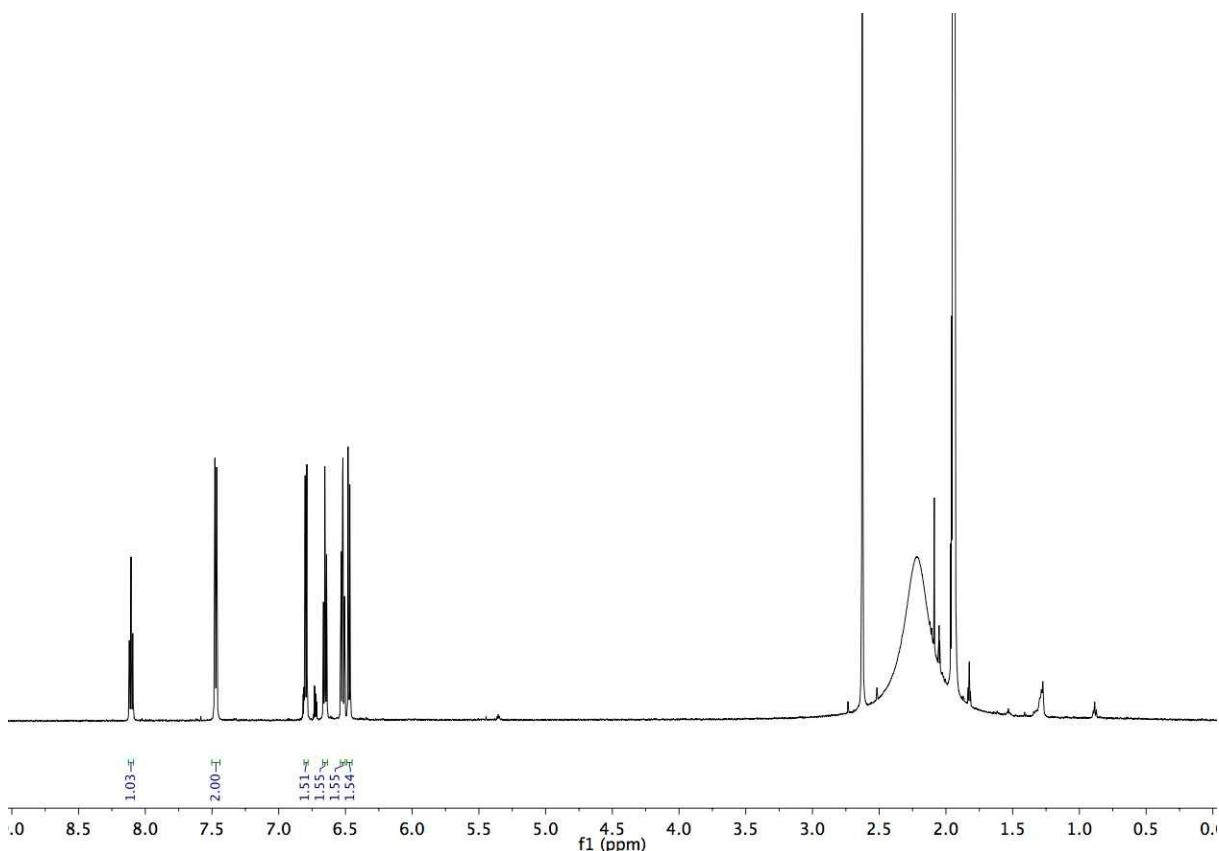
**Figure S29.**  $^1\text{H-NMR}$  of the mixture containing [2,6-dimethylpyridinium] $[\text{Re}^{\text{VII}}\text{O}_3(\text{C}_6\text{H}_4\text{O}_2)]$  and [2,6-dimethylpyridinium] $[\text{Re}^{\text{VII}}\text{O}(\text{C}_6\text{H}_4\text{O}_2)_2]$ .
