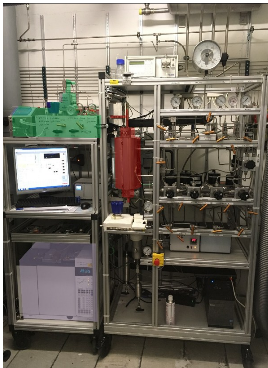
Fig. S1 Setup for HA synthesis comprising a liquid injection system (green), a reactor, a hot trap (red) and an online GC (purple).
