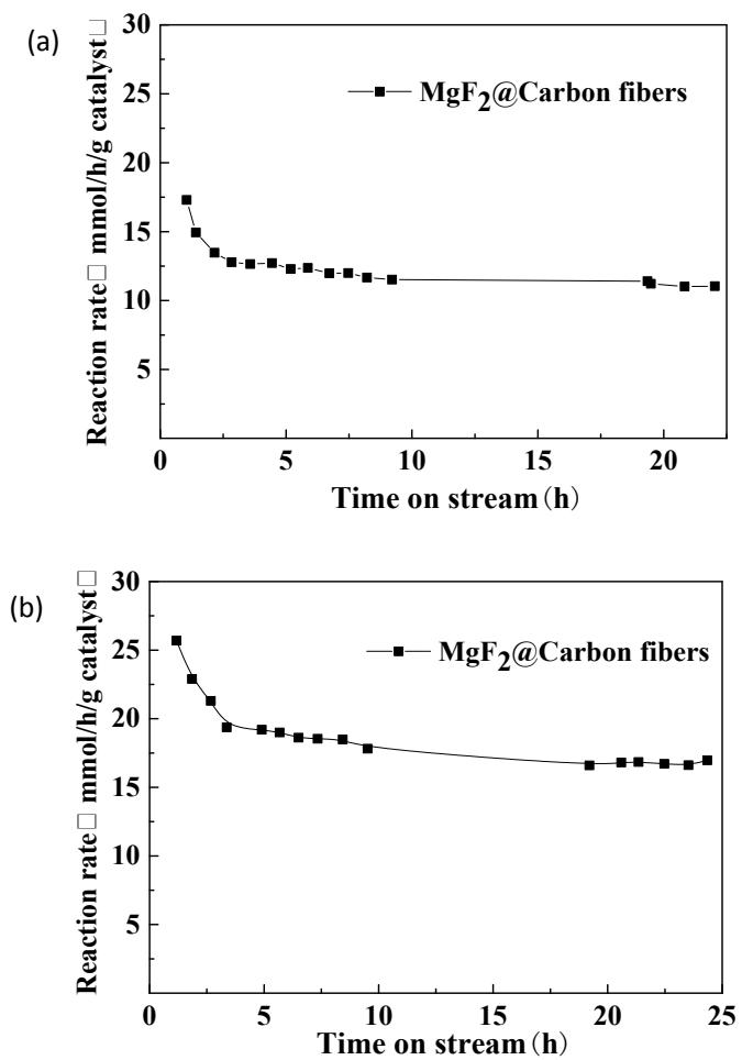
Figure S4 Dehydrofluorination of 1,1,1-trifluoroethane over nano  $\text{MgF}_2$  embedded in nanofiber at (a) 450 °C and (b) 500 °C. GHSV for 1,1,1-trifluoroethane of  $1200\text{h}^{-1}$  and diluted by equimolar  $\text{N}_2$ .
