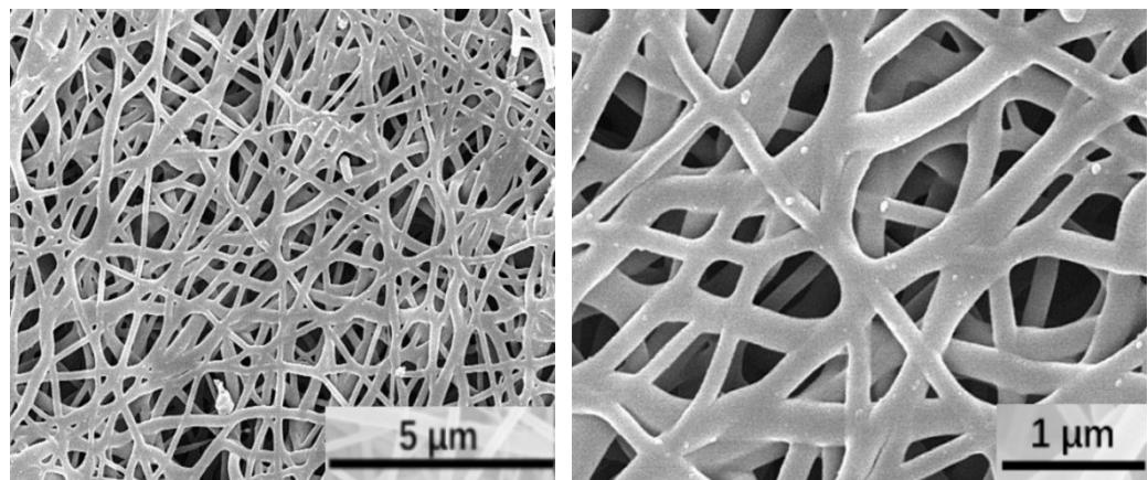
Figure S6 SEM images nano MgF<sub>2</sub> embedded in nanofiber after reaction at 450 °C.
