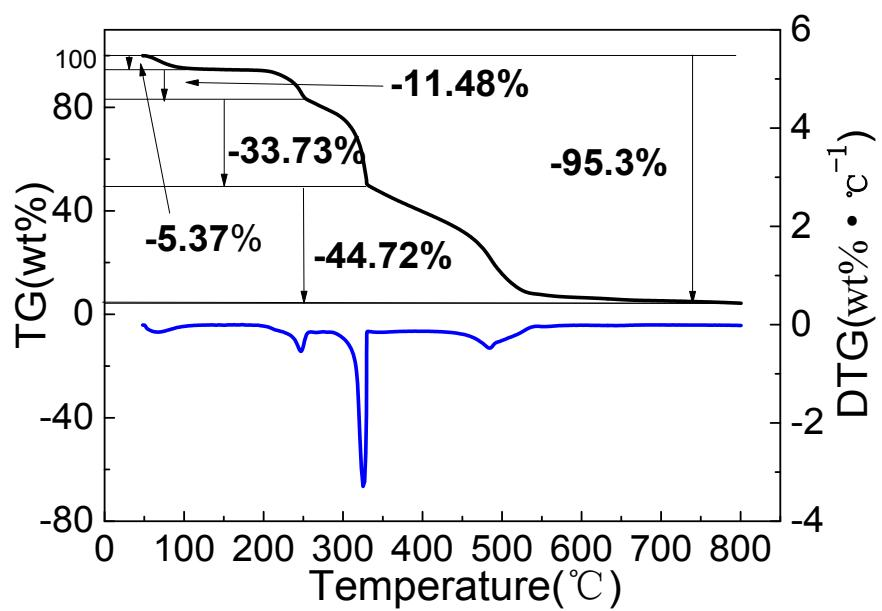
Figure S14 TG-DTG of PVP/PVDF/Mg(CH<sub>3</sub>COO)<sub>2</sub>·4H<sub>2</sub>O nanofibers with ramp rate of 10 °C/min in air atmosphere.
