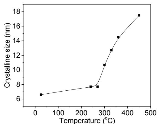
Figure S3 Crystalline size of plane (111) at temperatures between 25 °C and 500 °C for precipitated MgF<sub>2</sub>.
