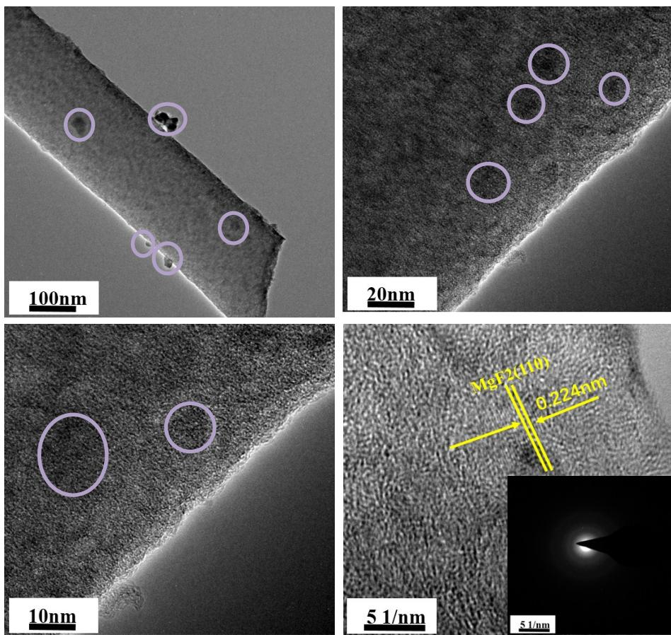
Figure S9 TEM images nano  $\text{MgF}_2$  embedded in nanofiber after reaction at 500 °C.
