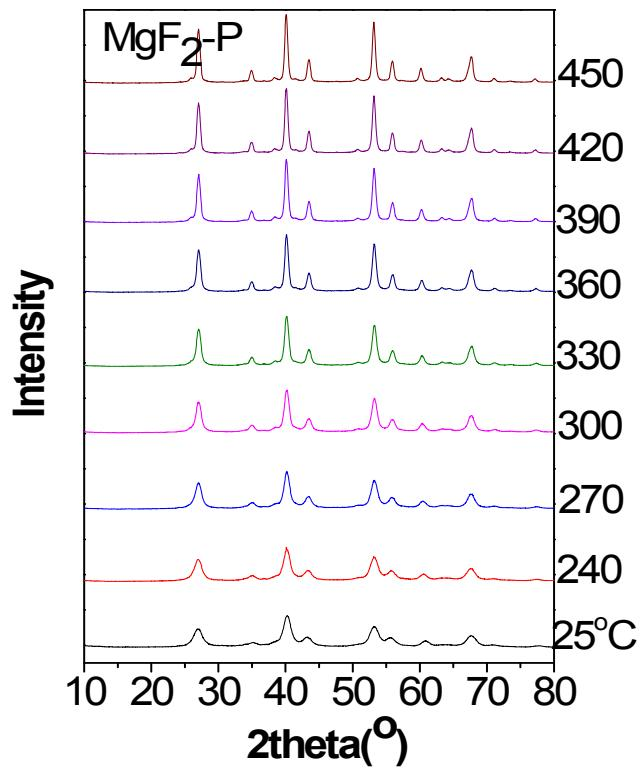
Figure S2 In situ XRD spectra of precipitated MgF<sub>2</sub> at temperatures between 25 °C and 450 °C.
