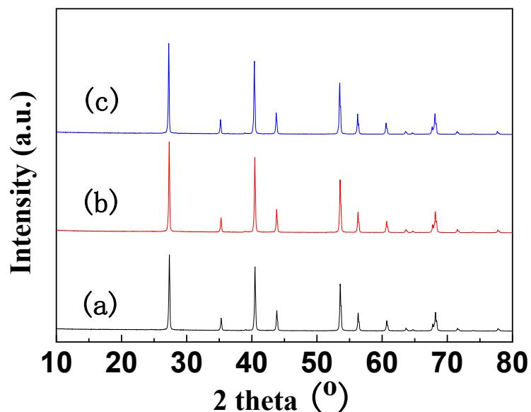
Figure S10 X-ray diffraction (XRD) patterns of precipitated  $\text{MgF}_2$  following calcination at 650 °C for 5 h. (a) before reaction, (b) spent  $\text{MgF}_2$  after reaction at 450 °C and (c) spent  $\text{MgF}_2$  after reaction at 500 °C.
