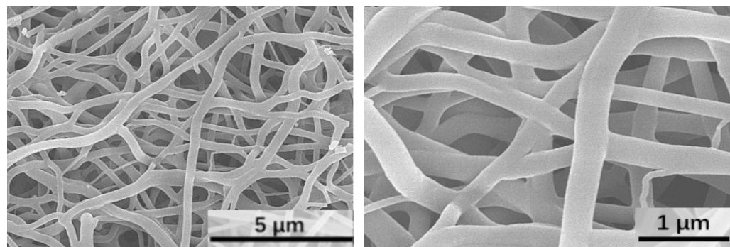
Figure S8 SEM images nano MgF<sub>2</sub> embedded in nanofiber after reaction at 500 °C.
