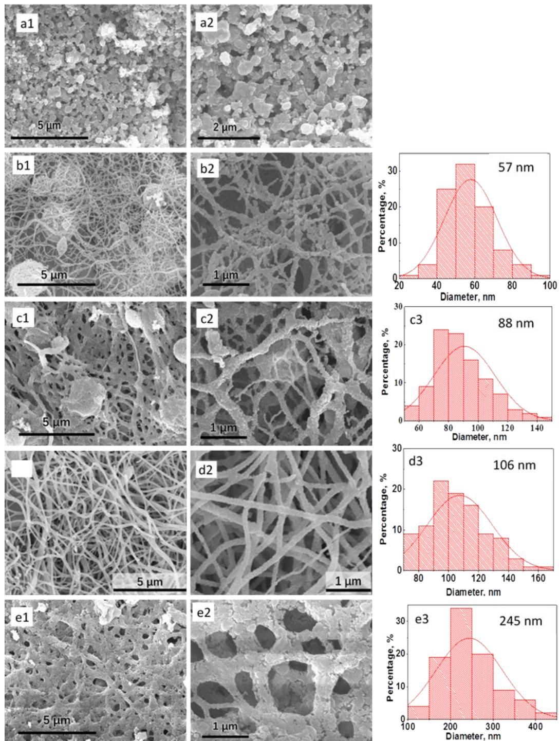
Fig. S13 Effect of PVP concentration on the Electrospun  $\text{MgF}_2$  nanofibers. SEM images and fiber diameter distribution of  $\text{MgF}_2$  with PVP concentration (a) 0 g/mL; (b) 0.05 g/mL (c) 0.07 g/mL; (d) 0.08 g/mL and (e) 0.10 g/mL in the electrospinning solution.
