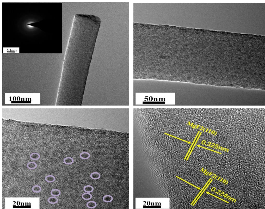
Figure S7 TEM images nano MgF<sub>2</sub> embedded in nanofiber after reaction at 450 °C.
