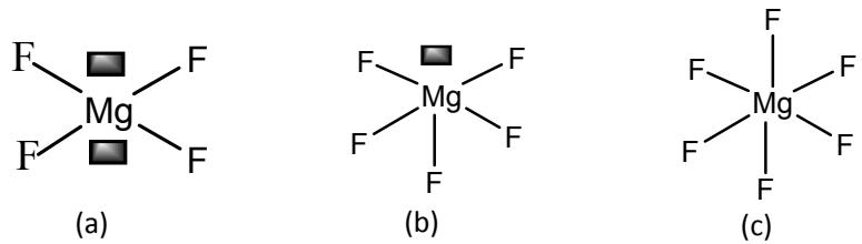
Figure S11 (a) 4-fold coordinated, (b) 5-fold coordinated and (c) 6-fold coordinated  $\text{MgF}_2$ .
