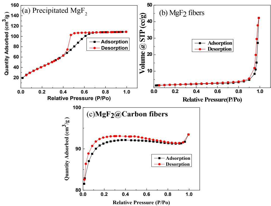
Figure S5 N<sub>2</sub> adsorption–desorption isotherms of (a) precipitated MgF<sub>2</sub>, (b) electrospun MgF<sub>2</sub> fibers and (c) nano MgF<sub>2</sub> embedded in carbon nanofiber.
