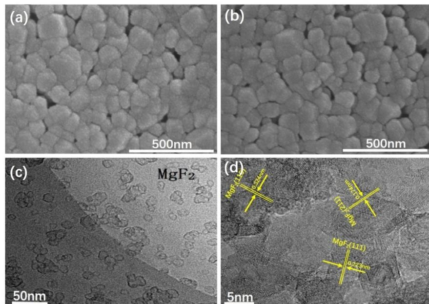
Figure S1 SEM images (a and b) and TEM images (c and d) of precipitated  $\text{MgF}_2$ .
