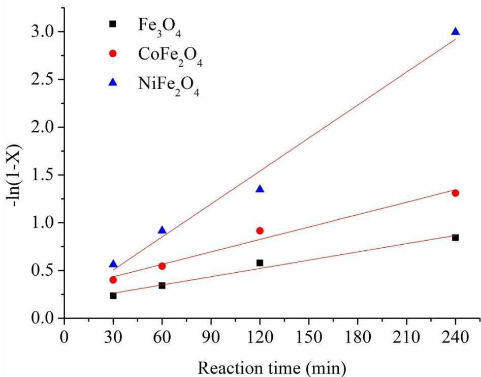
**Figure S1.**  $-\ln(1-X)$  vs. reaction time for  $\text{Fe}_3\text{O}_4$ ,  $\text{CoFe}_2\text{O}_4$  and  $\text{NiFe}_2\text{O}_4$ . Reaction conditions: FF (2 mmol), catalyst (0.06 g), 2-propanol (10 mL),  $T = 180^\circ\text{C}$ ,  $t = 0.5\text{-}4\text{ h}$ .
