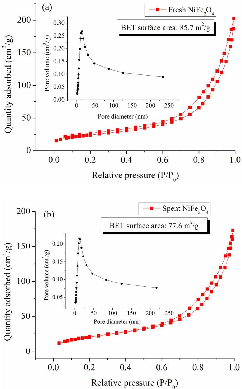
**Figure S3.**  $\text{N}_2$  adsorption-desorption isotherms and pore size distribution of fresh (a) and spent (b)  $\text{NiFe}_2\text{O}_4$  catalyst.
