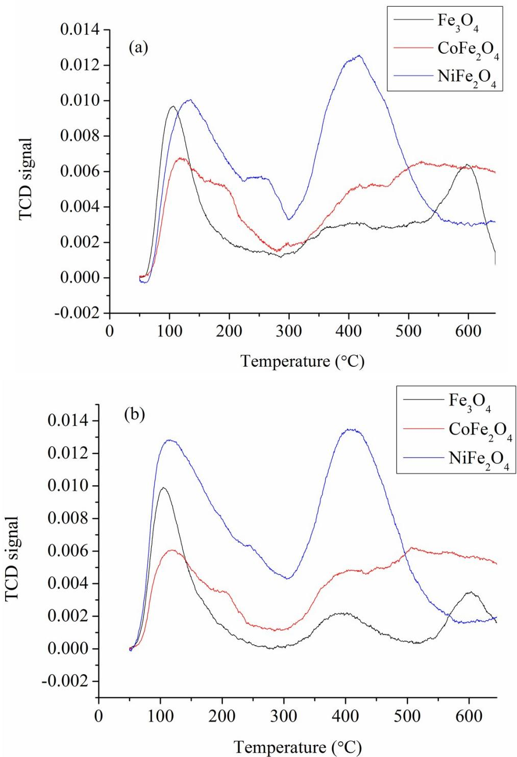
**Figure S2.** NH<sub>3</sub>-TPD (a) and CO<sub>2</sub>-TPD (b) profile of different nanoparticle ferrite catalysts.
