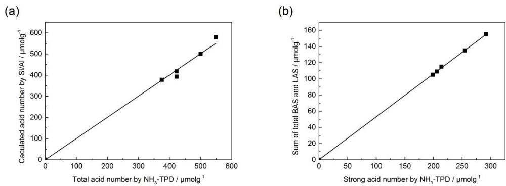
Fig. S7. Linear correlation of acid sites by different methods
