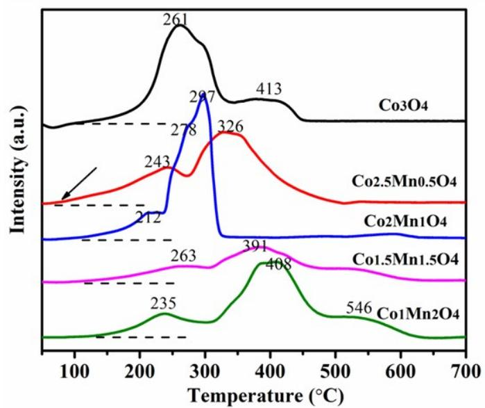
Fig. S5 H<sub>2</sub>-TPR profiles of the Co<sub>3-x</sub>Mn<sub>x</sub>O<sub>4</sub> NAs samples.
