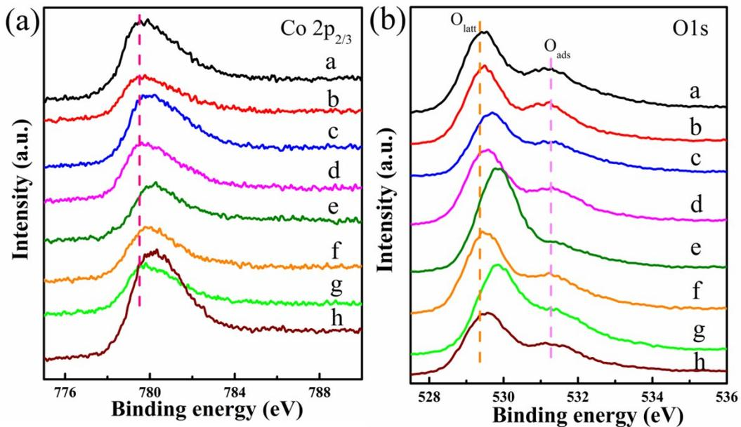
**Fig. S1** XPS spectra of the  $M\text{Co}_2\text{O}_4$  NAs samples supported on Ni foam: (a)  $\text{Co } 2p_{3/2}$ , (b)  $\text{O } 1s$ ; insert a-h correspond to  $\text{CuCo}_2\text{O}_4$ ,  $\text{MnCo}_2\text{O}_4$ ,  $\text{Co}_3\text{O}_4$ ,  $\text{NiCo}_2\text{O}_4$ ,  $\text{FeCo}_2\text{O}_4(2)$ ,  $\text{FeCo}_2\text{O}_4(3)$ ,  $\text{ZnCo}_2\text{O}_4$  and  $\text{Co}_2\text{AlO}_4$ , respectively.
