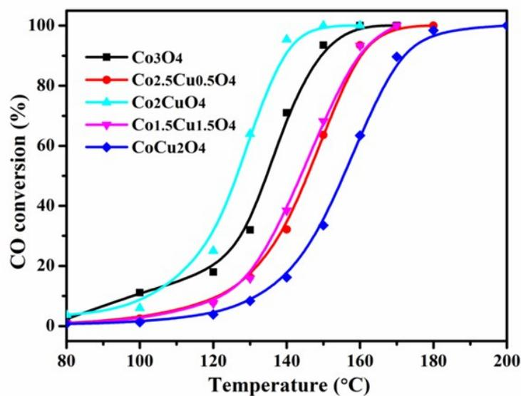
**Fig. S8** the catalytic activities of the as-prepared integrated  $\text{Co}_{3-x}\text{Cu}_x\text{O}_4$  NAs catalysts for CO oxidation.
