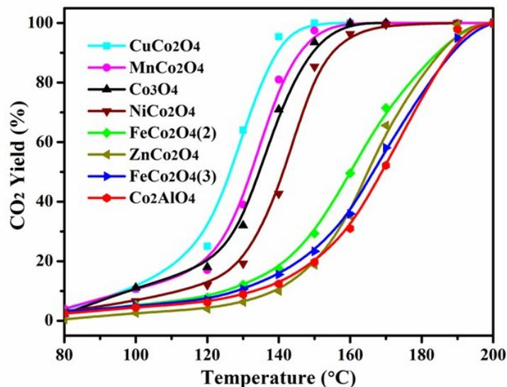
**Fig. S2** the  $\text{CO}_2$  yield curves over all the  $M\text{Co}_2\text{O}_4$  NAs samples as a function of temperature.
