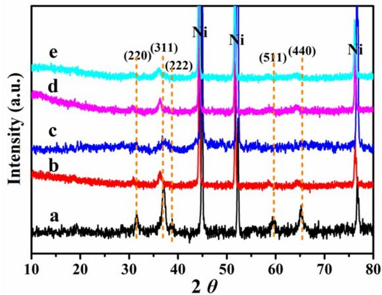
Fig. S3 the XRD patterns of  $\text{Co}_{3-x}\text{Mn}_x\text{O}_4$  NAs: inserted a-e correspond to  $\text{Co}_3\text{O}_4$ ,  $\text{Co}_{2.5}\text{Mn}_{0.5}\text{O}_4$ ,  $\text{MnCo}_2\text{O}_4$ ,  $\text{Co}_{1.5}\text{Mn}_{1.5}\text{O}_4$ , and  $\text{Mn}_2\text{CoO}_4$ , respectively.
