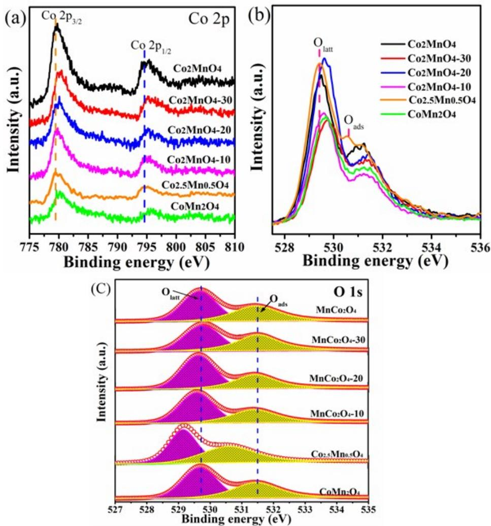
**Fig. S6** (a) Co 2p XPS spectra, (b) O 1s XPS spectra and (c) Core level O 1s XPS spectra of the MnCo<sub>2</sub>O<sub>4</sub>, MnCo<sub>2</sub>O<sub>4</sub>-30, MnCo<sub>2</sub>O<sub>4</sub>-20, MnCo<sub>2</sub>O<sub>4</sub>-10 and CoMn<sub>2</sub>O<sub>4</sub> NAs samples.
