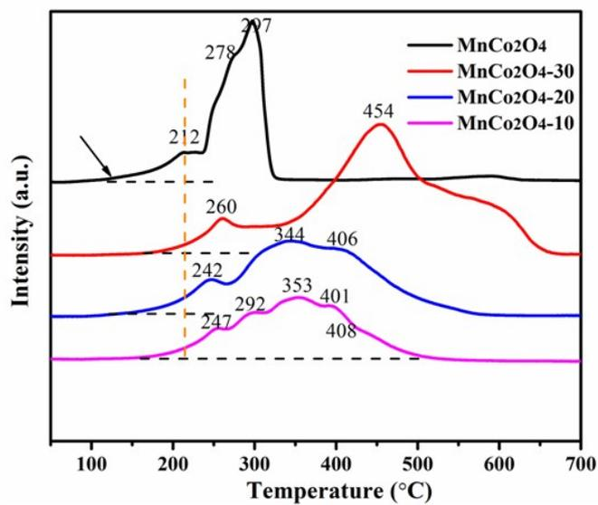
Fig. S4  $\text{H}_2$ -TPR profiles of the  $\text{MnCo}_2\text{O}_4$ -X NAs samples.
