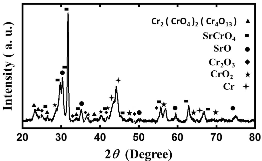
Figure S2 . pXRD profile after  $\text{H}_2$ -temperature programmed reduction of  $\text{SrCrO}_4$ .
