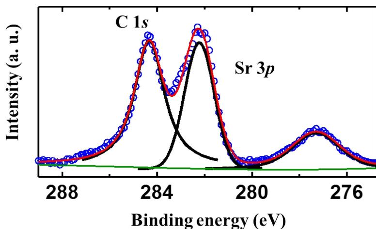
**Figure S3.** X-ray photoelectron spectral profiles of SrCrO<sub>4</sub> in the region of C 1s and Sr 3p.
