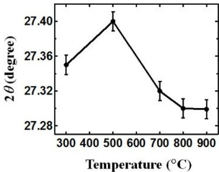
Figure S1. The dependence of  $2\theta$  of  $\text{SrCrO}_4$  as a function of temperature.
