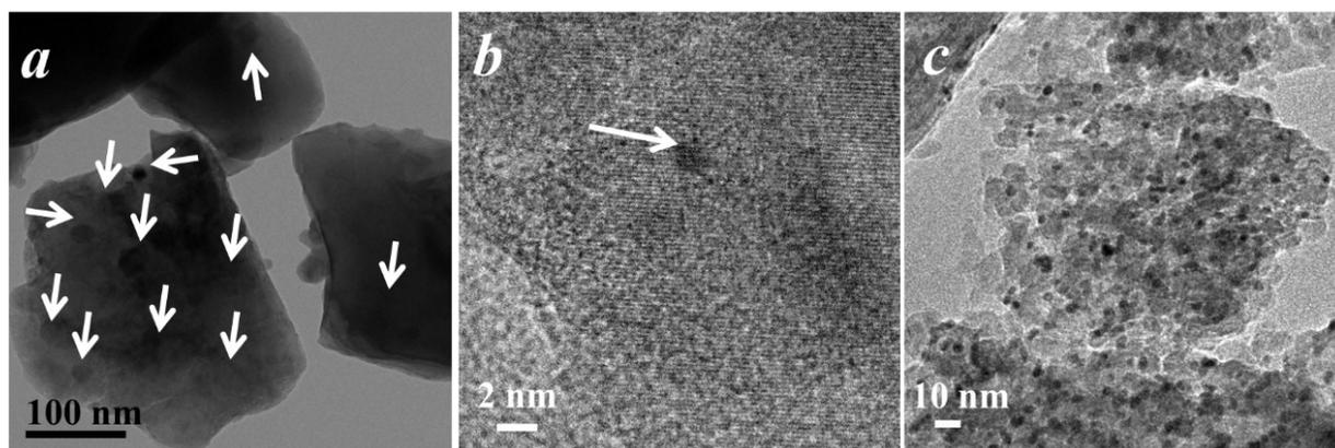
**Figure S6.** TEM (a) and HR-TEM image (b) of Pt/SrCrO<sub>4</sub> (Pt loading = 5 wt.%), TEM image of the commercial Pt/Al<sub>2</sub>O<sub>3</sub> (Pt loading = 5 wt.%).
