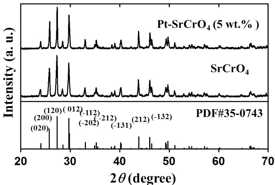
**Figure S5.** pXRD profile of Pt/SrCrO<sub>4</sub> (Pt loading = 5 wt.%). pXRD profile of SrCrO<sub>4</sub> is shown for reference purpose.
