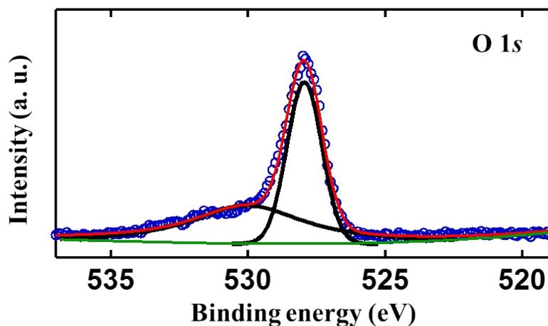
**Figure S4.** X-ray photoelectron spectral profiles of SrCrO<sub>4</sub> in the region of O 1s.
