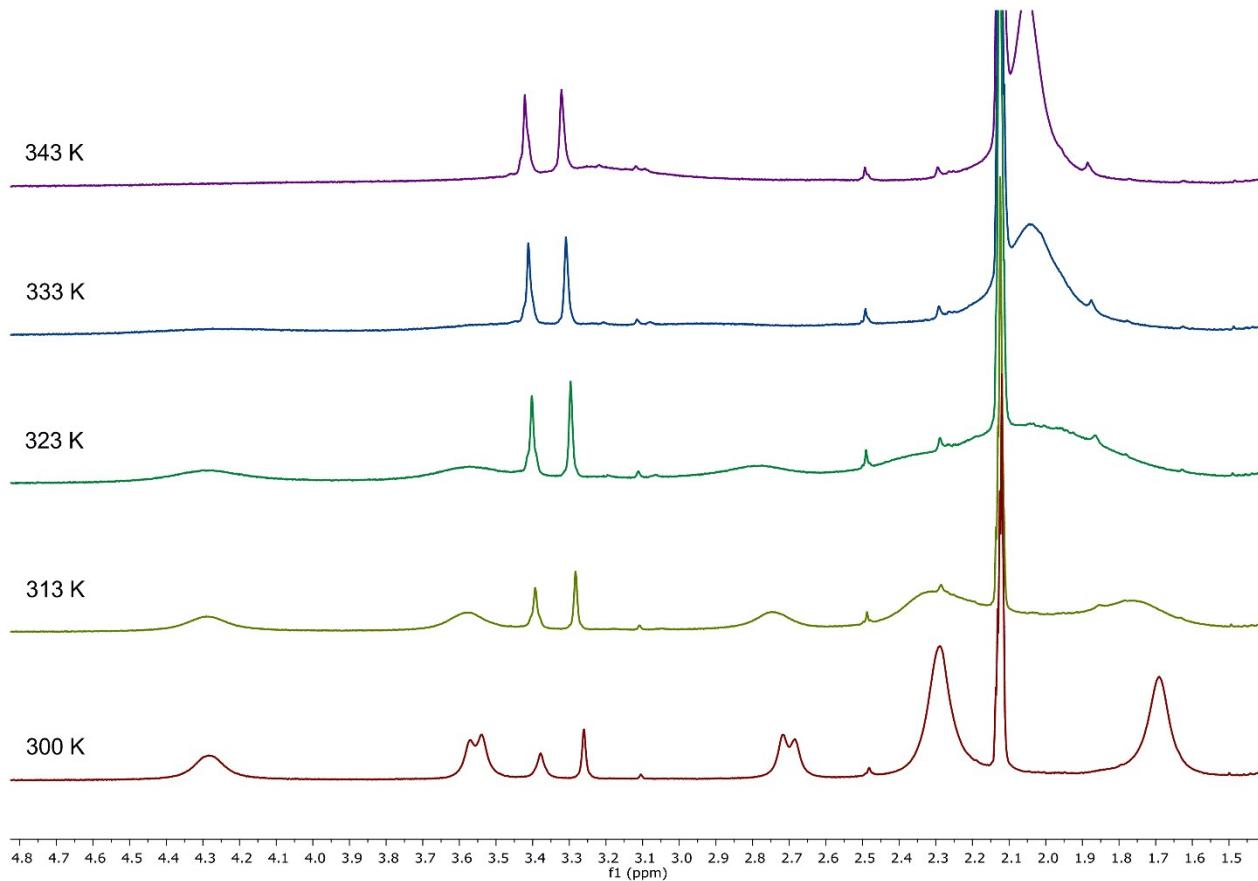
$^1\text{H}$  VT NMR (toluene- $d_8$ , 400.1 MHz) for  $[\{\text{L}^{\text{Se},(\text{CF}_3)_2}\}\text{CdN}(\text{SiMe}_3)_2]$  (**4**).
