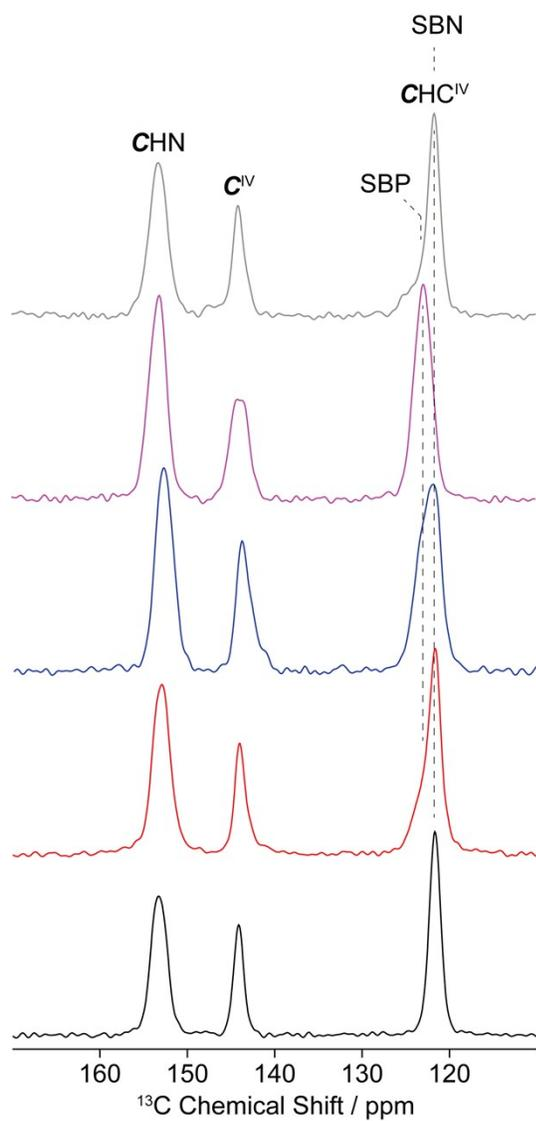
**Figure S5.**  $^{13}\text{C}$  CP MAS NMR of the SBN/SBP anion exchange of SBN pre-exchange (black), after 10 min (red), 25 min (blue), complete exchange to SBP (purple) and regeneration back to SBN (grey) obtained at 9.4 T. Spectral assignments are given in the figure.
