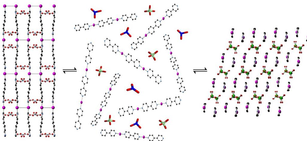
**Figure S2.** Schematic of perchlorate capture by SBN *via* a solvent-mediated anion exchange to form SBP.
