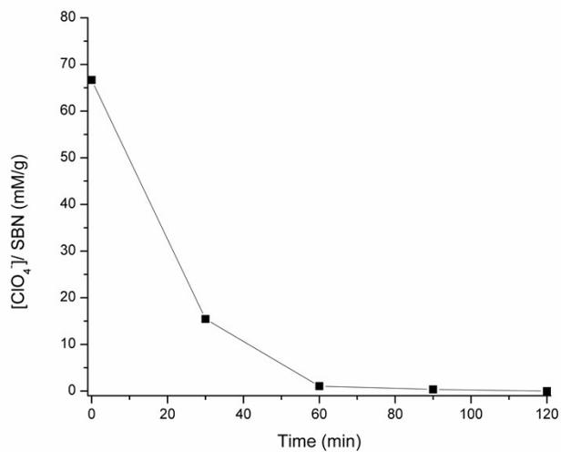
**Figure S3.** Perchlorate uptake per gram of SBN material versus time.
