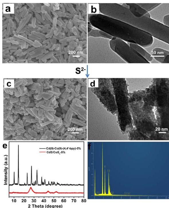
**Fig. S8** (a) SEM image and (b) TEM image of the Cd(II)-Co(II)-(4,4'-bpy)-5% coordination polymer. (c) SEM image, (d) TEM image, (e) XRD pattern and (f) EDX spectrum of the CdS/CoS<sub>x</sub>-5% nano hybrids.
