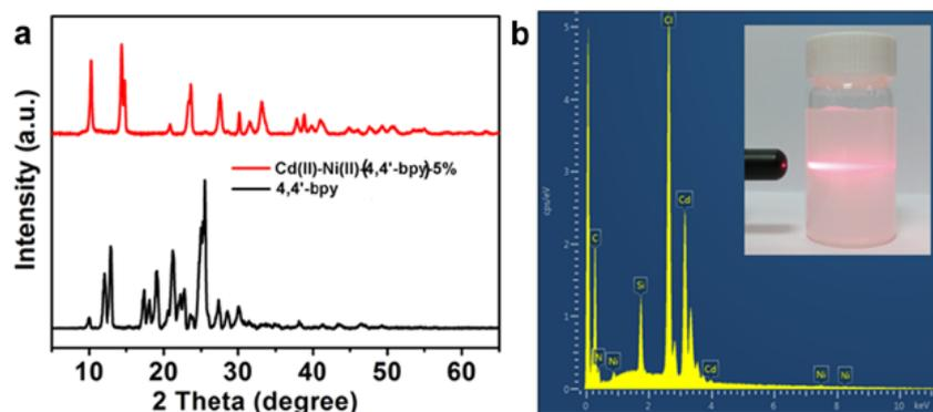
**Fig. S1** (a) XRD patterns of 4,4'-bpy and the Cd(II)-Ni(II)-(4,4'-bpy)-5% coordination polymer. (b) EDX spectrum of the Cd(II)-Ni(II)-(4,4'-bpy)-5% coordination polymer. The inset of (b) is the photograph of the dispersion containing Cd(II)-Ni(II)-(4,4'-bpy)-5% coordination polymer. The light beam is incident from the side to demonstrate the Tyndall effect.
