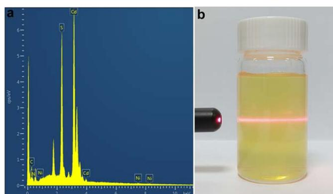
**Fig. S2** (a) EDX spectrum of the CdS/NiS<sub>x</sub>-5% nanohybrid. (b) The photograph of the dispersion containing CdS/NiS<sub>x</sub>-5% nanohybrid. The light beam is incident from the side to demonstrate the Tyndall effect.
