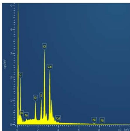
**Fig. S4** EDX spectrum of the intermediate collected after 3 min reaction with S<sup>2-</sup> anions.
