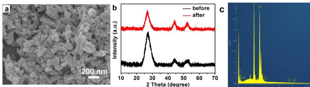
**Fig. S11** (a) SEM image, (b) XRD pattern and (c) EDX spectrum of the CdS/NiS<sub>x</sub>-5% nanohybrid photocatalyst after photocatalytic reaction test.
