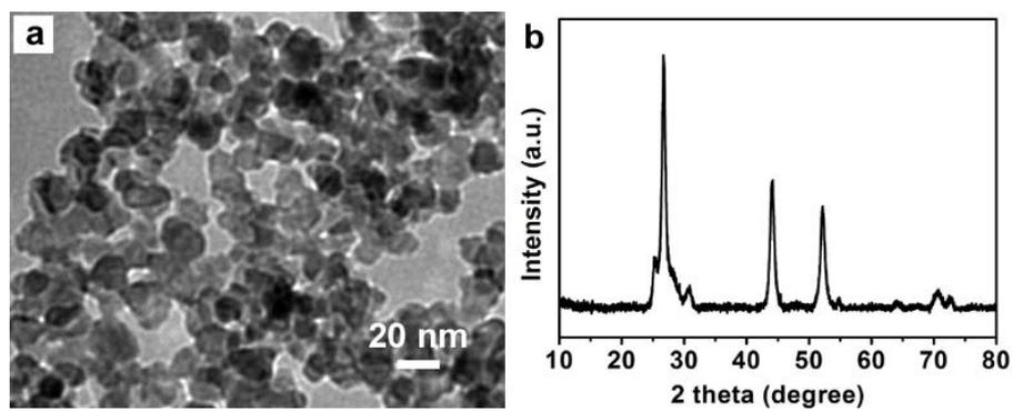
**Fig. S5** (a) TEM image and (b) XRD pattern of CdS/NiS<sub>x</sub>-5% sample obtained at 160 °C under hydrothermal condition.
