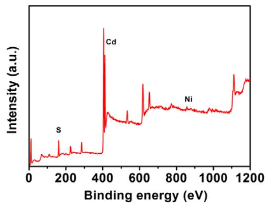
**Fig. S3** XPS survey spectrum of the CdS/NiS<sub>x</sub>-5% nano hybrid.
