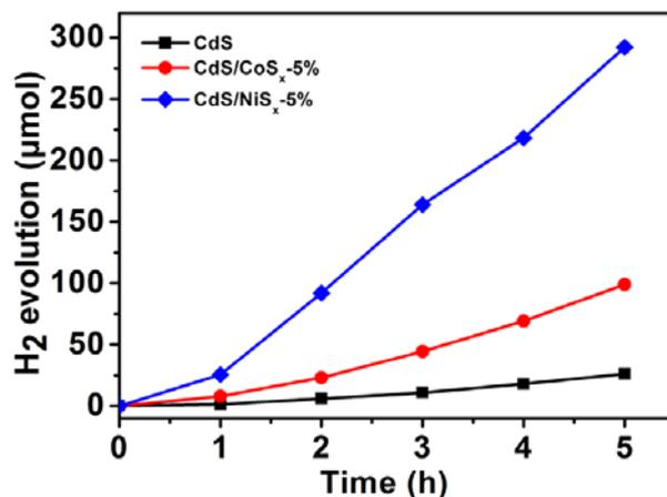
**Fig. S10** Time course of photocatalytic H<sub>2</sub> evolution over various photocatalytic reaction conditions. It was found that the photocatalytic activity of CdS/CoS<sub>x</sub>-5% is higher than that of CdS while lower than that of CdS/NiS<sub>x</sub>-5% photocatalyst.
