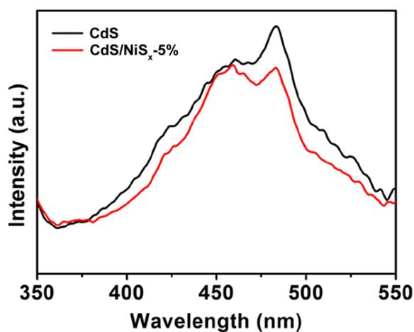
**Fig. S12** Photoluminescence spectra of the CdS and CdS/NiS<sub>x</sub>-5% nanohybrid (excitation wavelength: 330 nm).
