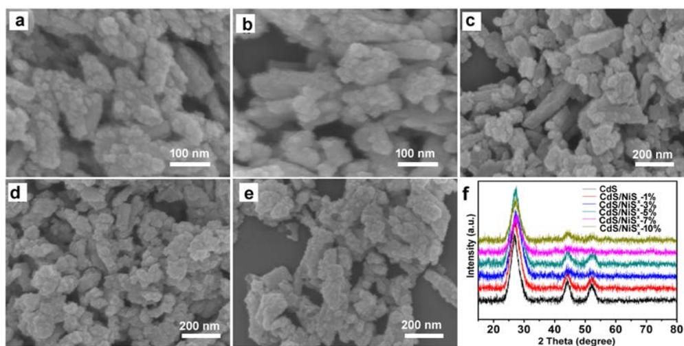
**Fig. S7** (a-e) CdS and CdS/NiS<sub>x</sub> nanohybrids with different Cd/Ni mole ratios: (a) CdS (b) CdS/NiS<sub>x</sub>-1%, (c) CdS/NiS<sub>x</sub>-3%, (d) CdS/NiS<sub>x</sub>-7%, (e) CdS/NiS<sub>x</sub>-10%. (f) XRD patterns of various CdS/NiS<sub>x</sub> nanohybrids.
