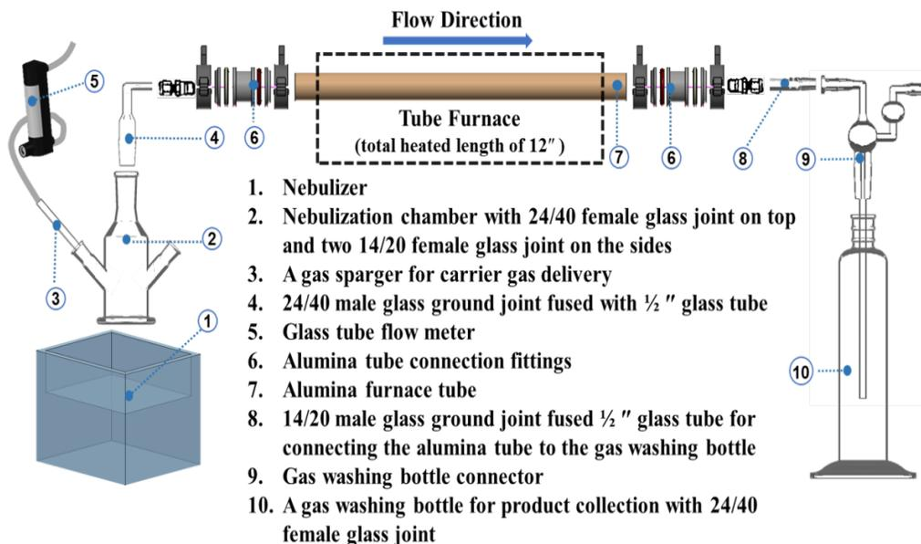
**Figure S1:** Schematic of the ultrasonic spray synthesis apparatus.
