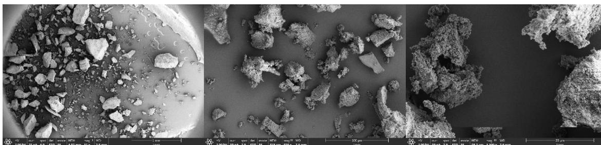
Fig. S12. SEM images for CPO-27-Mg1 afforded from MeOH/NaOH. From left to right, 1 mm; 100 μm; 10 μm
