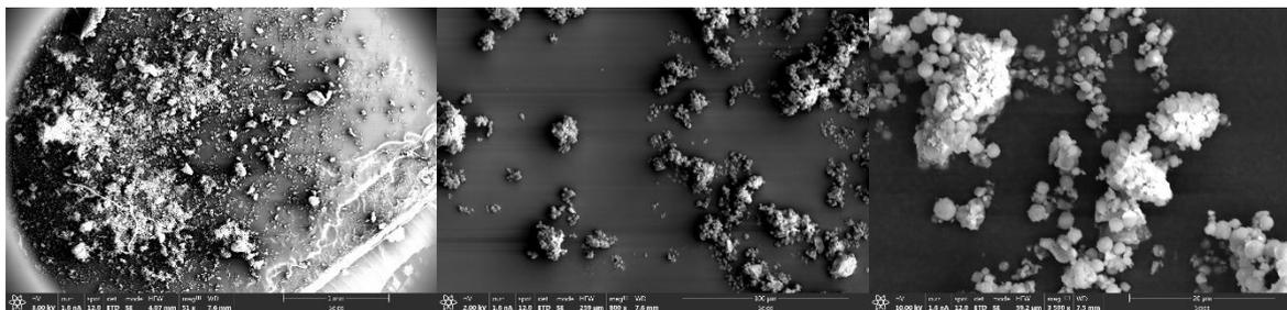
Fig. S16. SEM images for CPO-27-Zn4 afforded from THF without base. From left to right, 1 mm; 100 μm; 20 μm
