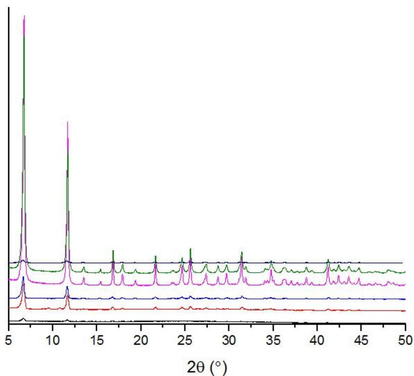
Fig. S5. Powder X-ray diffraction patterns for *CPO-27-Zn1* in MeOH/NaOH taken half-way through the synthesis (3h). -78 °C – black; -40 °C – red; -20 °C – blue; 0 °C – pink; ambient – green; 78 °C – navy.
