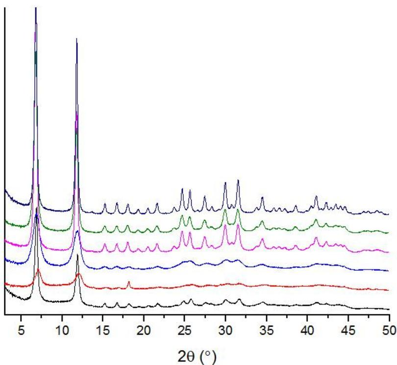
Fig. S2. Powder X-ray diffraction patterns for fully formed CPO-27-Mg1. -78 °C – black; -40 °C – red; -20 °C – blue; 0 °C – pink; ambient – green; 78 °C – navy.
