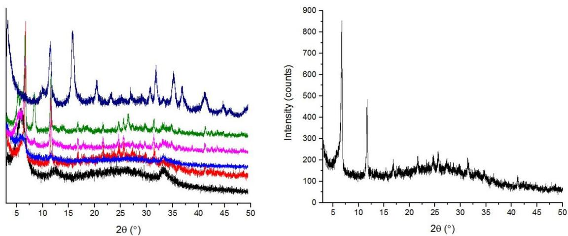
Fig. S8. Left - Powder X-ray diffraction patterns for *CPO-27-Zn5* in THF/NaOH taken half-way through the synthesis (3h). -78 °C – navy; -40 °C – green; -20 °C – pink; 0 °C – blue; ambient – red; 78 °C – black. Right – Powder X-ray diffraction pattern for *CPO-27-Zn5* in THF/NaOH at -40 °C.
