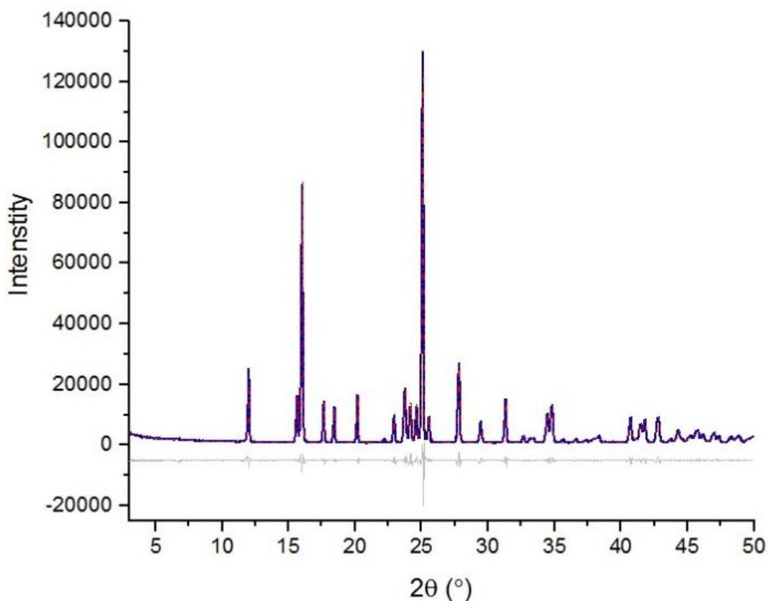
Fig. S11. Topas Pawley refinement for  $[\text{Zn}(\text{H}_2\text{dhtp})(\text{H}_2\text{O})_2]$  afforded from a CPO-27–Zn3 synthesis attempt in MeOH. Experimental in blue, calculated model in red and the calculated difference plot in grey.<sup>22</sup>
