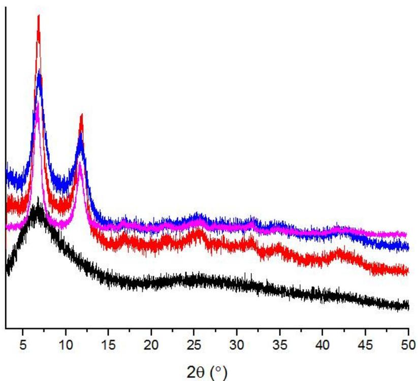
Fig. S3. Powder X-ray diffraction patterns for CPO-27-Ni1 taken half-way through the synthesis (3h). -20 °C – black; 0 °C – red; ambient – blue; 78 °C – pink.
