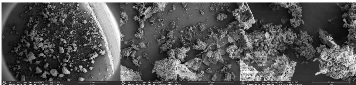
Fig. S17. SEM images for CPO-27-Zn5 afforded from THF/NaOH. From left to right, 1 mm; 100 μm; 10 μm
