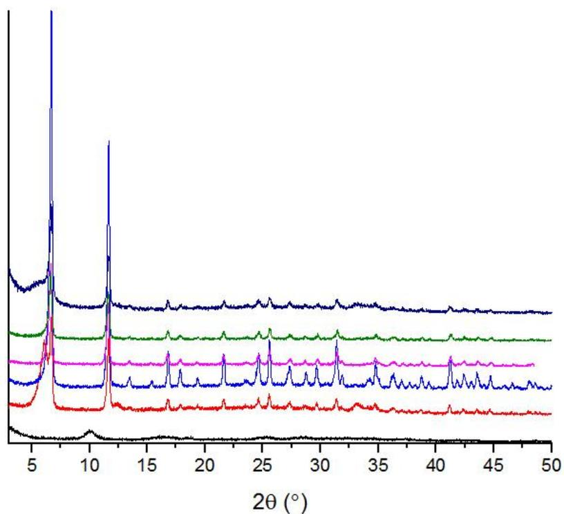
Fig. S9. Powder X-ray diffraction patterns for CPO-27-Zn6 in THF/TEA taken half-way through the synthesis (3h). -78 °C – navy; -40 °C – green; -20 °C – pink; 0 °C – blue; ambient – red; 78 °C – black.
