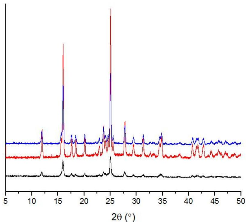
Fig. S7. Powder X-ray diffraction patterns for *CPO-27-Zn3* in MeOH without base taken half-way through the synthesis (3h). 0 °C – black; ambient – red; 78 °C – blue.
