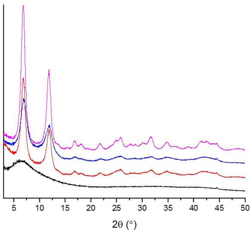
Fig. S4. Powder X-ray diffraction patterns for fully formed CPO-27-Ni1. -20 °C – black; 0 °C – red; ambient – blue; 78 °C – pink.
