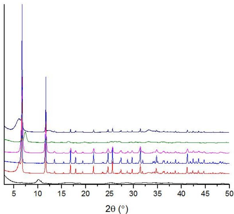
Fig. S10. Powder X-ray diffraction patterns for fully formed CPO-27-Zn6 in THF/TEA. -78 °C – navy; -40 °C – green; -20 °C – pink; 0 °C – blue; ambient – red; 78 °C – black.
