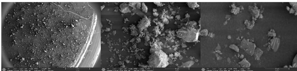
Fig. S13. SEM images for CPO-27-Ni1 afforded from MeOH/NaOH. From left to right, 1 mm; 50 μm; 10 μm
