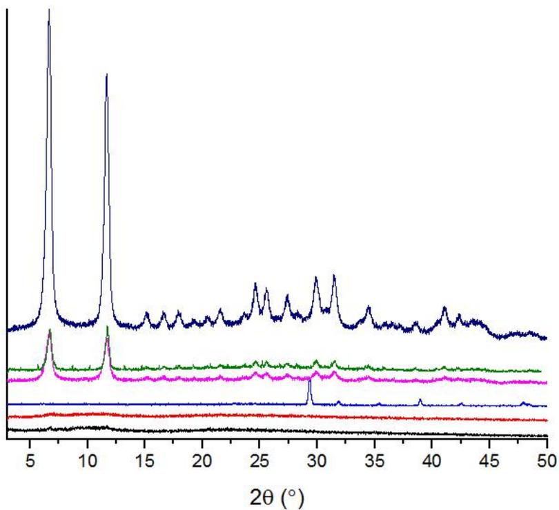
Fig. S1. Powder X-ray diffraction patterns for CPO-27-Mg1 taken half-way through the synthesis (3h). -78 °C – black; -20 °C – red; -40 °C – blue; ambient – pink; 78 °C – green; 0 °C – navy. All diffraction run for 3 hours with the exception of 0 °C which was run for 12 hours.
