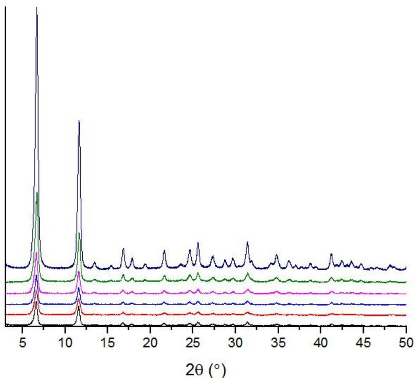
Fig. S6. Powder X-ray diffraction patterns for *CPO-27-Zn2* in MeOH/TEA taken half-way through the synthesis (3h). -78 °C – navy; -40 °C – green; -20 °C – pink; 0 °C – blue; ambient – red; 78 °C – black
