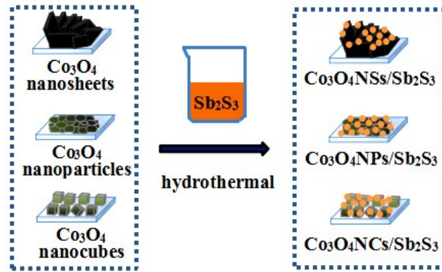
Fig.S5 Brief schematic diagram of synthetic route of \text{Co}_3\text{O}_4/\text{Sb}_2\text{S}_3 heterojunctions
