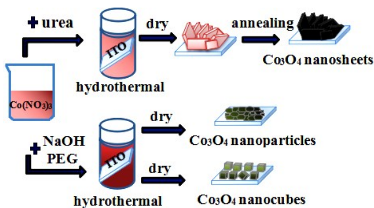
Fig.S1 Brief schematic diagram of synthetic route of \text{Co}_3\text{O}_4 nanostructures
