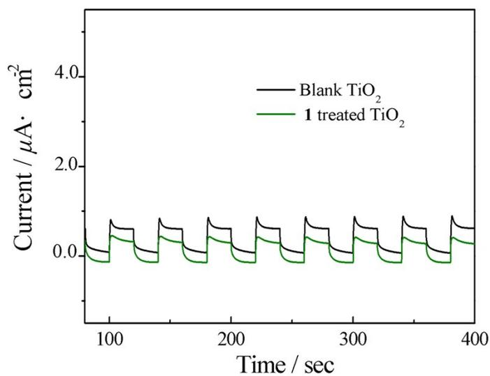
Fig. S6. Photocurrent densities of 1 treated electrode and the blank porous  $\text{TiO}_2$  electrode.
