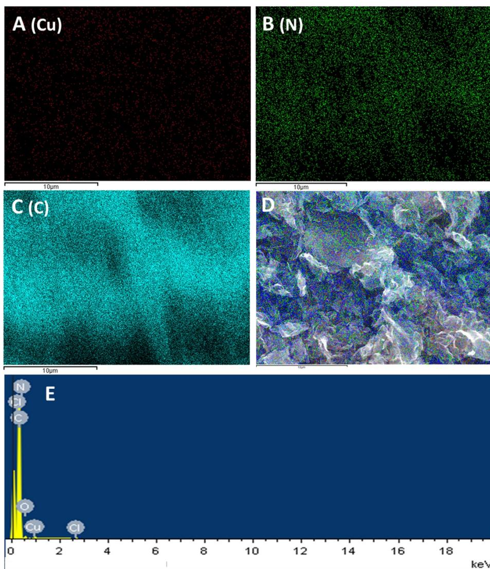
**Figure S6** The SEM-EDS mapping images for Cu (A), N (B), C (C) and total element mapping image for Cu, N, C, O and Cl (D), and the SEM EDS spectrum (E) for the prepared Cu-N-GR-800.
