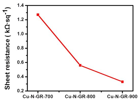
**Figure S9** Sheet resistance of the prepared Cu-N-GR nanosheets at different temperatures.
