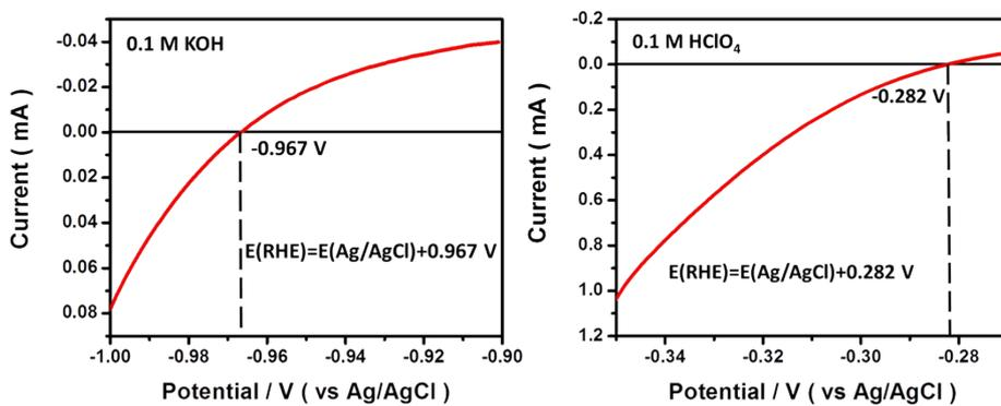
**Figure S8** Calibration to reversible hydrogen electrode (RHE).
