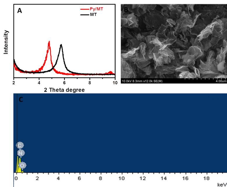
**Figure S1** (A) XRD patterns of MT (black) and Py/MT intercalation compounds (red). (B) SEM image of the N-GR-800. (C) The SEM-EDS spectrum for the prepared N-GR-800.
