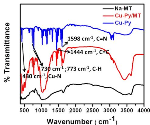
**Figure S3** The FT-IR spectrums of Cu-Py (blue), Cu-Py/MT intercalation compounds (red) and Na-MT (black).
