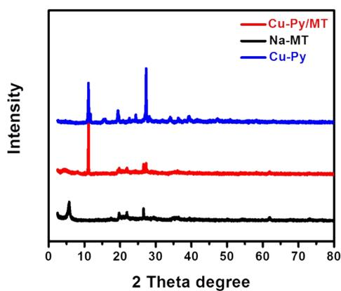
**Figure S2** XRD patterns of Na-MT (black), Cu-Py/MT intercalation compounds (red) and Cu-Py (blue).
