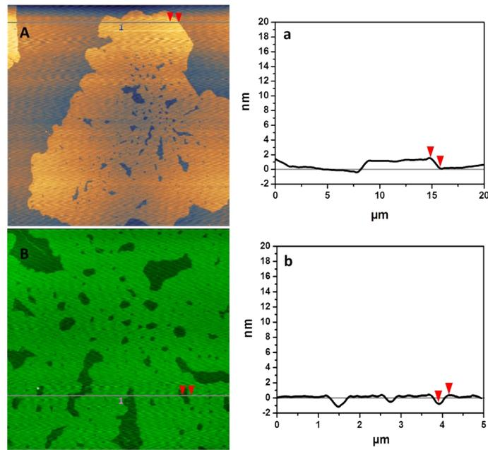
**Figure S5** The typical tapping mode AFM images of the prepared Cu-N-GR-800 deposited on a mica substrate in different regions (A and B) and the corresponding height profiles shown in (a) and (b).
