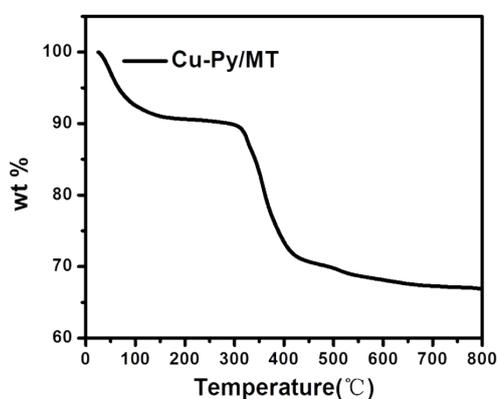
**Figure S4** TGA plot of Cu-Py/MT in air atmosphere.
