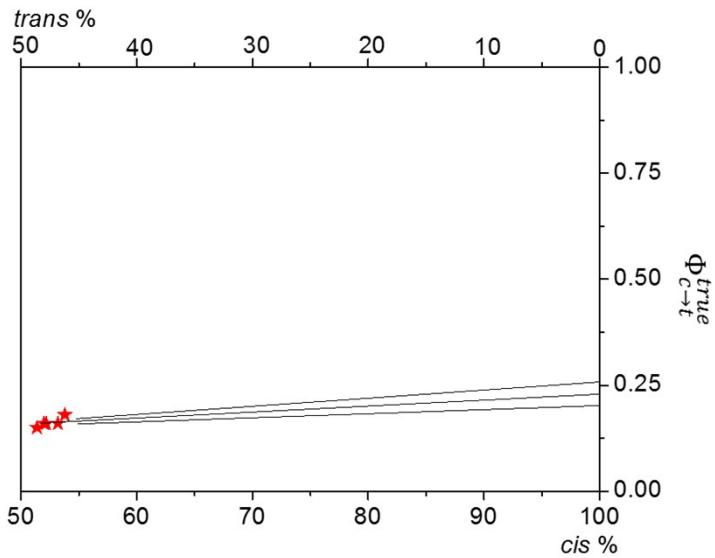
**Figure S3.** Extrapolation of the  $\Phi_{c \rightarrow t}^{true}$  magnitude for a pure (100%) cis-solution.
